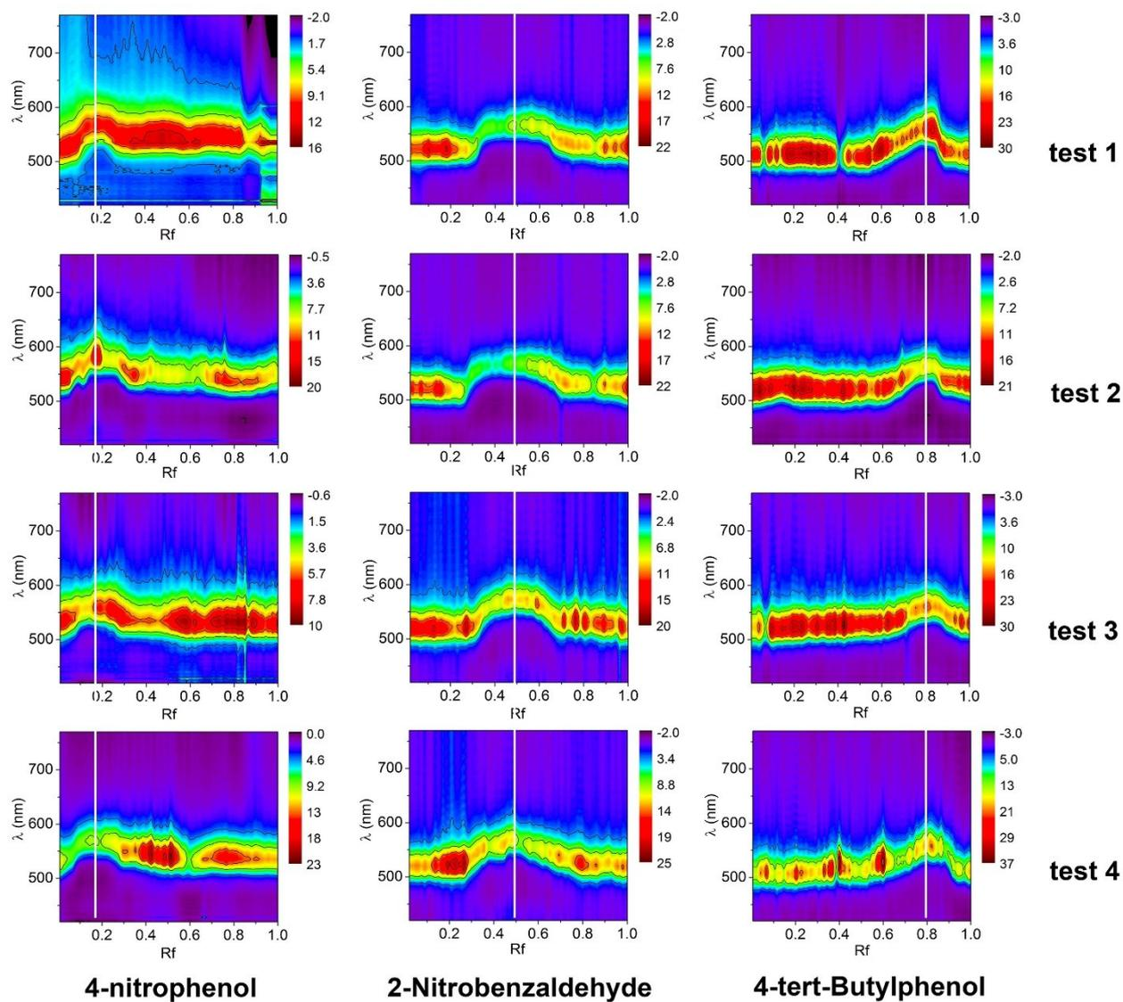
**Figure S5. Differential migration of 4-NP, 2-NBA and 4-t-BP.** Spatially resolved reflection spectra for the differential migration of 4-nitrophenol, 2-nitrobenzaldehyde and 4-tert-butylphenol on photonic crystal TLC plate in 4 repeated tests.
