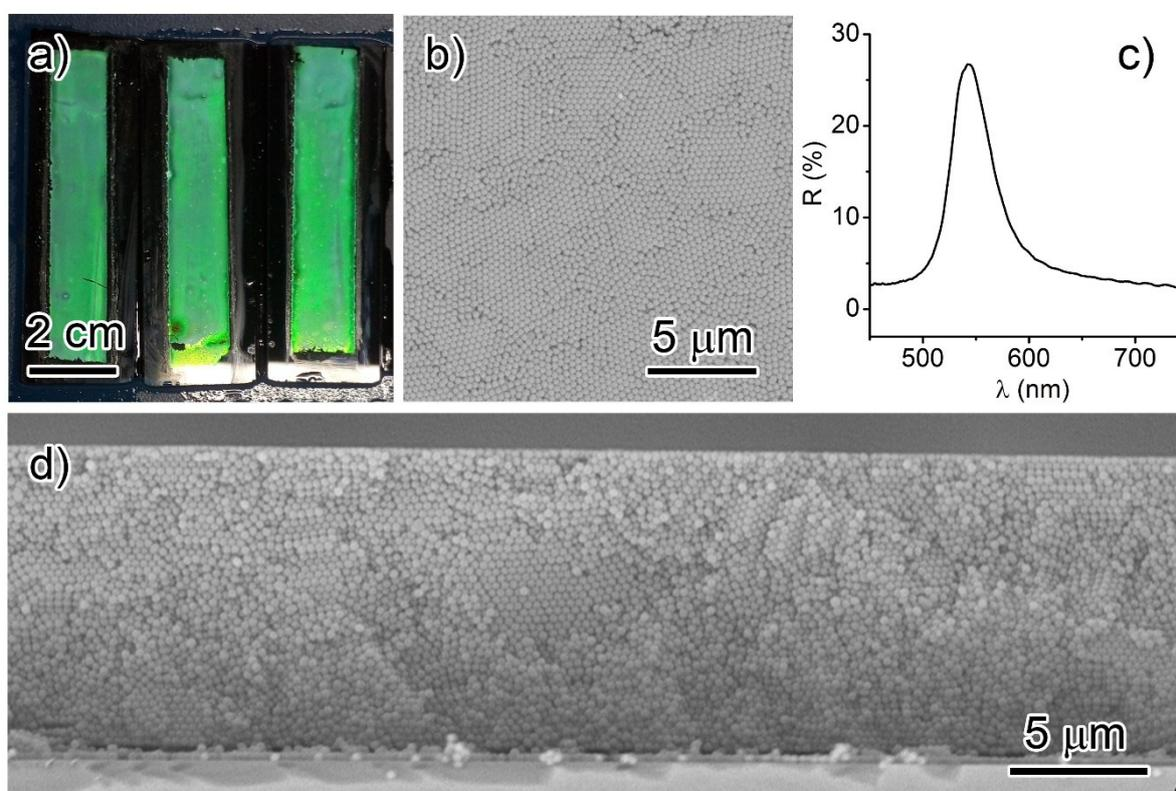
**Figure S1. Ordered structure and optical signal of photonic crystal film.** A) digital photo, b) top-view and d) cross-section SEM image and c) typical reflection spectrum of a green photonic crystal thin film composed of mesoporous SiO<sub>2</sub> particles. SEM image shows that the thin film is composed of crystalline and amorphous stacking of m-SiO<sub>2</sub> particles due to the microscopic phase separation in its metastable precursor.
