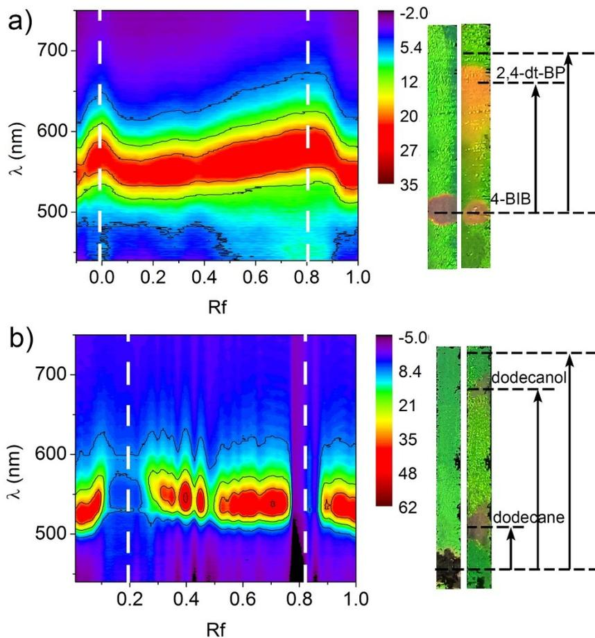
**Figure S10.** Separation of 4-BIB and 2, 4-dt-BP as well as dodecane and dodecanol by reversed phase PC-TLC. Spatial resolved reflection spectra and digital photos for the separation of 4-bromiodobenzene and 2, 4-di-tert-butylphenol as well as dodecane and dodecanol on reversed phase PC TLC plate.
