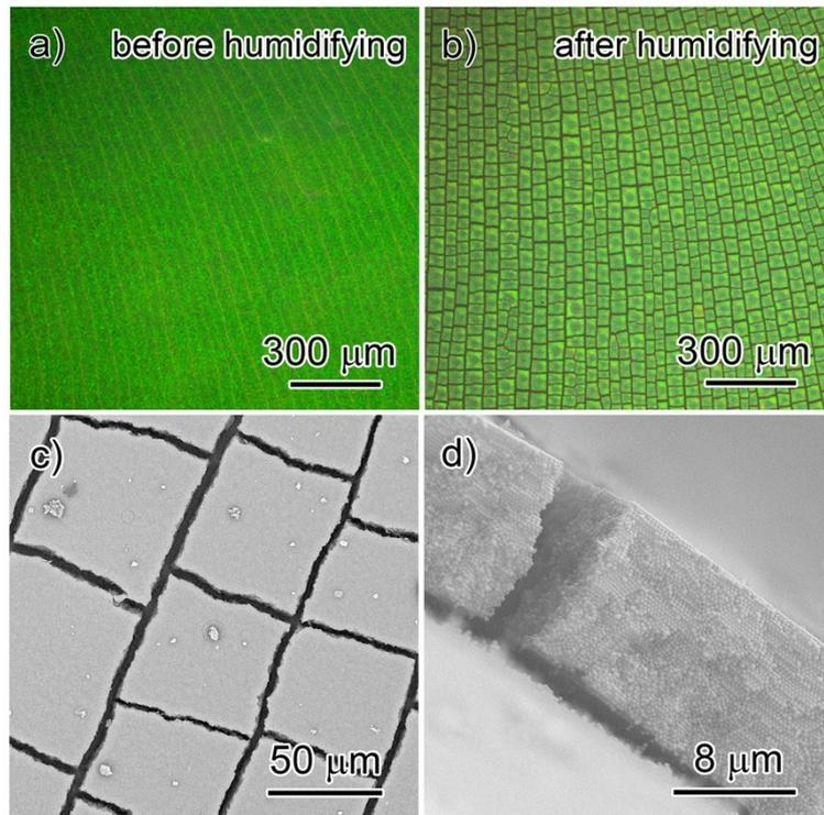
**Figure S3.** Optical microscope image of photonic crystal film a) before and b) after humidifying process in fabrication of TLC plate. c) top-view and d) cross-section SEM image of photonic crystal thin film prepared by mesoporous SiO<sub>2</sub> nanoparticles.
