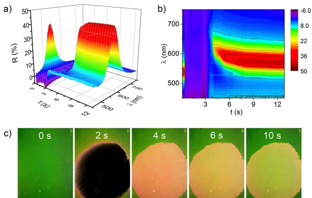
**Figure S4.** a ,b) Time resolved reflection spectra and c) color change of photonic crystal film during the process of sample loading.
