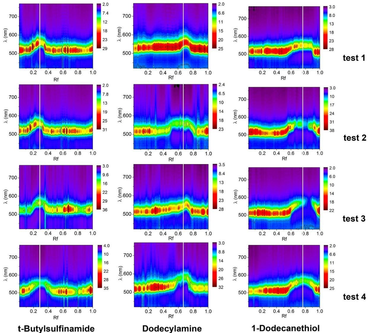
**Figure S6. Differential migration of t-BSA, DA and DT.** Spatial resolved reflection spectra for the differential migration of t-butylsulfonamide, dodecylamide and dodecanethiol on photonic crystal TLC plate in 4 repeated test.
