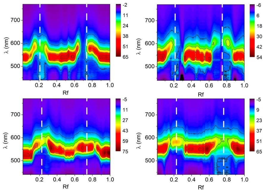
**Figure S7. Separation of 4-NP and 4-t-BP.** Spatial resolved reflection spectra for the separation of 4-nitrophenol and 4-t-butylphenol on photonic crystal TLC plate in 4 repeated test.
