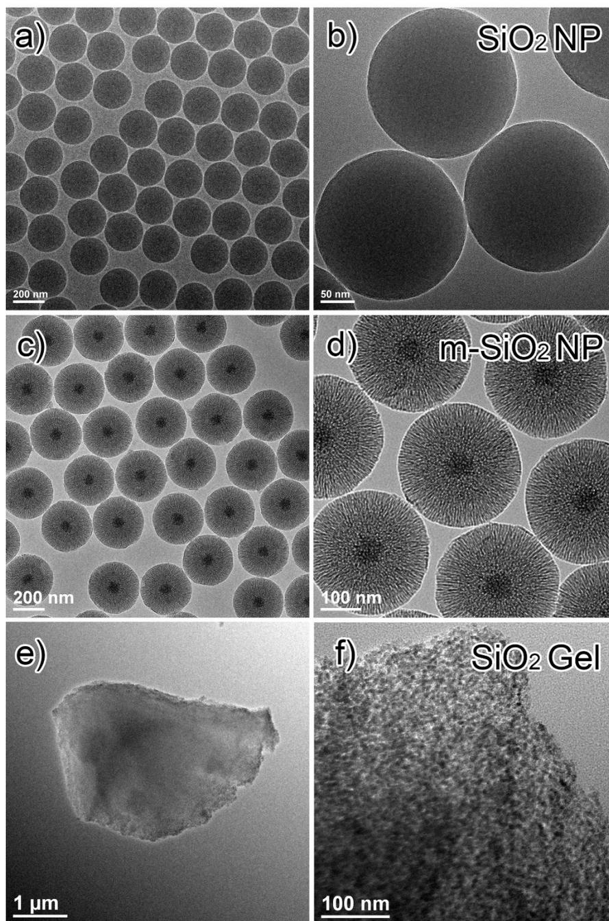
**Figure S2. Three kinds of SiO<sub>2</sub> particles for fabrication of TLC plates.** TEM image of a, b) dense SiO<sub>2</sub> nanoparticle, c, d) mesoporous SiO<sub>2</sub> nanoparticles and e, f) mesoporous SiO<sub>2</sub> gels for the preparation of TLC plates.
