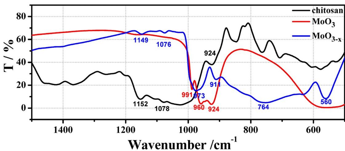
Figure S2 FT-IR spectra of  $\text{MoO}_{3-x}$  quantum dot. Chitosan and  $\text{MoO}_3$  were used as control.
