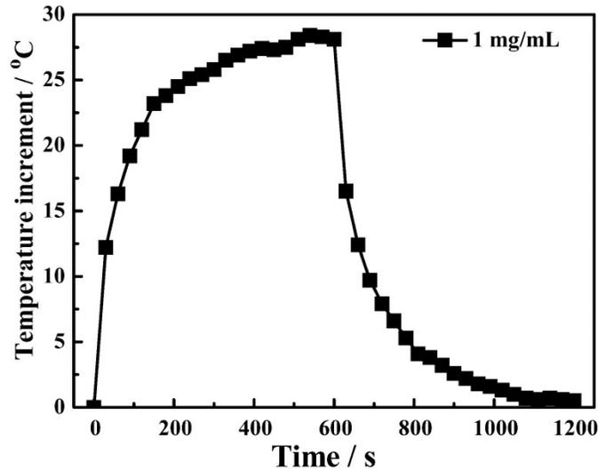
**Figure S4.** Temperature variations of solution containing 1 mg/ml nanocube. The NIR laser irradiation lasted 10 min and then was turned off.
