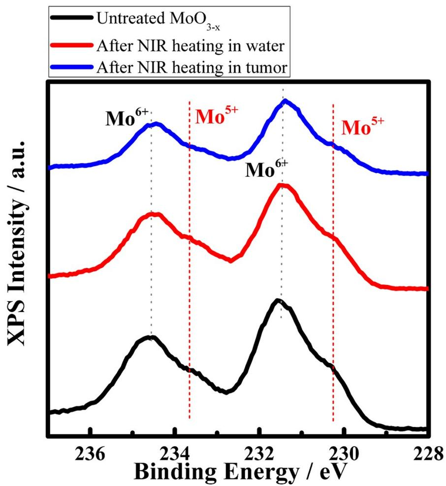
Figure S6 The XPS spectra of MoO<sub>3-x</sub> QDs before and after heating treatment.
