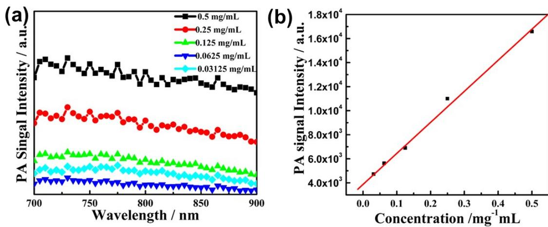
**Figure S7** (a) Photoacoustic signal of MoO<sub>3-x</sub> solutions with different concentrations. (b) Plot of photoacoustic signal at 880 nm versus MoO<sub>3-x</sub> concentrations.
