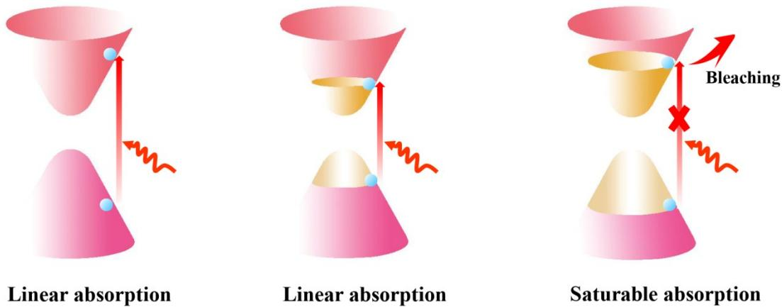
Figure S1. Schematic diagram of optical saturable absorption
