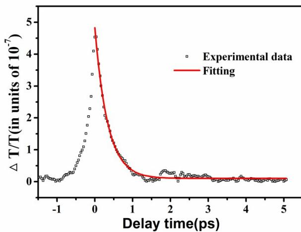
Figure S2. (a) Experimental setup for pump-probe measurement; (b) Pump-probe trace for reference sample 0.3mm ZnS single crystal
