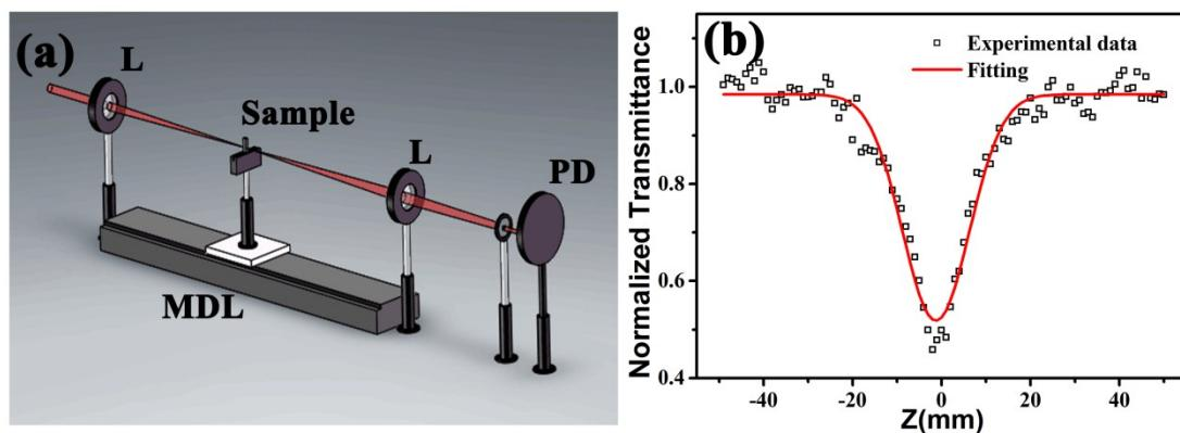
Figure S3. (a) Schematic of the conventional Z-scan measurement: L, lens; PD, photodiode; MDL, mechanical delay line; (b) Z-scan traces for reference sample 0.3mm ZnS single crystal.
