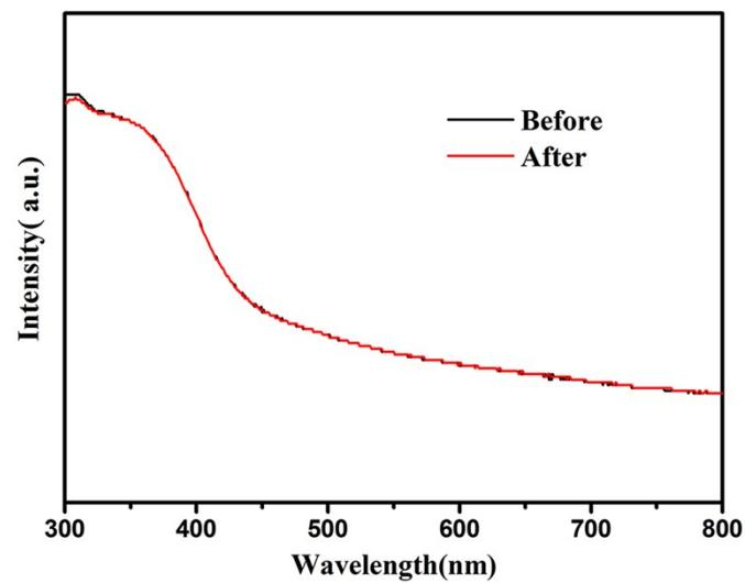
Figure S4. The absorption spectrum of BPQDs before (black line) and after (red line) the experiments
