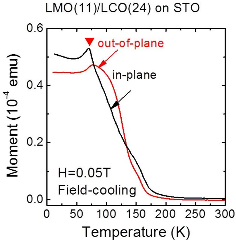
**Figure S4** Temperature dependence of the magnetization of [LMO(11)/LCO(24)]<sub>5</sub>/STO, measured with an in-plane (black curve) or out-of-plane (red curve) field of 0.05 T. Antiferromagnetic phase transition was observed in both cases, as marked by a triangle.
