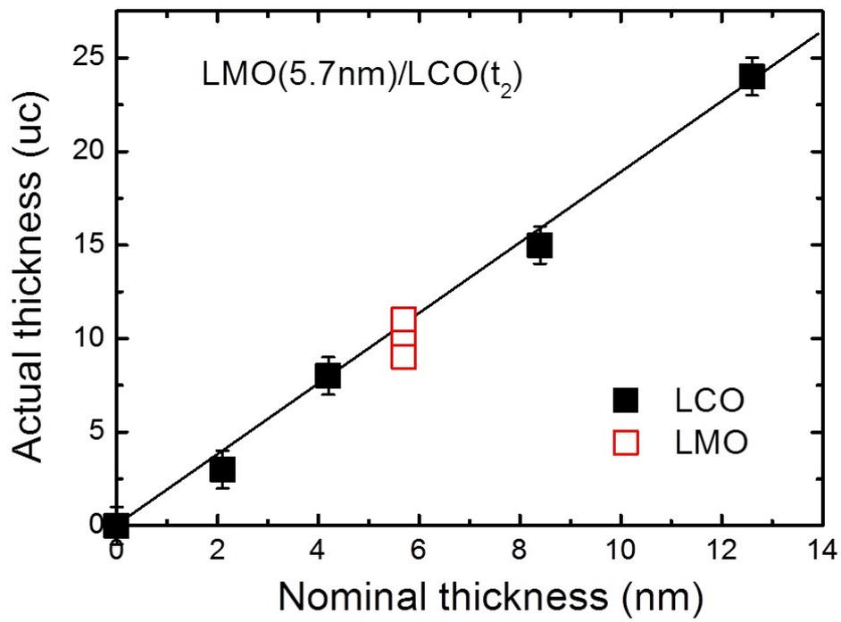
**Figure S2** A conversion relationship between nominal and actual layer thickness obtained by directly counting cell numbers in HAADF images of the SLs on STO. Solid lines are guides for the eye.
