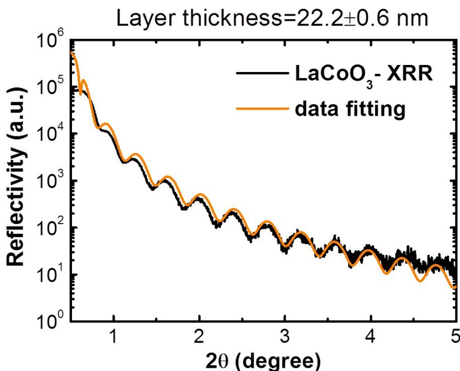
**Figure S1** Small angle x-ray reflectivity of the LCO single layer and the corresponding results of data fitting that gives layer thickness.
