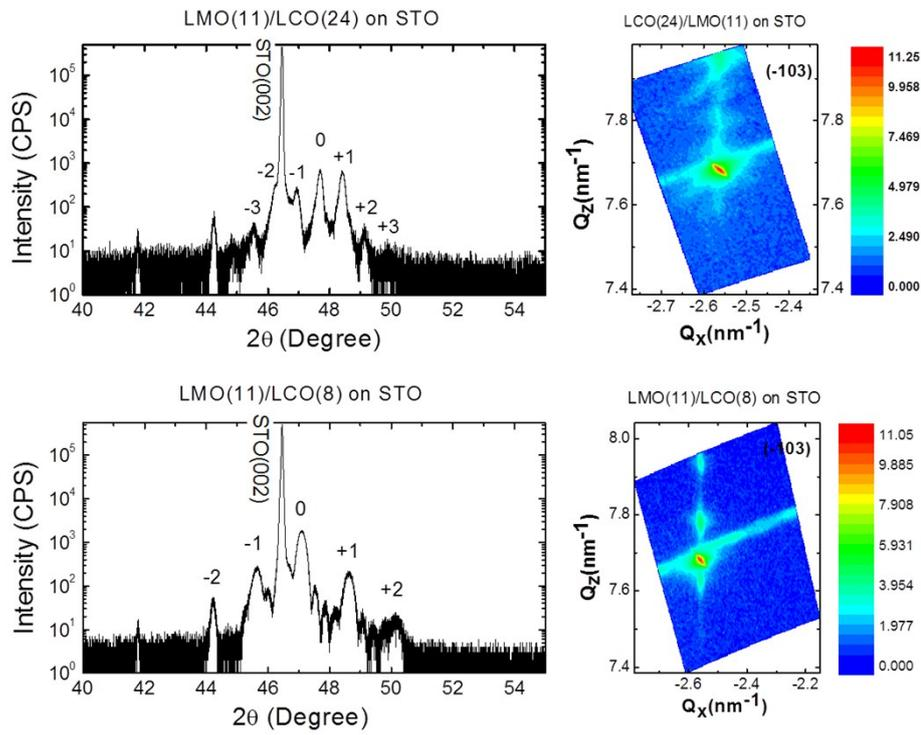
**Figure S3** (Left panel) X-ray diffraction spectra (left panel) for superlattice samples marked in the figure. Satellite peaks corresponding to superlattice structure (marked by numbers) can be clearly seen. (Right panel) The reciprocal space mapping (RSM) for the (-103) reflection.
