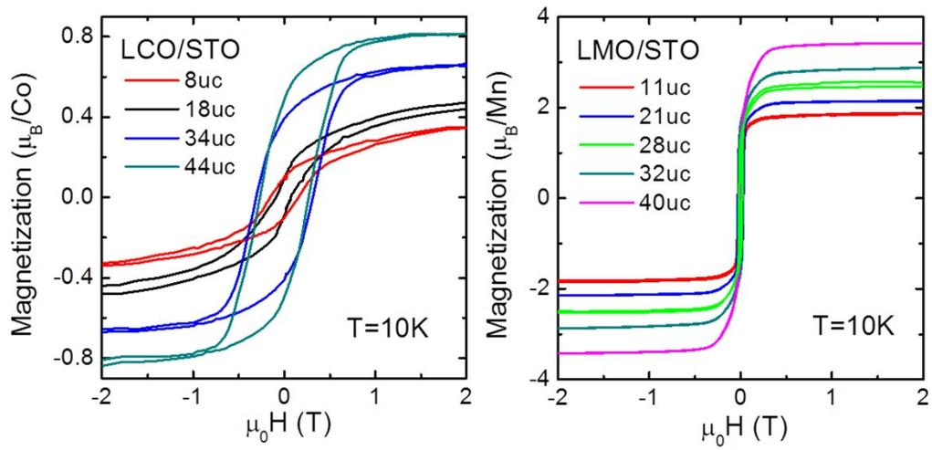
**Figure S7** Magnetizations of the LCO and LMO single layers on STO, measured at 10 K as functions of magnetic field.
