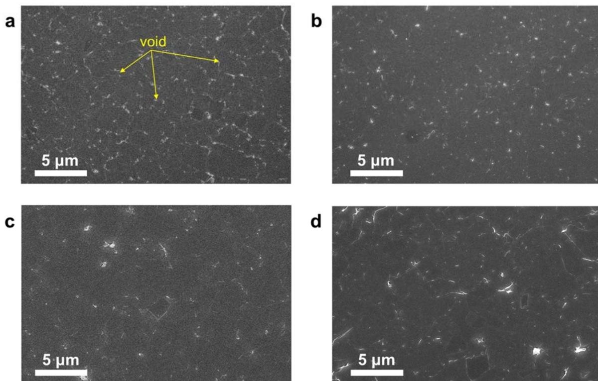
**Fig. S2** SEM image of the surface of Ag-doped RuO<sub>2</sub> NSs films with various deposition condition: (a) Just 2 times LB deposition + Ag doping (Sample 3). (b) 2 times LB deposition + Ag doping (2 times repeated, Sample 4). (c) 4 times LB deposition + Ag doping (Sample 5). (d) 6 times LB deposition + Ag doping (Sample 6)
