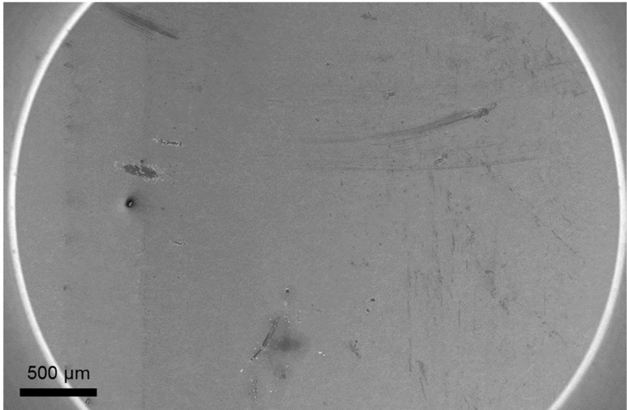
**Fig. S3** Low magnification SEM image of the surface of Ag-doped RuO<sub>2</sub> NSs films after 200,000 cycle 1R folding test. The coating of Ag-doped RuO<sub>2</sub> NSs in folding area was slightly degraded but the connections of Ag-doped RuO<sub>2</sub> NSs were remained.
