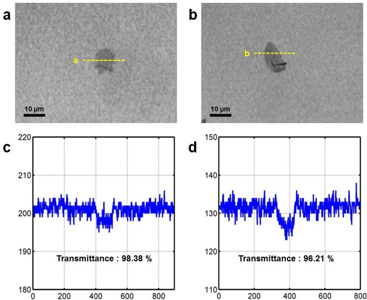
**Fig. S1** Light transmittances of RuO<sub>2</sub> NSs. Optical microscope images of (a) monolayer and (b) two-layer RuO<sub>2</sub> NS (c), (d) Line profiles showing the total transmitted white light intensities along the yellow dotted lines in (a) and (b), respectively. It should be noted that the transmittances of RuO<sub>2</sub> NSs decreased linearly by about 2% with increasing number of layers.
