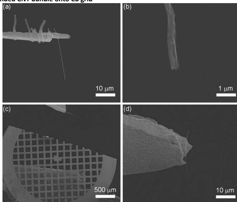
**Fig. S6** The transfer of debonded CNT bundle onto Cu grid. (a) The pulled out CNT bundle. (b) The root of CNT bundle. (c) The sectioned copper grid. (d) The CNT bundle bonded onto sharp corner.
