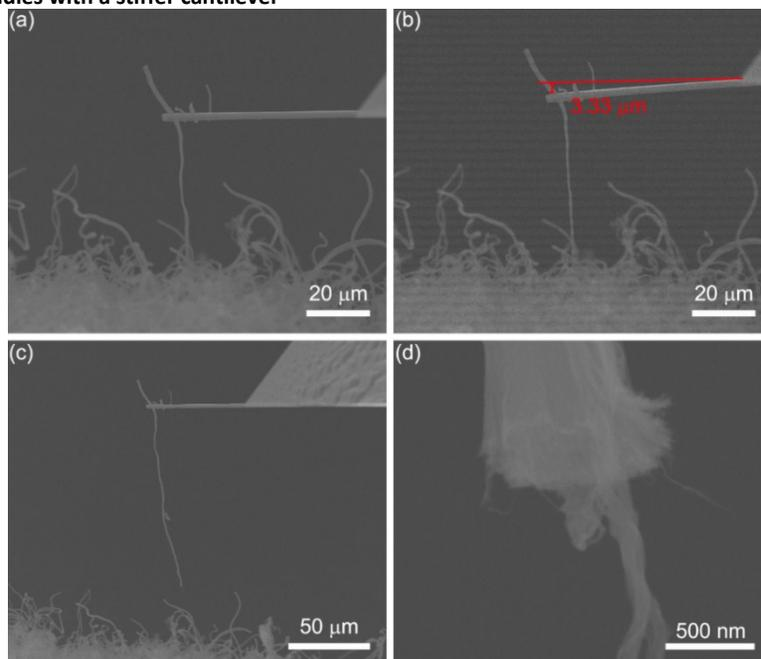
**Fig. S4** SEM images of a CNT bundle debonding from graphene using a cantilever with spring constant of 10.6 N/m. (a) The CNT bundle was engaged with an AFM cantilever. (b) The last moment of CNT bundle debonding from graphene. (c) The pulled-out CNT bundle. (d) High-magnification SEM image of the CNT bundle root.
