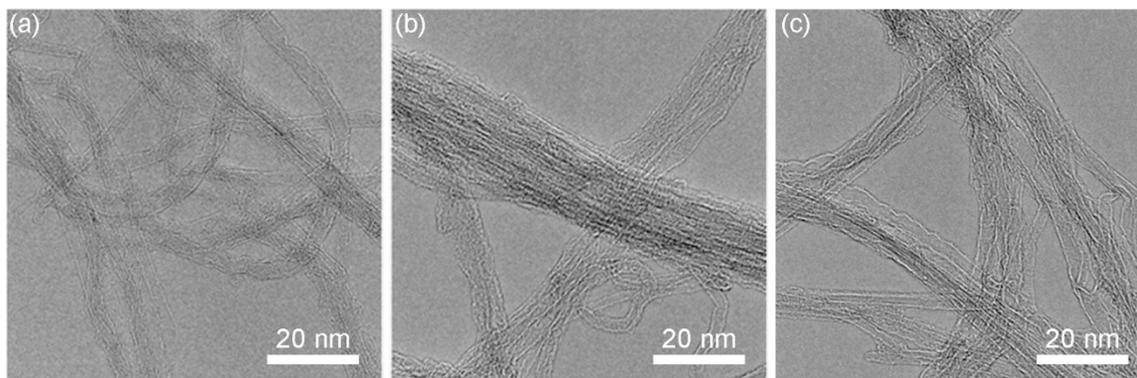
Fig. S1 HRTEM analysis of CNTs from CNTs/graphene nanostructure
