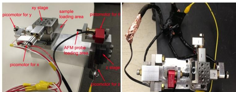
Fig. S2 Configuration of in-house nanomechanical tester
