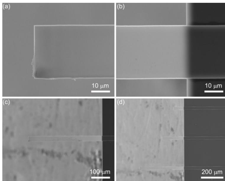
**Fig. S3** SEM images of cantilever after debonding test. (a) Front of cantilever. (b) Bottom of cantilever. (c) Entire cantilever. (d) Three cantilevers sitting on one AFM probe.
