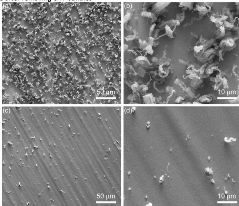
**Fig. S7** SEM images of graphene/Cu after removing CNT forest from 3D CNTs/graphene nanostructures with scotch tape. (a and b) After first peel. (c and d) After second peel.
