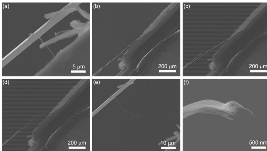
**Fig. S5** Snapshots of a standing-alone CNT bundle debonding from graphene.
