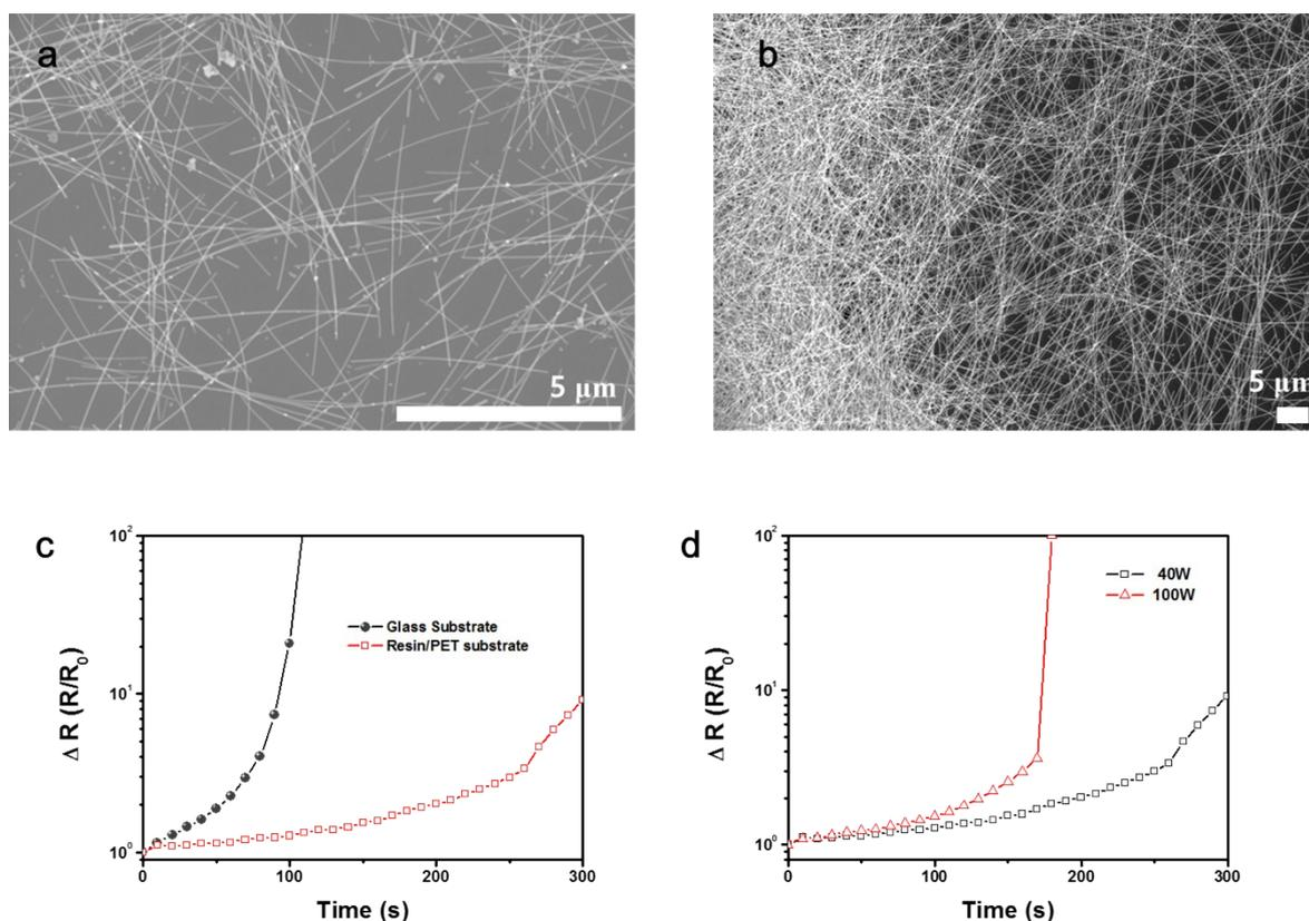
**Figure S1** SEM pictures of synthesized (a) short/thin AgNWs (10 μm / 40 nm) and (b) long/thick AgNWs (100 μm / 100 nm). c) UV resistant test of embedded NWs versus NWs on a bare glass substrate under 40 W plasma treatment. d) UV failure test of embedded NWs under 40 and 100 W plasma power treatment condition.
