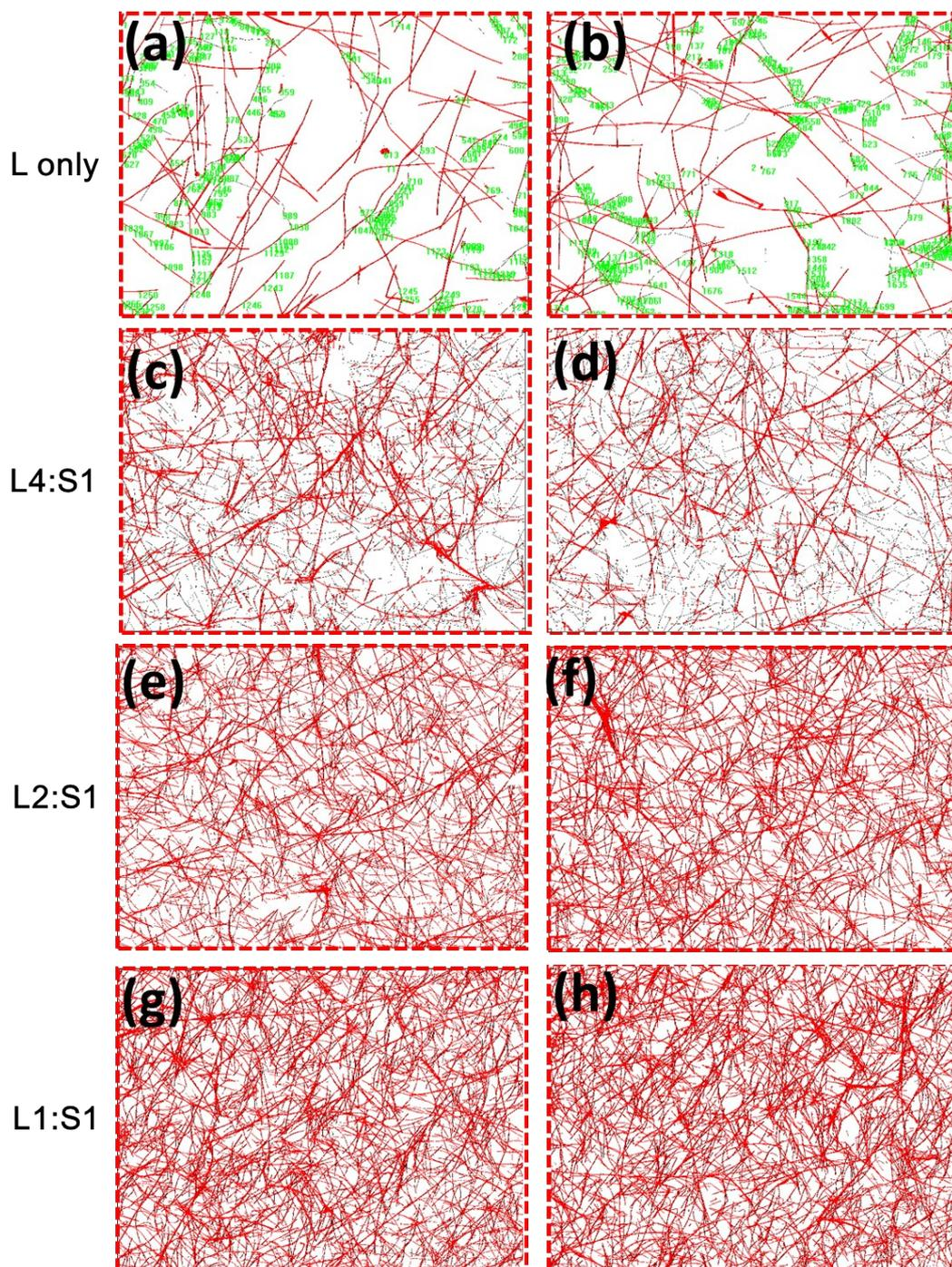
**Figure S6.** Transformed and counted SEM images based on different coating ratio by segmentation in Image Pro.
