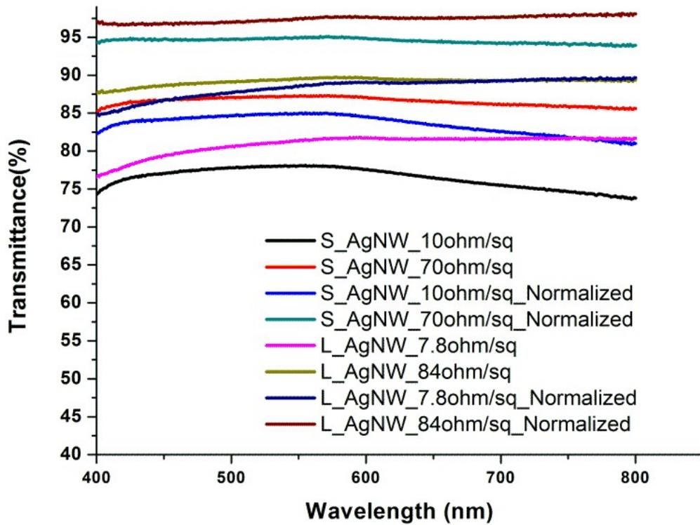
**Figure S2** Spectral transmittance of various transparent electrode based on different AgNWs structures.
