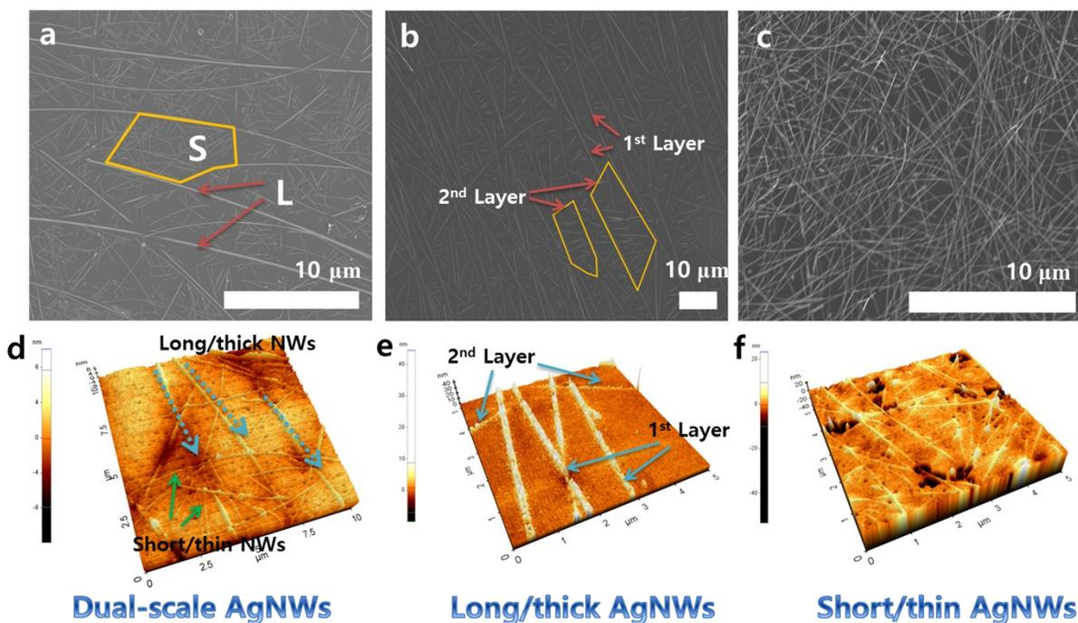
**Figure S4** SEM and AFM analyses of fabricated transparent conductor using (a, d) dual-scale AgNW percolation network, (b,e) only long/thick AgNW percolation network, and (c,f) only short/thin AgNWs percolation network.
