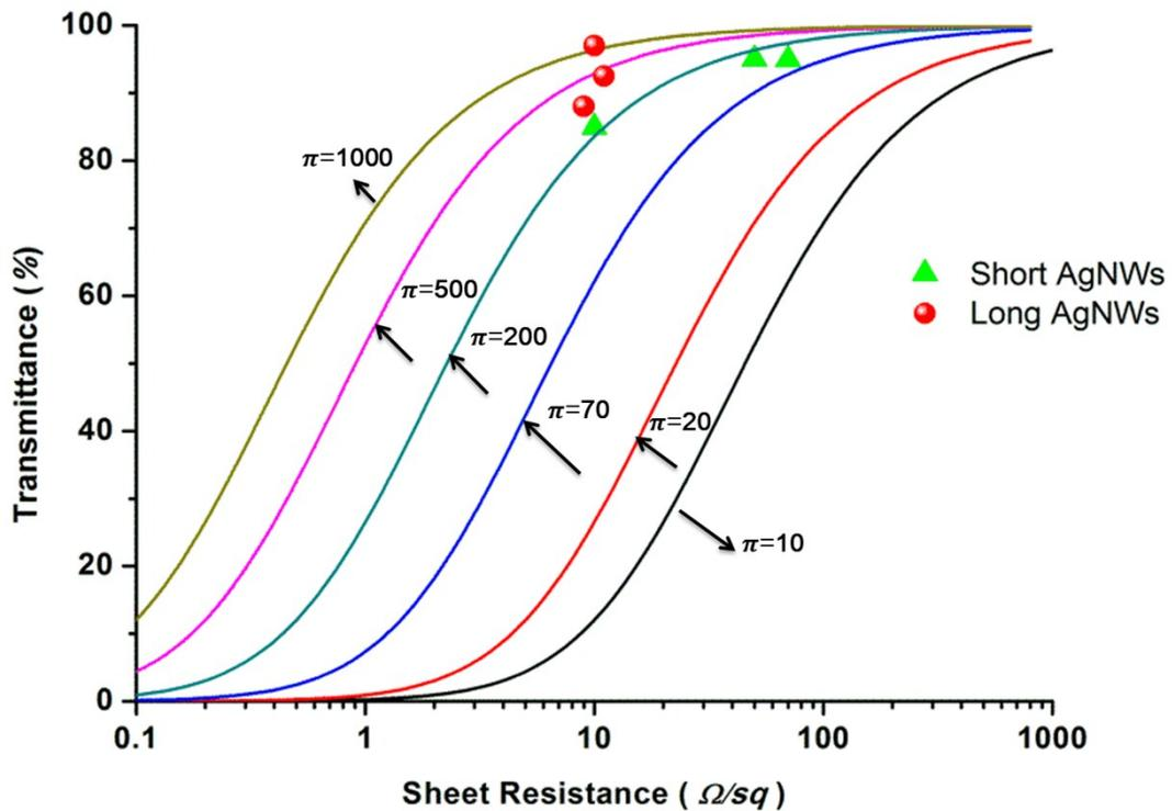
**Figure S3** Plotted figure of merit based on calculation (eq.1) and FOMs of fabricated electrodes
