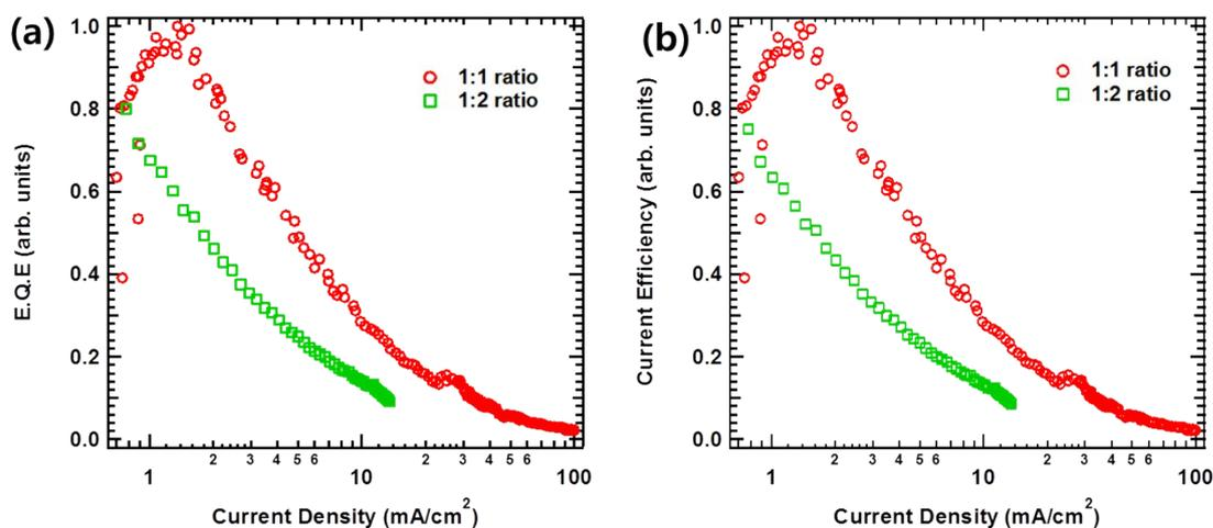
Figure S7. OLED characterization in (a) E.Q.E. and (b) current efficiency based on different AgNWs ratio.
