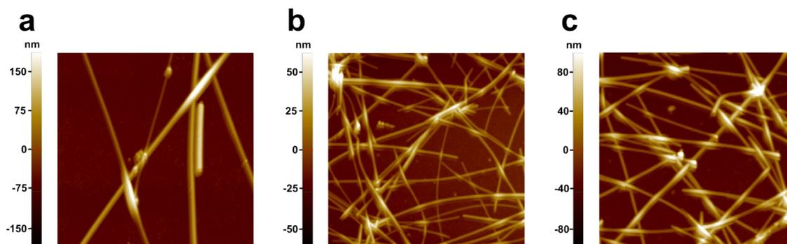
**Figure S5.** AFM topography information of AgNWs network before embedding (a) long/thick AgNWs (b) short/thin AgNWs (c) dual-scale AgNWs.
