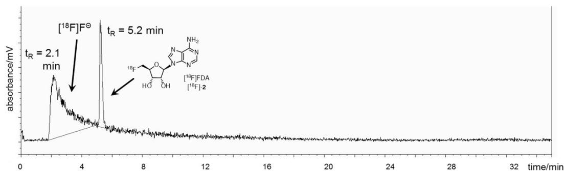
**Figure S61.** HPLC radioactivity trace of the control reaction where the fluorinase (20 mg.mL<sup>-1</sup>) was incubated with only [<sup>18</sup>F]fluoride for 30 min. [<sup>18</sup>F]FDA [<sup>18</sup>F]-2 was observed at  $t_R = 5.2$  min. Run with under gradient conditions.
