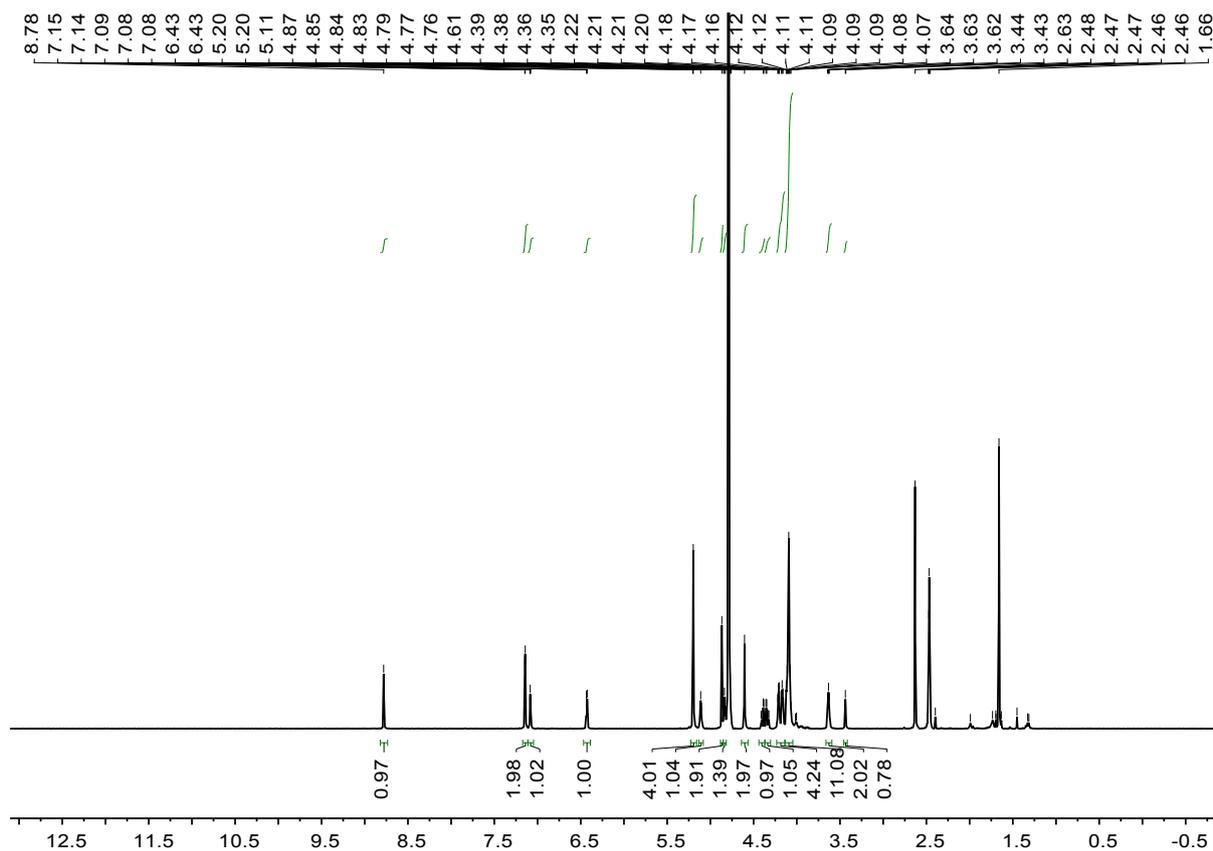
**Figure S31.**  $^1\text{H}$  NMR spectrum (500.1 MHz, 1:1  $\text{D}_2\text{O}:\text{d}_3\text{-MeCN}$ ) of **22**. The large peak at 1.6 ppm is residual  $t\text{-BuOH}$  from the freeze drying process.
