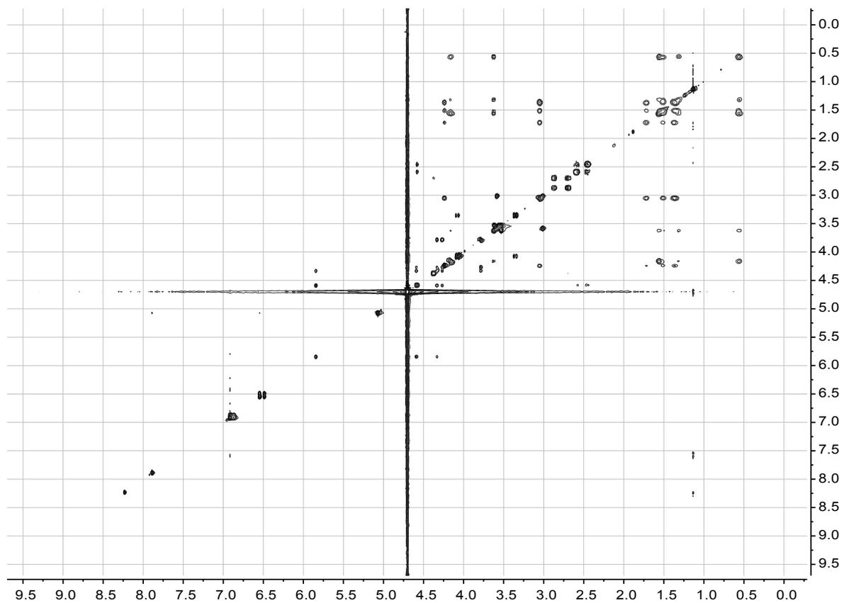
**Figure S46.** TOCSY NMR spectrum (500.1 MHz, D<sub>2</sub>O, 90ms mixing time) of **30**.
