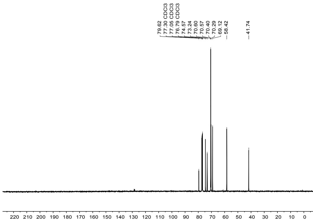
Figure S16.  $^{13}\text{C}$  NMR spectrum (125.8 MHz,  $\text{CDCl}_3$ ) of **14**.
