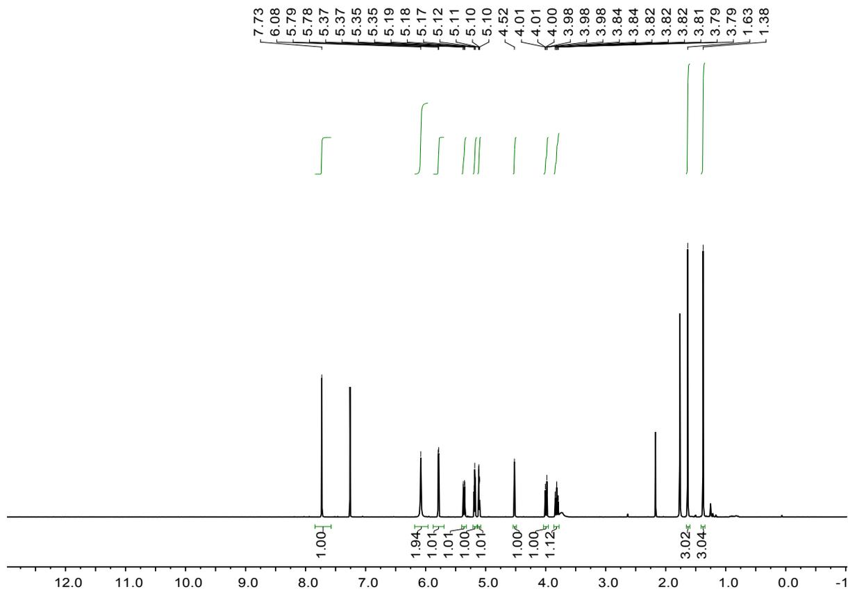
Figure S23.  $^1\text{H}$  NMR spectrum (500.1 MHz,  $\text{CDCl}_3$ ) of **19**.
