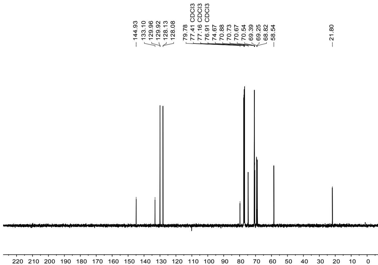
Figure S12.  $^{13}\text{C}$  NMR spectrum (125.8 MHz,  $\text{CDCl}_3$ ) of **13**.
