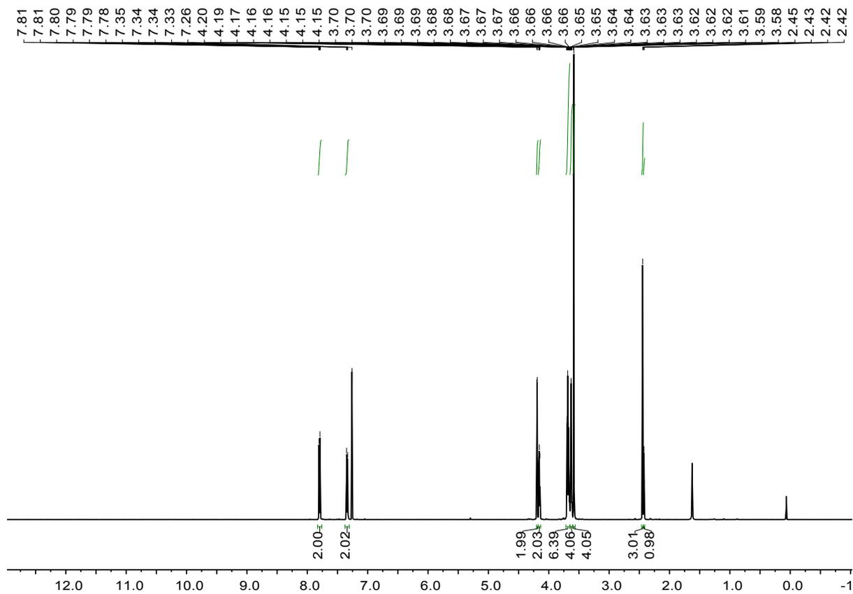
Figure S11.  $^1\text{H}$  NMR spectrum (500.1 MHz,  $\text{CDCl}_3$ ) of **13**.
