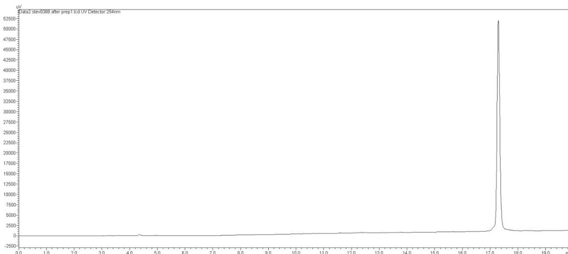
**Figure S33.** HPLC trace (254 nm) of **22** after purification.
