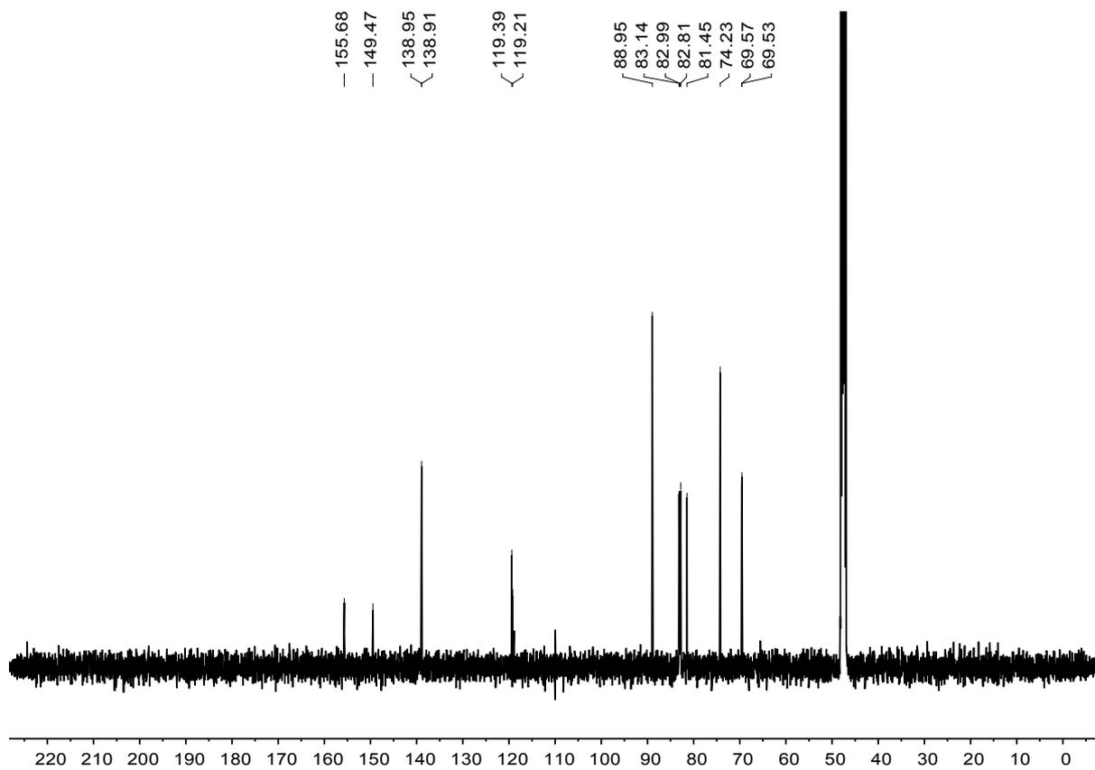
Figure S29.  $^{13}\text{C}$  NMR spectrum (125.8 MHz,  $d_4$ -MeOD) of **20**.
