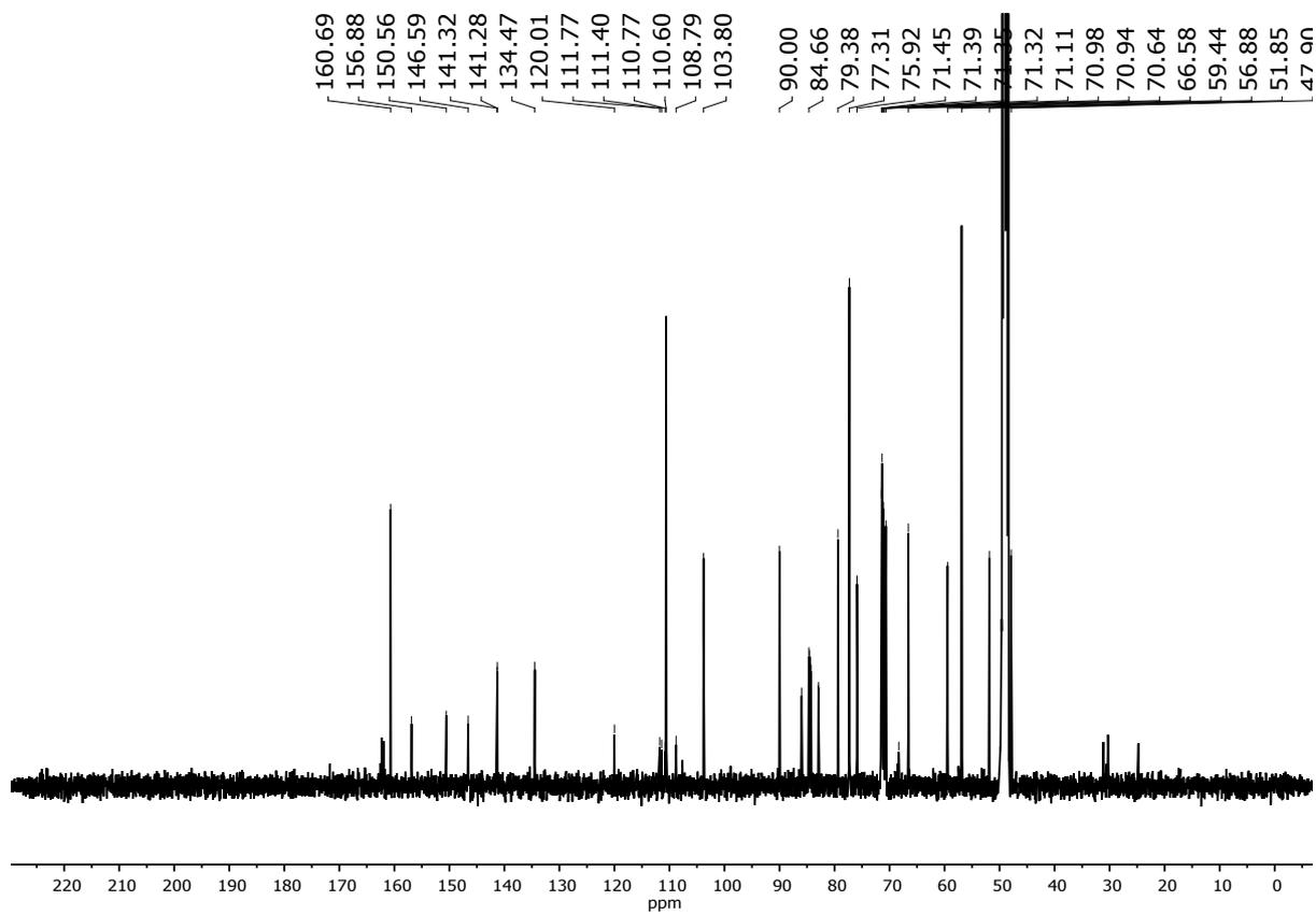
**Figure S38.**  $^{13}\text{C}$  NMR spectrum (125.7 MHz,  $d_4$ -MeOD) of **24**.
