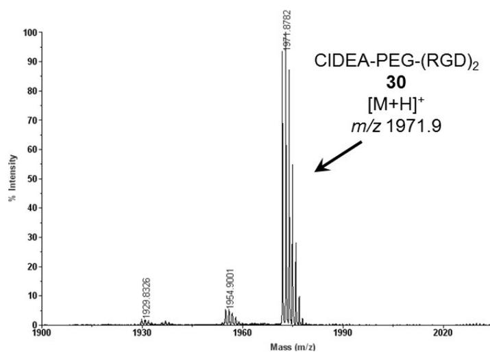
**Figure S48.** MALDI-TOF MS spectrum of **30** after purification, showing the  $[M+H]^+$  ion at  $m/z = 1971.9$ . MALDI-TOF MS acquired by the University of St Andrews Mass Spectrometry Service.
