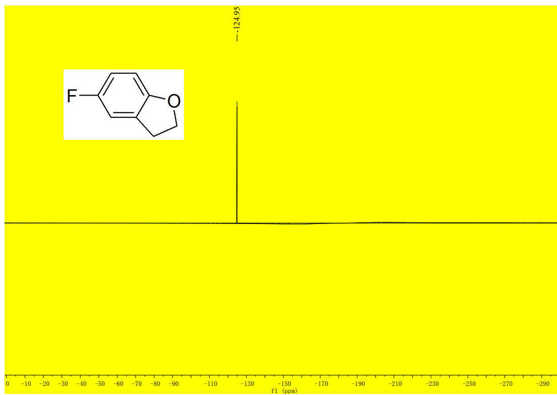
Figure S48. ^{19}\text{F} NMR spectrum of 5-fluoro-2,3-dihydrobenzofuran in \text{CDCl}_3 .
