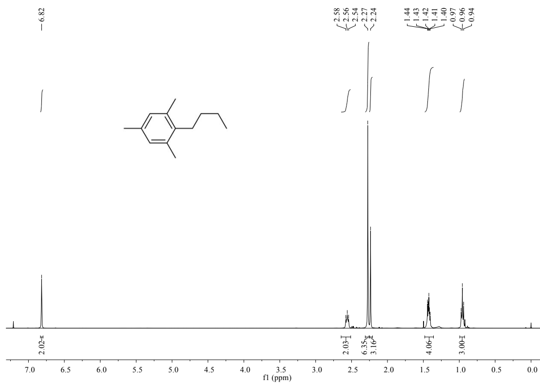
Figure S32. 1 H NMR spectrum of Butylmesitylene in CDCl 3 . 12
