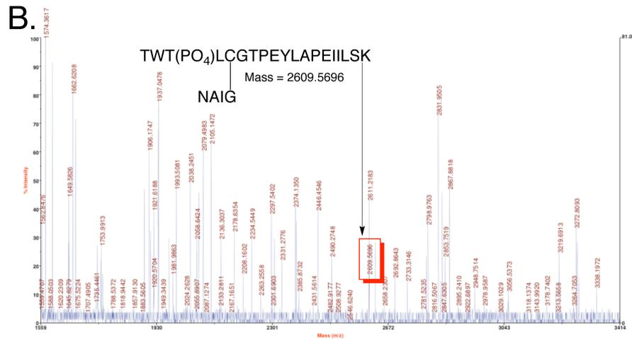
MALDI Spectra for untreated PKAC $\alpha$  control (A.) and PKAC $\alpha$  treated with Inhibitor 1 (B.).
