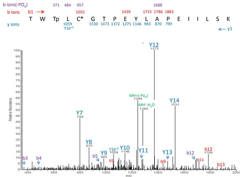
**Results:** Analysis of the modified sample yielded coverage of 73.24 % of the PKAC $\alpha$  sequence as mapped by high confidence identification of tryptic peptides. The peptide containing Cys199 was observed with the appropriate mass change to confirm modification with the Asn-Ala-Ile-Gly amino acids of **1** with a high confidence (Xcoor of 4.075).
