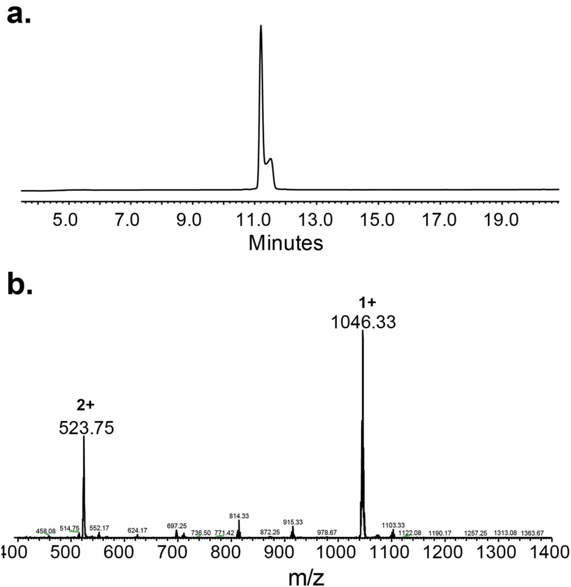
**Figure S3.** Analytical HPLC (**a**) and ESI-MS (**b**) of the purified peptide C6U. Similar conditions for Figure S2 were used. Calc. mass 1045.32, observed 1045.41.
