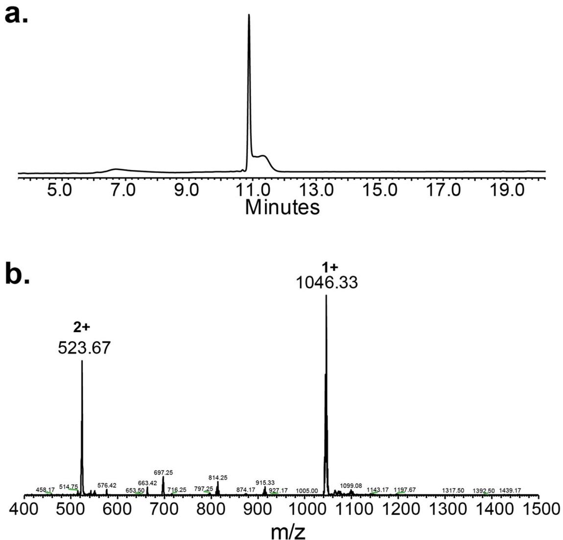
**Figure S2.** Analytical HPLC (a) and ESI-MS (b) of the purified peptide C3U. Prior to HPLC analysis, the peptide was reduced with TCEP in the presence of sodium ascorbate to prevent possible deselenization side-reaction.<sup>9</sup> Under these conditions, the peptide is mainly in the reduced form. Calc. mass 1045.32, observed 1045.33. The shoulder on the right of the main peak showed a mass for oxidized dimeric peptide.
