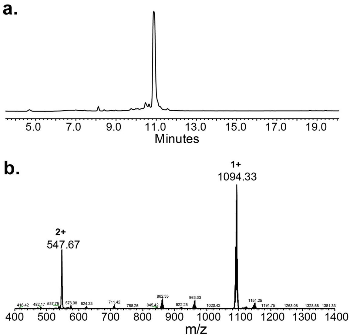
**Figure S4.** Analytical HPLC (**a**) and ESI-MS (**b**) of the purified peptide C3U/C6U. Similar conditions for Figure S2 and S3 were used. Calc. mass 1093.27, observed 1093.33.
