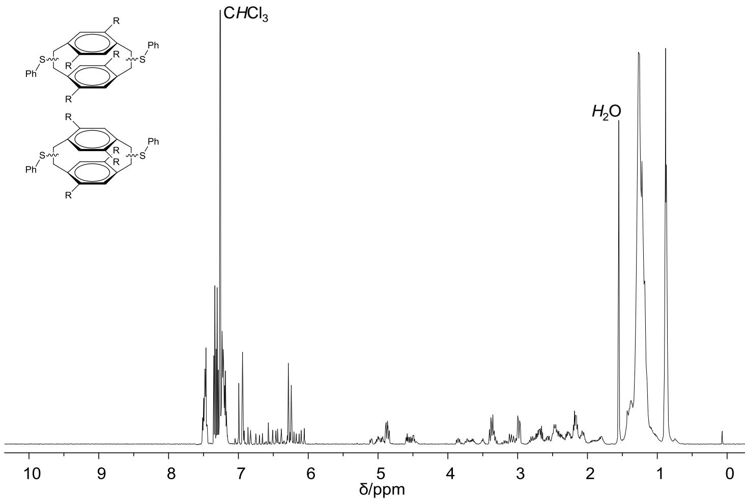
**31.  $^1\text{H}$  NMR ( $\text{CDCl}_3$ , 400 MHz) Spectrum of Oxidation of Phenyl Sulfides of Compound 18 (19)**
