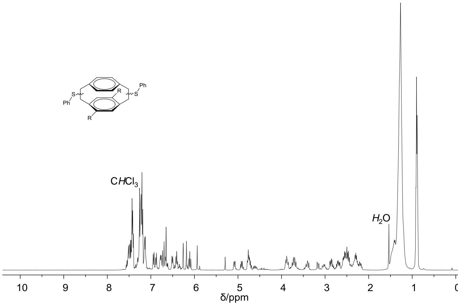
**25.  $^1\text{H}$  NMR ( $\text{CDCl}_3$ , 500 MHz) Spectrum of Oxidation of Phenyl Sulfides of Compound 13 (14)**
