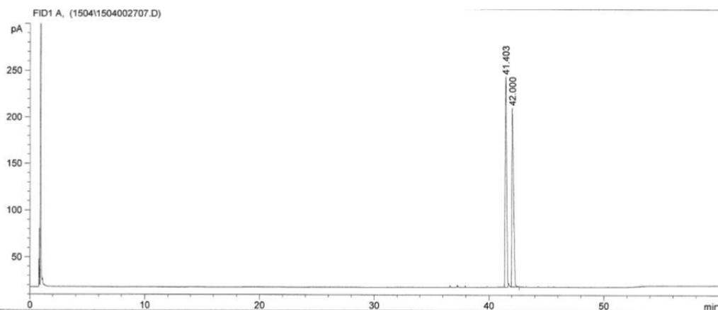
**Figure S8.** Chiral GC of the conversion of *rac*-1b with *ee* = 0%.
