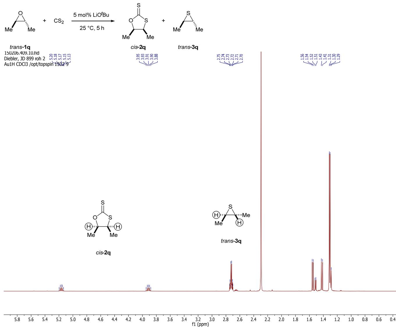
Figure S6. <sup>1</sup>H-NMR spectrum of the crude reaction mixture of the conversion of *trans-1q* and characteristic resonances of *cis-2q* and *trans-3q*.<sup>1,2</sup>
