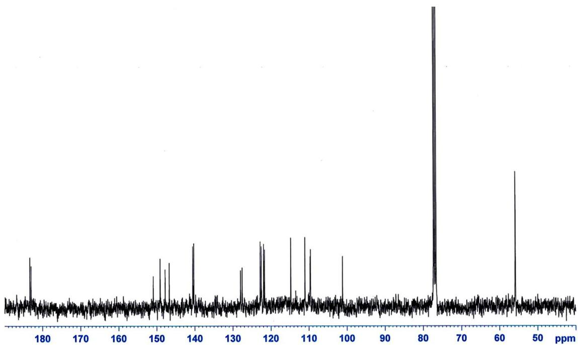
**Compound 5.** 100.62 MHz  $^{13}\text{C}$  NMR of **5** in  $\text{CDCl}_3$  at room temperature. The spectrum shows many split signals due to the asymmetry of the molecule, including the two signals at 183.36 and 183.05 ppm attributed to the keto-enol carbonyls of **5**.
