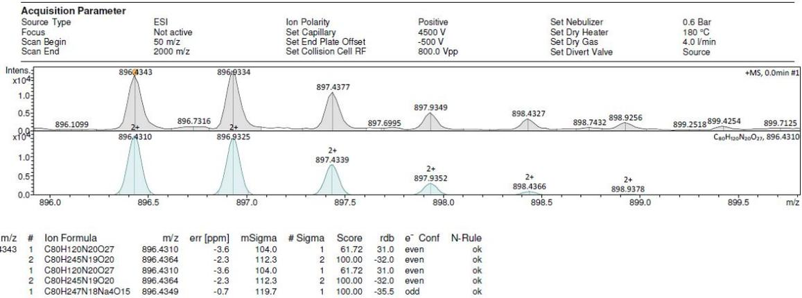
**Figure S23.** RP-HPLC and HRESI-MS traces of peptide **25**, linear gradient of 5%B to 65%B over 30 min, *ca* 2%B per minute.
