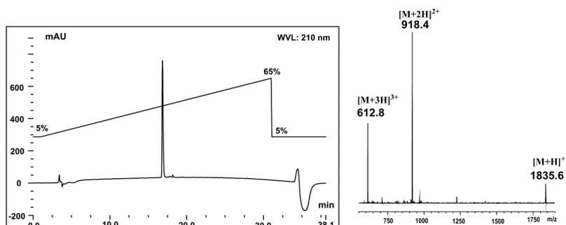
**Figure S18.** RP-HPLC and ESI-MS traces of peptide **20**, linear gradient of 5%B to 65%B over 30 min, *ca* 2%B per minute.
