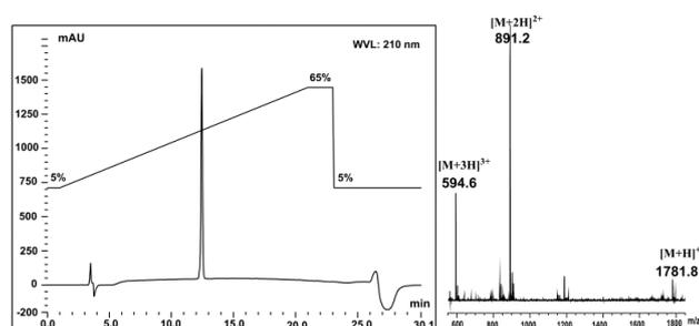
**Figure S9.** RP-HPLC and ESI-MS traces of peptide **9**, linear gradient of 5%B to 65%B over 20 min, *ca* 3%B per minute.
