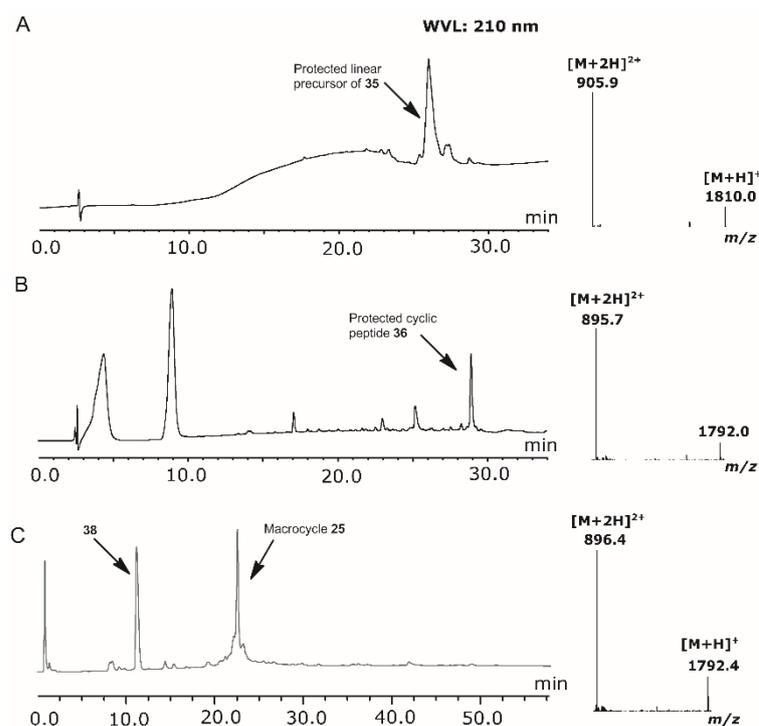
**Figure S27.** Analytical LC-MS chromatograms for the synthesis of macrocycle **25**. (A) The linear peptide **35**; (B) crude cyclic peptide **36**, analysed by Agilent Zorbax 300SB-C<sub>3</sub> column (3.0 x 150 mm; 3.5  $\mu$ m), gradient 5-95% B over 30 min, 0.3 mL min<sup>-1</sup> flow rate; (C) The condensation reaction to yield **25**, analysed by Agilent Zorbax 300SB-C<sub>3</sub> column (3.0 x 150 mm; 3.5  $\mu$ m), gradient 5-65% B over 60 min, 0.3 mL min<sup>-1</sup> flow rate.
