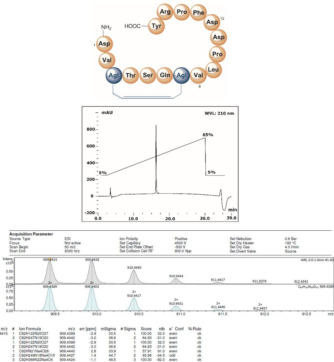
**Figure S24.** RP-HPLC and HRESI-MS traces of peptide **26**, linear gradient of 5%B to 65%B over 30 min, ca 2%B per minute.
