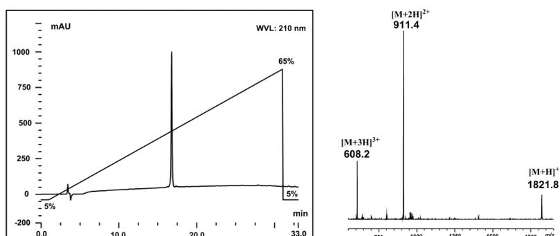
**Figure S20.** RP-HPLC and ESI-MS traces of peptide **22**, linear gradient of 5%B to 65%B over 30 min, *ca* 2%B per minute.
