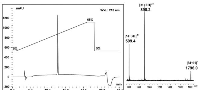
**Figure S8.** RP-HPLC and ESI-MS traces of peptide **8**, linear gradient of 5%B to 65%B over 20 min, *ca* 3%B per minute.
