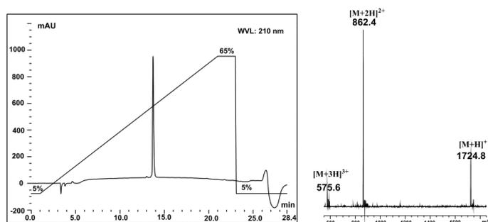
**Figure S16.** RP-HPLC and ESI-MS traces of peptide **16**, linear gradient of 5%B to 65%B over 20 min, *ca* 3%B per minute.
