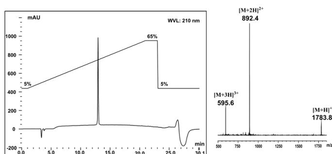
**Figure S11.** RP-HPLC and ESI-MS traces of peptide **11**, linear gradient of 5%B to 65%B over 20 min, *ca* 3%B per minute.
