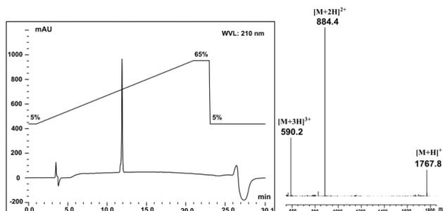
**Figure S10.** RP-HPLC and ESI-MS traces of peptide **10**, linear gradient of 5%B to 65%B over 20 min, *ca* 3%B per minute.
