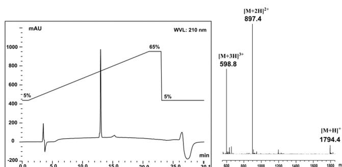
**Figure S6.** RP-HPLC and ESI-MS traces of peptide **6**, linear gradient of 5%B to 65%B over 20 min, *ca* 3%B per minute.
