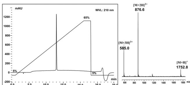
**Figure S7.** RP-HPLC and ESI-MS traces of peptide **7**, linear gradient of 5%B to 65%B over 20 min, *ca* 3%B per minute.
