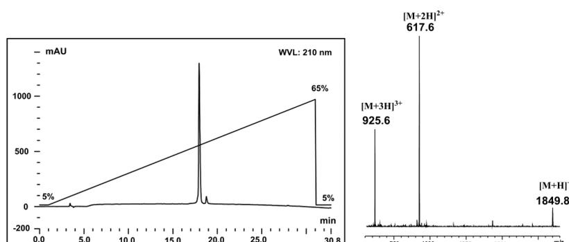
**Figure S19.** RP-HPLC and ESI-MS traces of peptide **21**, linear gradient of 5%B to 65%B over 30 min, *ca* 2%B per minute.
