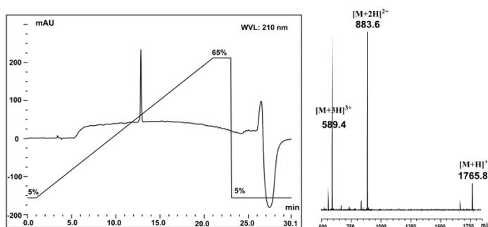
**Figure S12.** RP-HPLC and ESI-MS traces of peptide **12**, linear gradient of 5%B to 65%B over 20 min, *ca* 3%B per minute.
