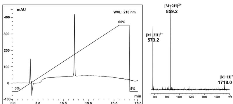
**Figure S17.** RP-HPLC and ESI-MS traces of peptide **17**, linear gradient of 5%B to 65%B over 20 min, *ca* 3%B per minute.
