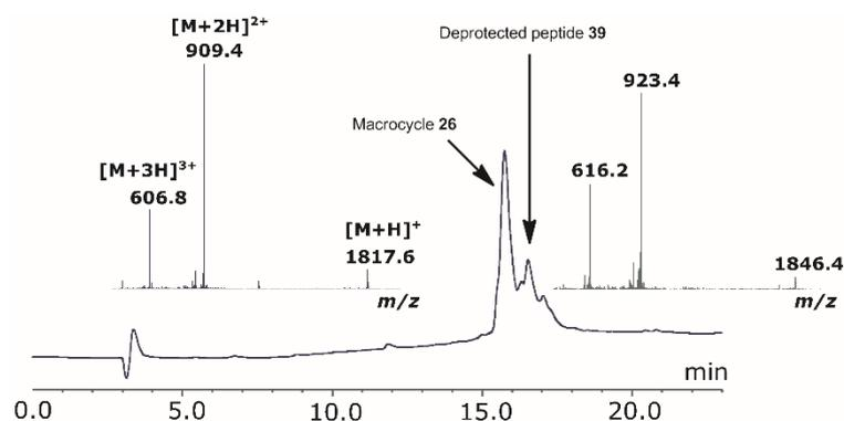
**Figure S28.** Analytical LC-MS chromatograms for the synthesis of macrocycle **26** showing the mass and retention time difference between **26** and its linear precursor. Analysed by Agilent Zorbax 300SB-C<sub>3</sub> column (3.0 x 150 mm; 3.5  $\mu$ m), gradient 1-61% B over 20 min, 0.3 mL min<sup>-1</sup> flow rate.
