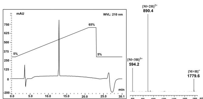
**Figure S5.** RP-HPLC and ESI-MS traces of peptide **5**, linear gradient of 5%B to 65%B over 20 min, *ca* 3%B per minute.
