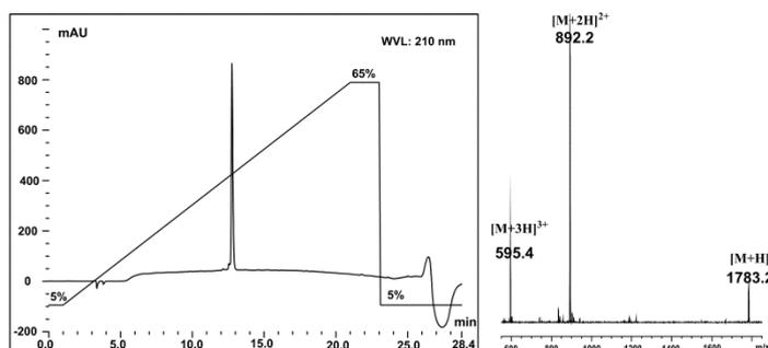
**Figure S15.** RP-HPLC and ESI-MS traces of peptide **15**, linear gradient of 5%B to 65%B over 20 min, *ca* 3%B per minute.
