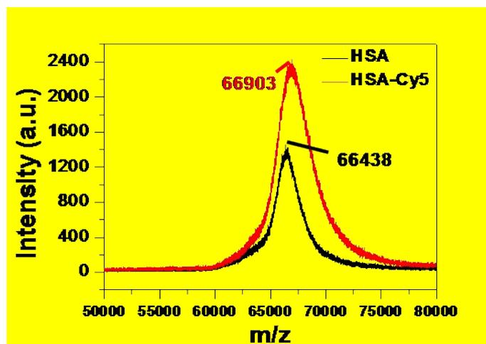
**Fig. S6** MALDI-TOF MS spectra for HSA and Cy5 labeled HSA (the red line). The results revealed a difference in mass of HSA after covalent linkage with Cy5, which were consistent with the successful formation of Cy5 labeled HSA.
