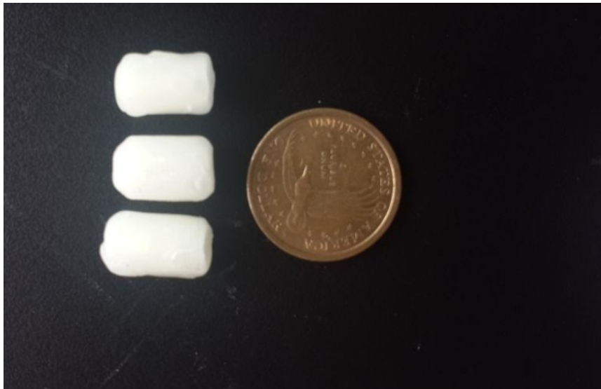
Figure S3. The finished paraffin wax capsule.
