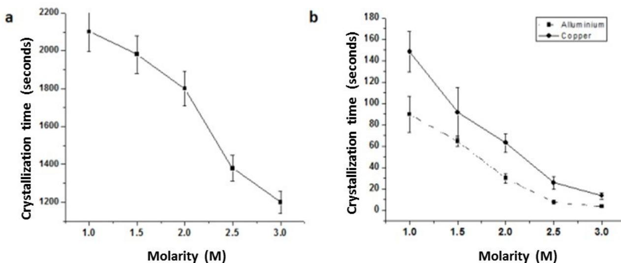
**Figure 1. Effect of concentration on crystallization time.** The time required to obtain crystals for different concentrations of glycine is shown in (a) control (b) under laser with copper as well as aluminum wire.
