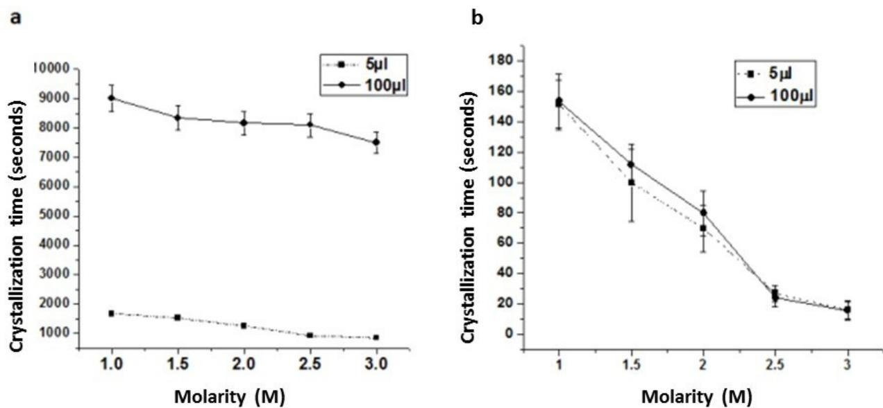
**Figure 2. Effect of drop size on crystallization time.** Crystallization time with respect to different sample volume for various concentrations of glycine is shown in (a) control, (b) under laser with copper wire. For the clarity purpose, only 5  $\mu$ l and 100  $\mu$ l is drop sizes are shown.
