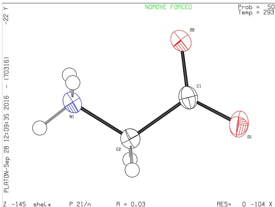
**Figure 5:** The structure of  $\alpha$ -glycine, showing 50% probability displacement ellipsoid and the atom-numbering scheme.
