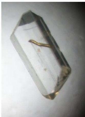
**Figure 4:** Laser-induced glycine crystal formed around the nucleant aluminum wire
