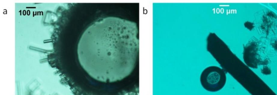
**Figure 3.** (a) Glycine crystal formation on the surface of the bubble, (b) Crystal formation away from the bubble.
