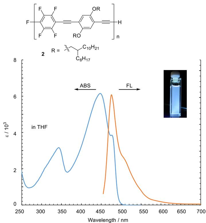
**Fig. S5** UV-Vis and fluorescence spectra of **2** in THF (blue line: UV-vis; orange line: fluorescence excited at 445 nm). The inset shows a photograph of **2** in a THF solution under irradiation with UV light at a wavelength of 365 nm.
