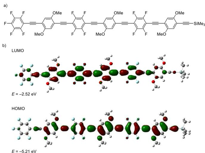
**Fig. S6** (a) The chemical structure of the model compound for the calculation. (b) MO diagrams of the model compound based on the DFT calculations (B3LYP/6-31G(d,p)//B3LYP/6-31G(d,p)).
