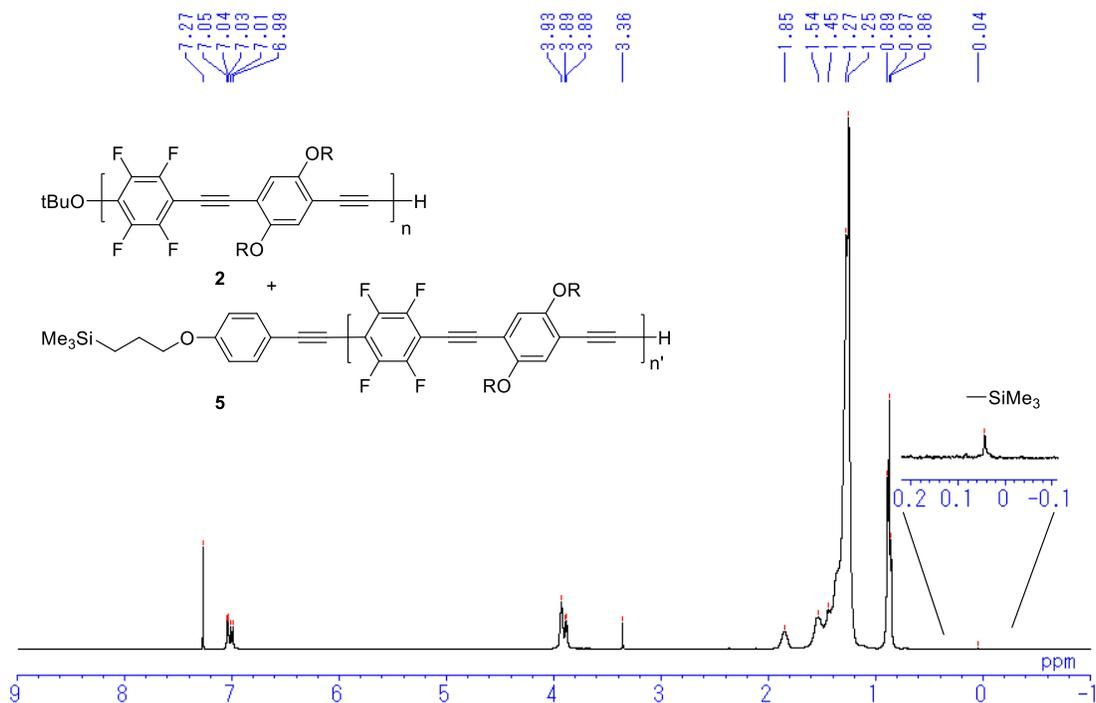
**Fig. S4**  $^1\text{H}$  NMR spectrum of the polymer obtained by the polymerization of **1** with 5 mol % *t*-BuOK/10 mol% cryptand[2.2.2] in the presence of 5 mol % **4** in THF at room temperature for 90 s.
