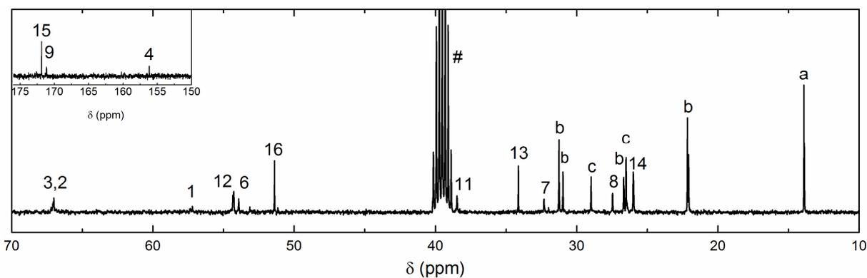
Figure S 12.  $^{13}\text{C}$  NMR spectrum of trialkylamino thioether **3**. Recorded in  $\text{DMSO-d}_6$  (#).
