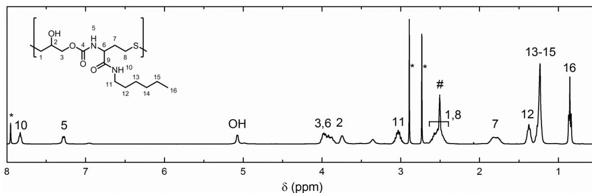
Figure S 17.  $^1\text{H NMR}$  spectrum of poly(TEU). Recorded in  $\text{DMSO-}d_6$  (#). Residual solvent peaks: \* DMF.
