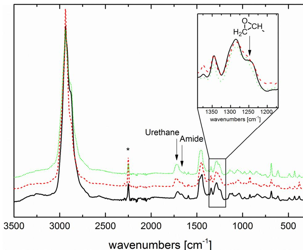
Figure S 26. Raman spectra of hydrogels obtained by thiol-epoxy polymerization (solid black line), and by multicomponent reaction using thiol-ene Michael addition with a PEG(X) diamine and TMPT (X = 2, dashed red line; X = 7, dotted green line). Inset graph shows the ring stretch band of the monosubstituted epoxide.
