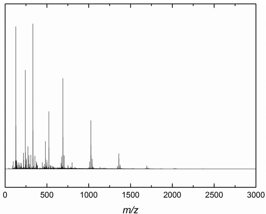
Figure S 25. MALDI-TOF MS spectrum of poly(sulfoxide urethane)s obtained through oxidation with H<sub>2</sub>O<sub>2</sub>.
