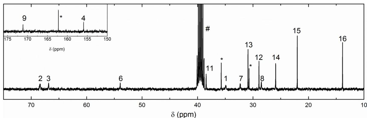
Figure S 18.  $^{13}\text{C NMR}$  spectrum of poly(TEU). Recorded in  $\text{DMSO-}d_6$  (#). Residual solvent peaks: \* DMF.
