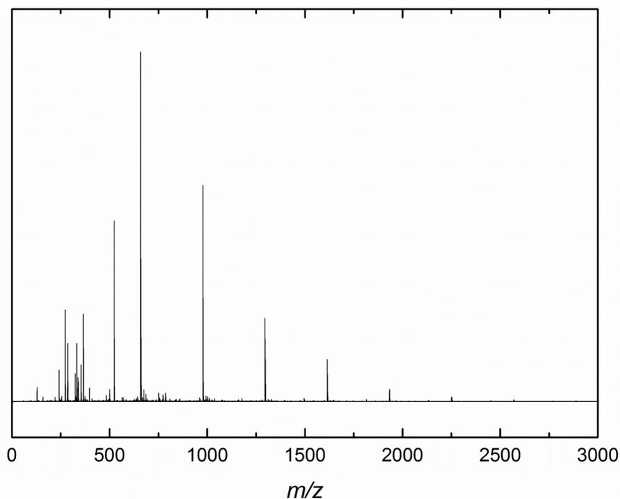
Figure S 24. MALDI-TOF MS spectrum of poly(thioether urethane) prior oxidation by H<sub>2</sub>O<sub>2</sub>.
