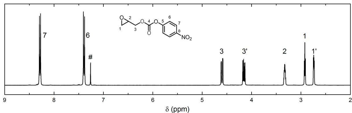
Figure S 1. <sup>1</sup>H NMR spectrum of *p*-nitrophenyl glycidyl carbonate. Recorded in chloroform-*d* (#).
