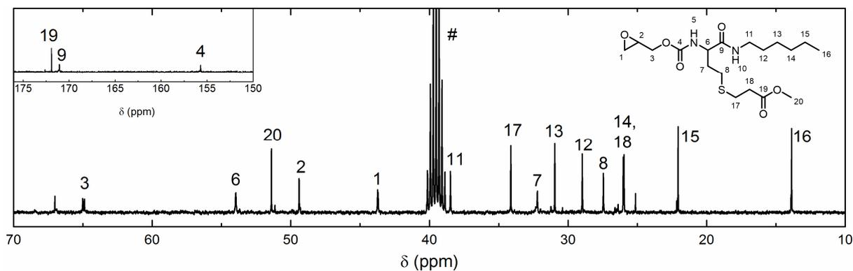
Figure S 8.  $^{13}\text{C}$  NMR spectrum of epoxy thioether **2**. Recorded in  $\text{DMSO-}d_6$  (#).
