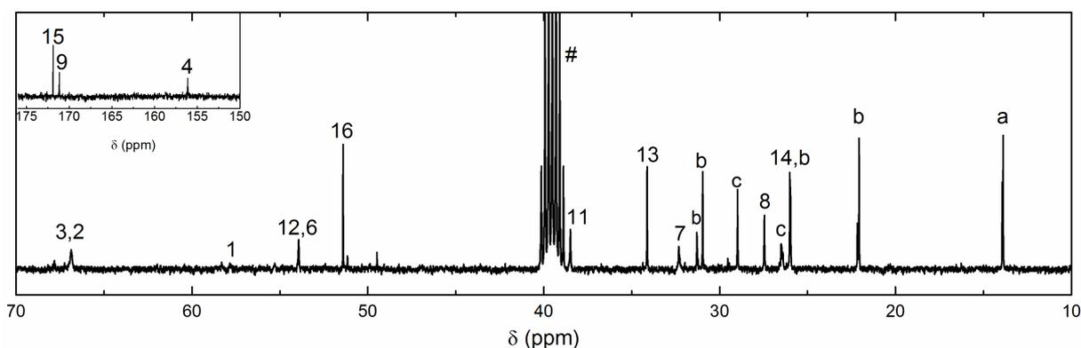
Figure S 16.  $^{13}\text{C}$  NMR spectrum of trialkylamino *bis*(thioether) **4**. Recorded in DMSO- $d_6$  (#).
