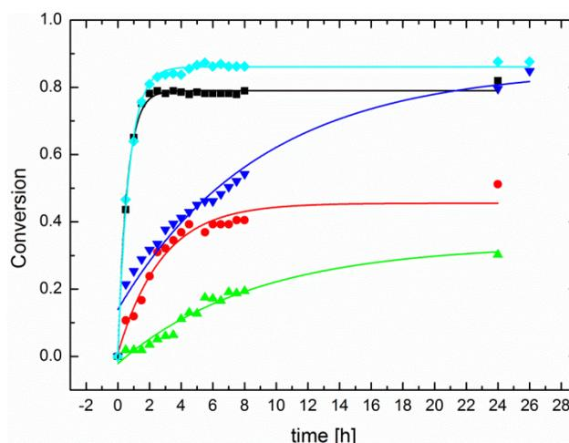
Figure S 19. Conversion Vs. time plot of the thiol-epoxy reaction using 3 mol% of LiOH (■), TBD (●), NaOEt (▲), DBU (▼) and KO $^t$ Bu (◆) as base.
