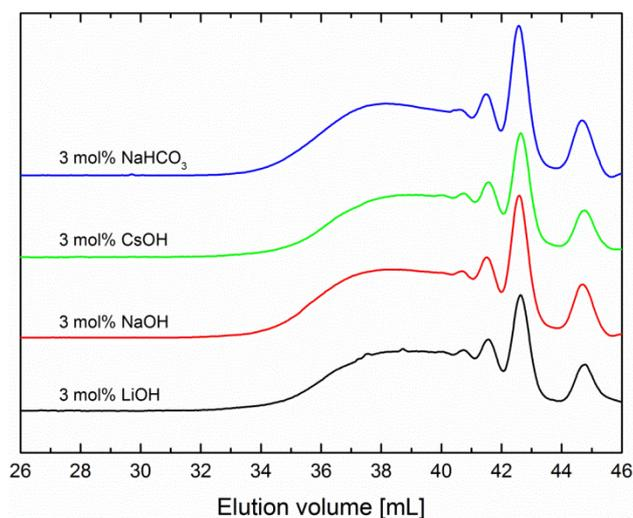
Figure S 20. Influence of the alkaline catalysts on the SEC elution curves of the resulting poly(thioether urethane)s.
