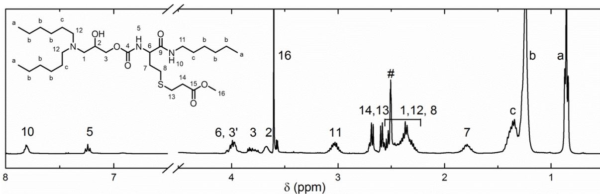
Figure S 11.  $^1\text{H}$  NMR spectrum of trialkylamino thioether **3**. Recorded in  $\text{DMSO-d}_6$  (#).
