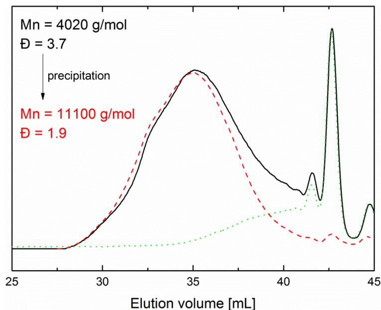
Figure S 23. Precipitation of poly(TEU) from DMF in MeCN showing the elugram of the crude unpurified poly(TEU) (solid black line), the purified polymer (dashed red line) and the mother liquor (dotted green line). Synthesis conditions:  $c(\mathbf{1}) = 0.25$  M, H<sub>2</sub>O/MeCN (70:30), RT, 24 h, 3 mol% LiOH, 1 eq hexyl amine.
