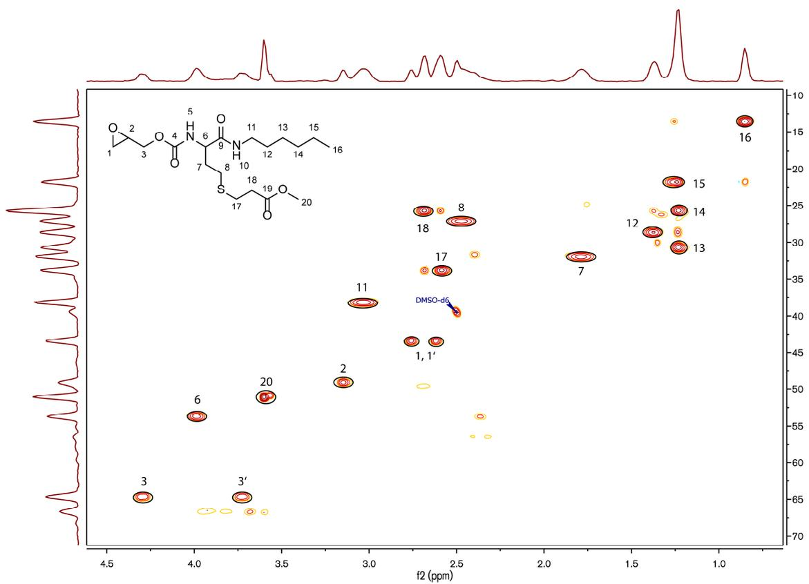
Figure S 10. HSQC spectrum of epoxy thioether **2**. Recorded in DMSO-d<sub>6</sub>.
