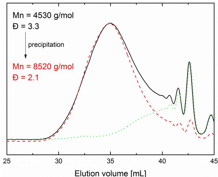
Figure S 22. Precipitation of poly(TEU) from DMF in MeCN showing the elugram of the crude unpurified poly(TEU) (solid black line) the purified polymer (dashed red line) and the mother liquor (dotted green line). Synthesis conditions:  $c(\mathbf{1}) = 1.50$  M, THF/H<sub>2</sub>O (90:10), RT, 24 h, 3 mol% LiOH, 1 eq hexyl amine.
