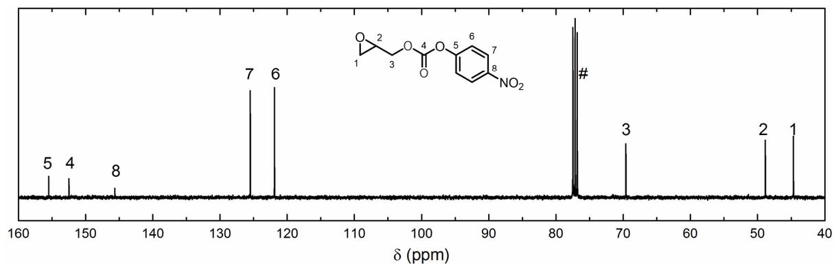
Figure S 2. <sup>13</sup>C NMR spectrum of *p*-nitrophenyl glycidyl carbonate. Recorded in chloroform-*d* (#).
