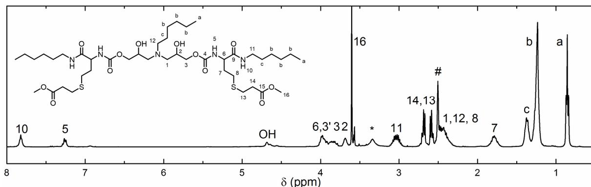
Figure S 15.  $^1\text{H}$  NMR spectrum of trialkylamino *bis*(thioether) **4**. Recorded in DMSO- $d_6$  (#). Residual solvent peaks: \*  $\text{H}_2\text{O}$ .
