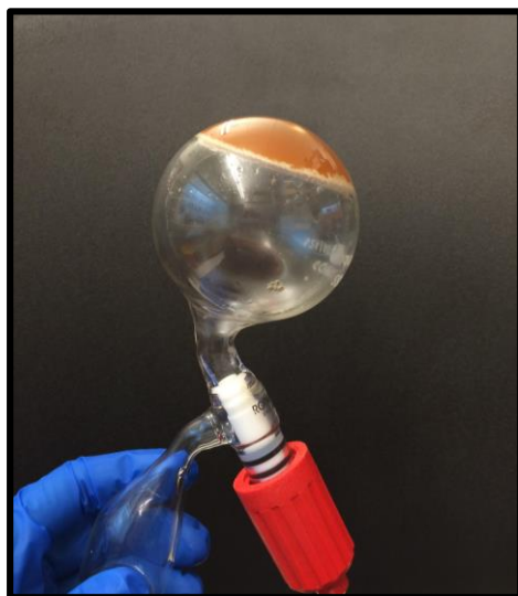
Figure S4. Gelation of poly(styrene oxide)- b -poly( \epsilon -caprolactone) prepared by sequential addition via the new adapted organocatalyst switch approach using DMSO as solvent after 10 h upon addition of \epsilon -CL monomer due to formation of intra/intermacromolecular esterification
