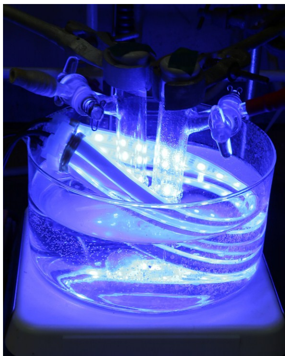
Figure S1. Representative configuration comprising reaction vial surrounded by LED strips (10 W, 460-470 nm).
