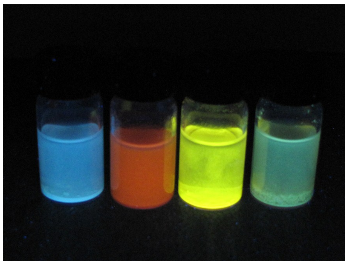
Fig. S6 The photographs of the four CS-CMPs suspended in dichloromethane. (from left to right are: Bn-CS-CMP , TPA-CS-CMP , TPE-CS-CMP , and TPM-CS-CMP )
