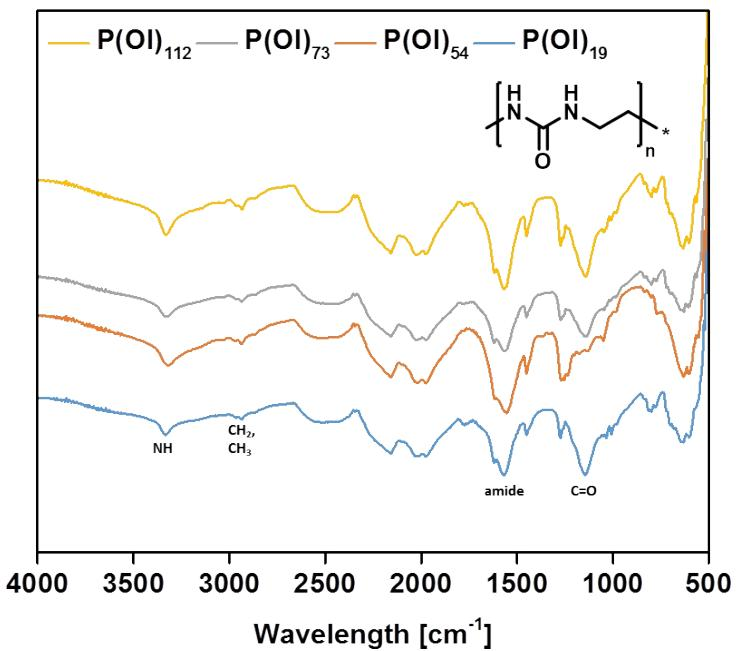
**Figure S12:** Normalized FTIR spectra of the purified  $P(OI)_n$  (3a-d).
