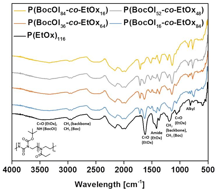
**Figure S24:** Normalized FTIR spectra of the purified  $P(BocOI_n-co-EtOx_m)$  precursors (**4a-d**) and  $P(EtOx)_{116}$  (**6**).
