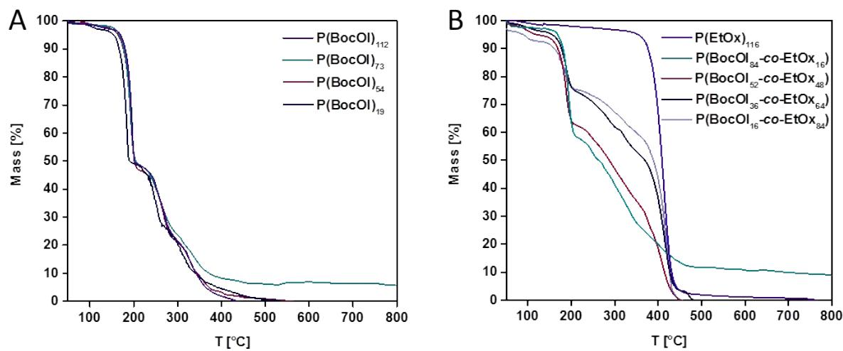
**Figure S26:** TGA traces of the Boc protected A: homopolymers (**2a-d**) and B: copolymers (**4a-d**) and  $P(EtOx)_{116}$  (**6**).
