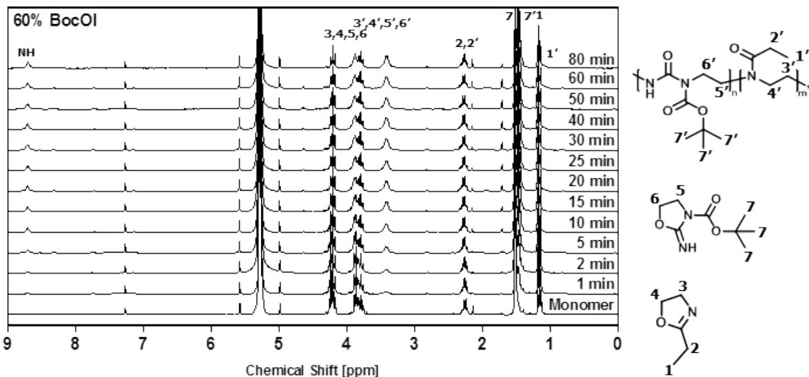
**Figure S18:** <sup>1</sup>H-NMR shifts ( $\text{CDCl}_3$ , 300 MHz) of time dependent P(BocOI-*co*-EtOx) kinetics in  $\text{CH}_2\text{Cl}_2$  at 100 °C with  $[\text{M}]/[\text{I}] = 60$  aiming 60% BocOI, recorded at RT.
