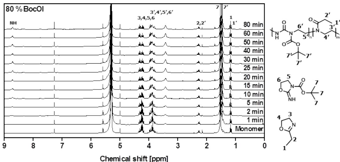
**Figure S19:** <sup>1</sup>H-NMR shifts ( $\text{CDCl}_3$ , 300 MHz) of time dependent P(BocOI-*co*-EtOx) kinetics in  $\text{CH}_2\text{Cl}_2$  at 100 °C with  $[\text{M}]/[\text{I}] = 60$  aiming 80% BocOI, recorded at RT.
