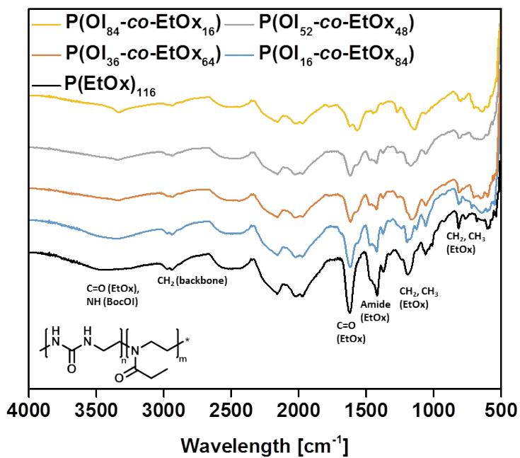
**Figure S25:** Normalized FTIR spectra of the purified  $P(OL_n\text{-}co\text{-}EtOx_m)$  (**5a-d**) and  $P(EtOx)_{116}$  (**6**).
