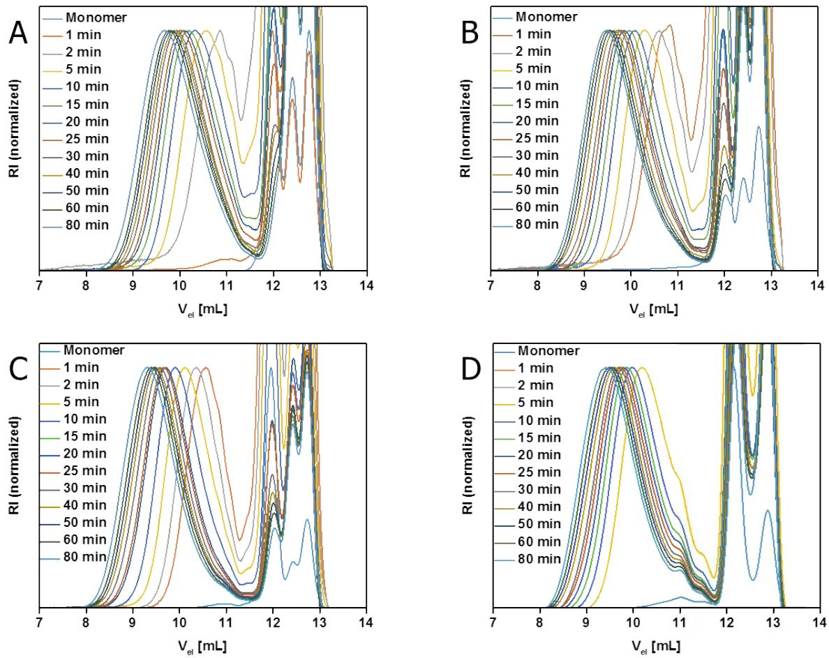
**Figure S15:** SEC-traces ( $\text{CHCl}_3$ -*i*-PrOH, PS-cal.; 1<sup>st</sup> system peak after 12 mL) of time dependent  $\text{P}(\text{BocOI}_n\text{-co-}\text{EtOx}_m)$  kinetics in  $\text{CH}_2\text{Cl}_2$  at 100 °C bearing different monomer ratios (**A**: 20% BocOI, **B**: 40% BocOI, **C**: 60% BocOI, **D**: 80% BocOI).
