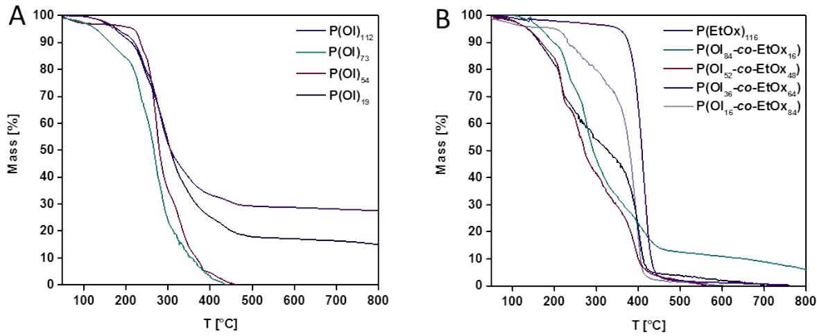
**Figure S27:** TGA traces of the deprotected **A**: homopolymers (**3a-d**) and **B**: copolymers (**5a-d**) and P(EtOx)<sub>116</sub> (**6**).
