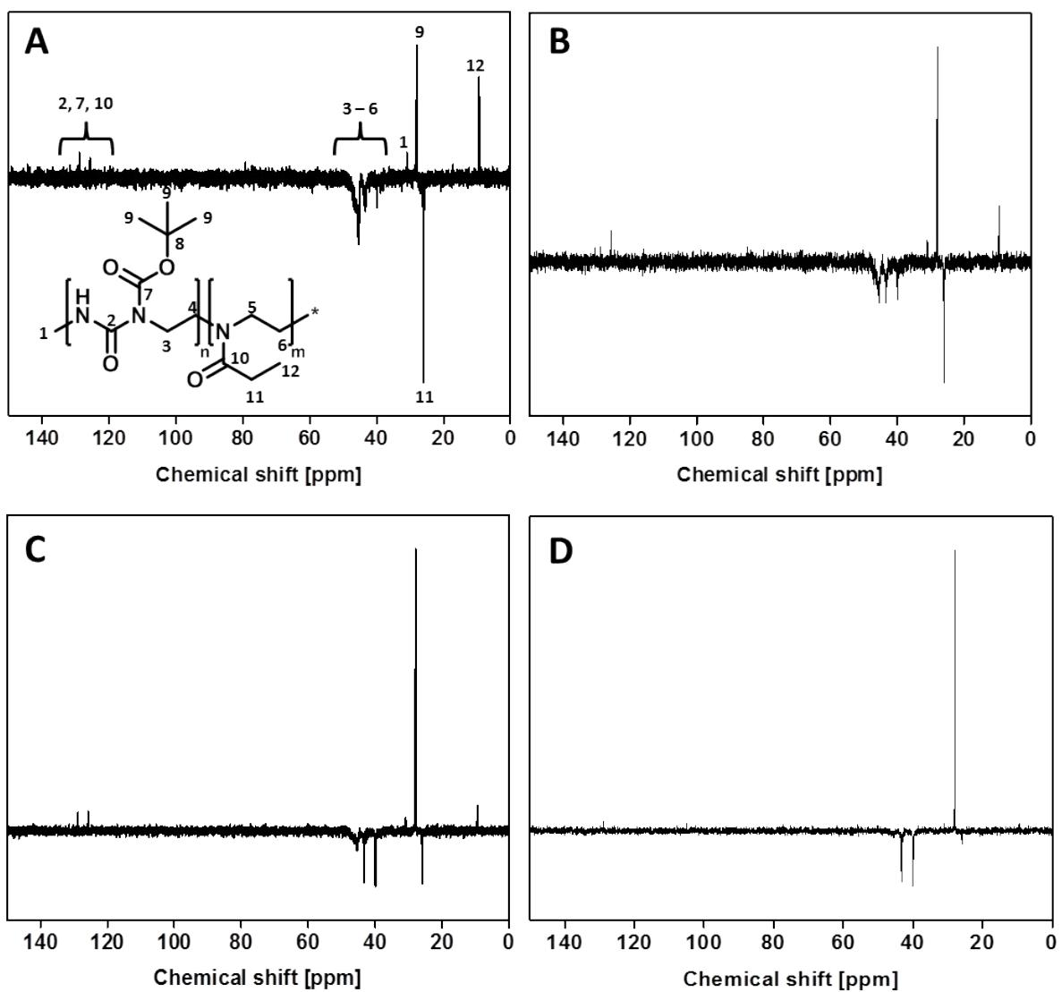
**Figure S21:**  $^{13}\text{C}$ -NMR ( $\text{CDCl}_3$ , 300 MHz) spectra of the purified  $P(\text{BocOI}_n\text{-co-}\text{EtOx}_m)$ . **A: 4a.** **B: 4b.** **C: 4c.** **D: 4d.**
