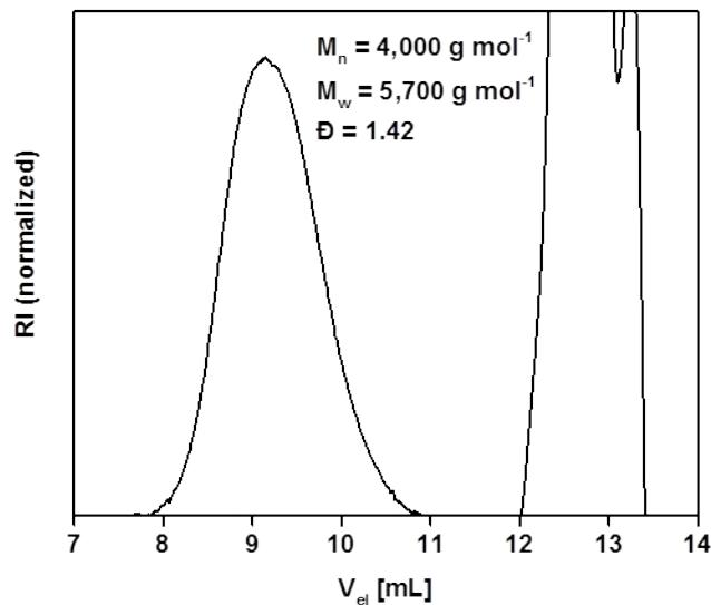
**Figure S31:** SEC-trace ( $\text{CHCl}_3$ -*i*-PrOH, PS-cal.; 1<sup>st</sup> system peak after 12 mL) of  $\text{P}(\text{BocOI})_{300}$ .
