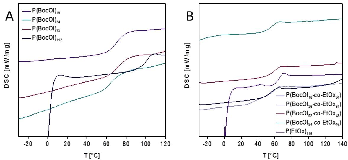
**Figure S28:** DSC traces of the Boc-protected **A**: homopolymers (**2a-d**) and **B**: copolymers (**4a-d**) and P(EtOx)<sub>116</sub> (**6**).
