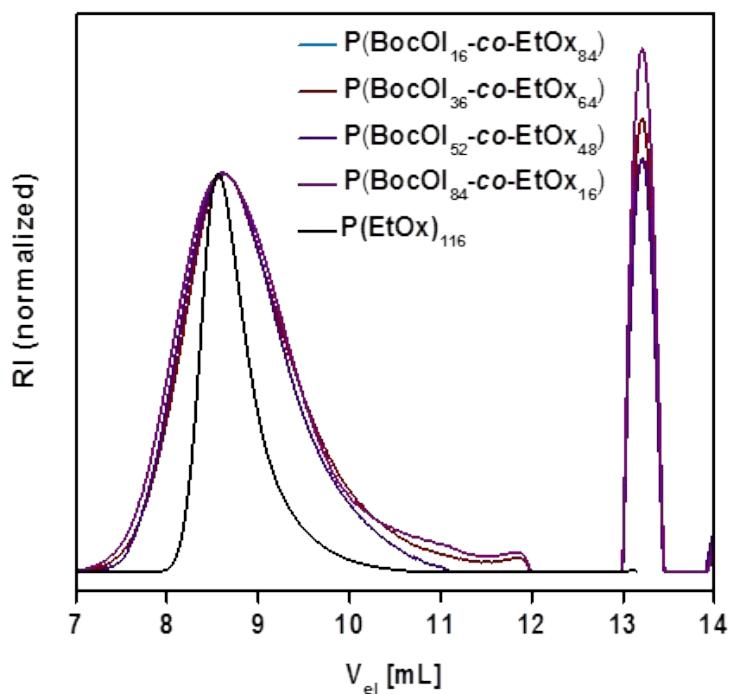
**Figure S23:** SEC-traces ( $\text{CHCl}_3$ -*i*-PrOH, PS-cal.; 1<sup>st</sup> system peak after 12 mL) of the purified Boc-protected copolymer precursors (**4a-d**).
