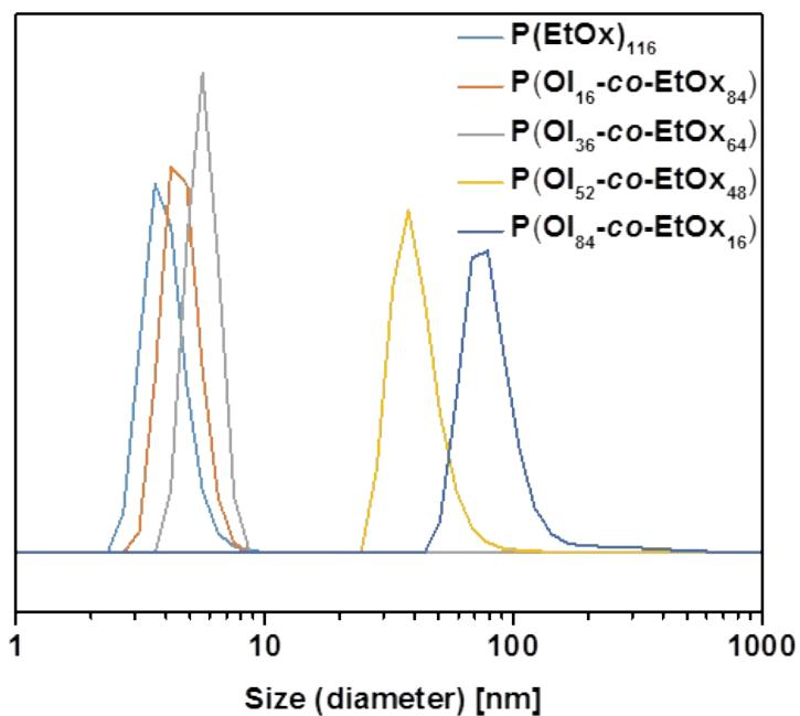
**Figure S30:** Size distribution of the self-assembled structures measured *via* DLS (number PSD).
