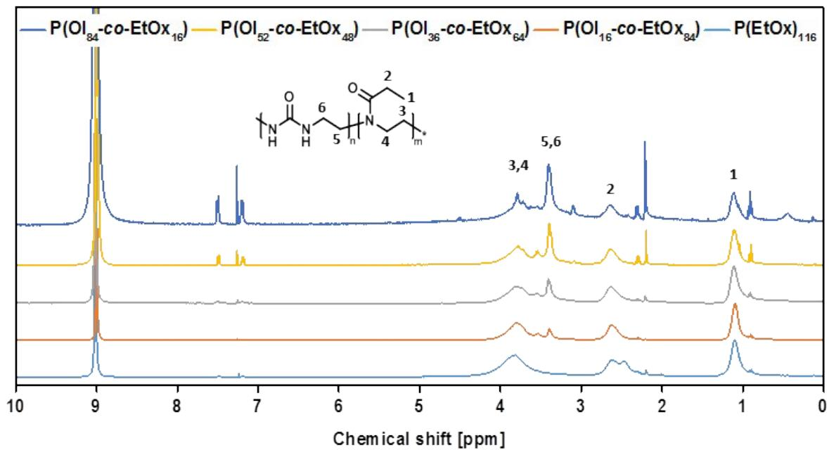
**Figure S22:**  $^1\text{H}$ -NMR (35% DCl in  $\text{D}_2\text{O}$ ,  $\text{CDCl}_3$ -standard, 300 MHz) of  $\text{P}(\text{OI}_n\text{-co-}\text{EtOx}_m)$  (**5a-d**) and  $\text{P}(\text{EtOx})_{116}$  (**6**).
