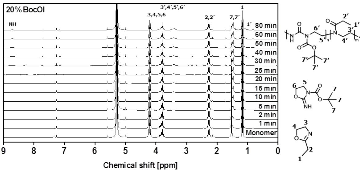
**Figure S16:** <sup>1</sup>H-NMR shifts ( $\text{CDCl}_3$ , 300 MHz) of time dependent P(BocOI-*co*-EtOx) kinetics in  $\text{CH}_2\text{Cl}_2$  at 100 °C with  $[\text{M}]/[\text{I}] = 60$  aiming 20% BocOI, recorded at RT.
