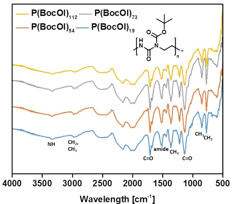
**Figure S11:** Normalized FTIR spectra of the purified  $P(BocOI)_n$  precursors (2a-d).
