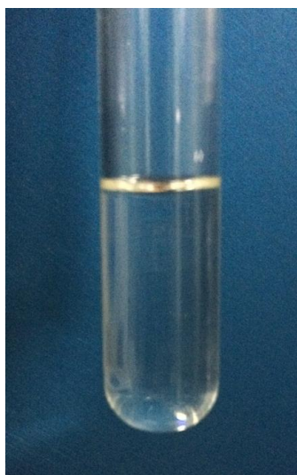
Fig. S1. Photograph of the homogeneous mixture of p -MeSt and IL.
