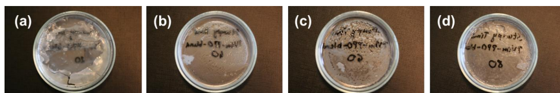
Figure S2. Photographs of poly( N -vinylimidazole) (PVIIm) and poly(propylene glycol) dimethacrylate (PPGDMA) homopolymer blends (PVIIm- blend -PPG) with different compositions: 20 wt% (a), 40 wt% (b), 60 wt% (c) and 80 wt% of PPG (d).
