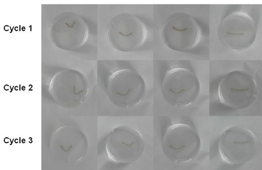
Fig. S6 Cycled shape memory performance of PBA-DA hydrogel in Gly aqueous solution (pH 6.0).
