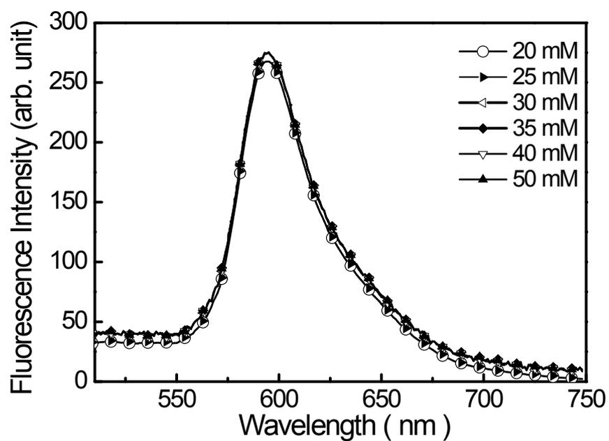
**Figure S8.** Changes in the fluorescence spectra of P1@GOx hydrogel (0.57 g) as a function of glucose concentrations (20 to 50 mM). Excitation wavelength,  $\lambda_{\text{ex}} = 490$  nm.
