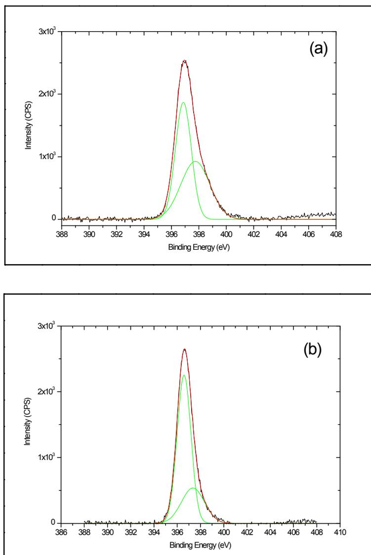
**Figure S1.** (A) FT-IR spectra of (a) GOx, (b) P1, (c) P2, and (d) P1@GOx. (B) XPS spectra of (a) P1 and (b) P2. Red and green curves indicate the fitted and deconvoluted ones, respectively.
