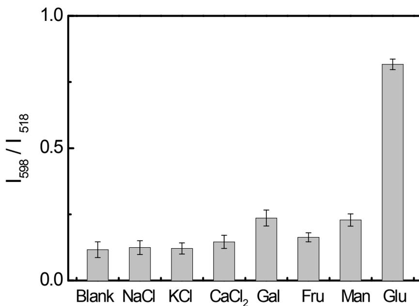
**Figure S6.** Selectivity of the **P1-GOx** hydrogel upon exposure to sodium chloride, potassium chloride, calcium chloride, galactose (Gal), fructose (Fru), mannose (Man) and glucose (Glu). [Monosaccharides] = 10 mM and [Electrolytes] = 10 mM.  $I_{598}$  and  $I_{518}$  correspond to the emission intensity of the **P1-GOx** hydrogel at 598 nm and 518 nm, respectively.
