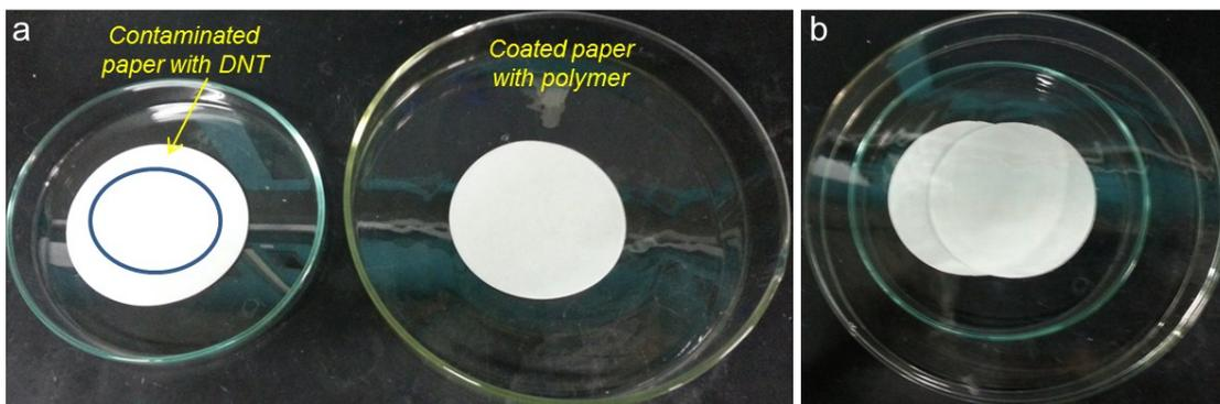
**Fig. S8** The demonstration for nitro compound vapors detection. (a) The bright image of filter paper contaminated by nitro compound (left). The right one is the substrate fabricated by spray coating polymer nanoparticles of **PTriPE** in THF/H<sub>2</sub>O (1:9 v/v) mixture onto filter paper, amounting to approximately concentration as 1.0  $\mu\text{g}/\text{cm}^2$ . (b) The demonstration for DNT vapor detection.
