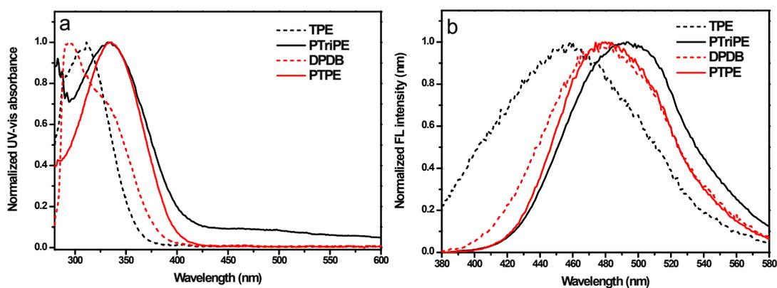
**Fig. S2** UV-Vis (a) and fluorescence spectra (b) of **TPE**, **DPDB**, **PTriPE** and **PTPE** in THF, THF/ $\text{H}_2\text{O}$  (1:9 v/v) mixture.
