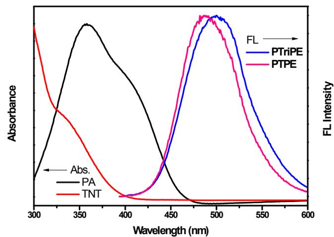
**Fig. S11** The normalized UV-vis absorption of PA and TNT, and normalized fluorescence of **PTriPE** and **PTPE** in THF/H<sub>2</sub>O (1:9 v/v).
