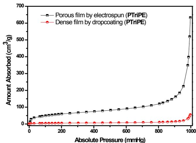
**Fig. S5**  $\text{N}_2$  absorption isotherms at  $-196 \text{ }^\circ\text{C}$  for **PTriPE** porous film by electrospun and **PTriPE** dense film by drop coating.
