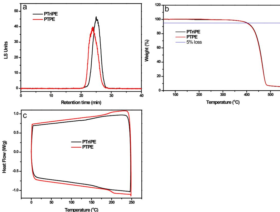
**Fig. S1** (a) GPC spectrum of polymers **PTriPE** and **PTPE** in THF. (b) TGA thermograms of polymers **PTriPE** and **PTPE** under nitrogen at a heating rate of  $20\text{ }^{\circ}\text{C}\cdot\text{min}^{-1}$ . (c) DSC thermograms of polymers **PTriPE** and **PTPE** under nitrogen at a heating rate of  $20\text{ }^{\circ}\text{C}\cdot\text{min}^{-1}$ .
