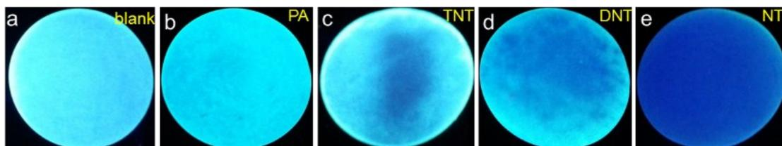
**Fig. S10** The fluorescence quenching of substrate on exposure to nitro compounds vapor, the fluorescent images of substrates are check by neck eyes after 30 min. (a) The image of substrate under UV light illumination (365 nm) without nitro compound. Figure b, c, d and e are the images of substrate under UV light illumination (365 nm) after contacting for PA, TNT, DNT and NT, respectively.
