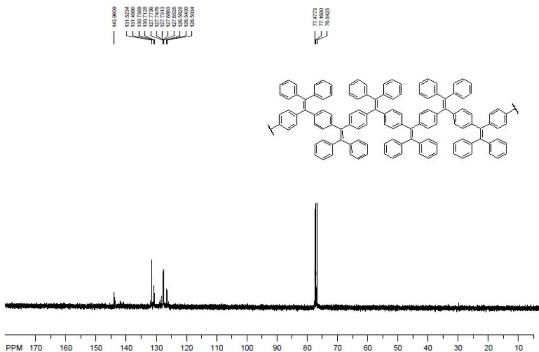
**Fig. S17**  $^{13}\text{C}$  NMR spectrum of PTriPE in  $\text{CDCl}_3$ .
