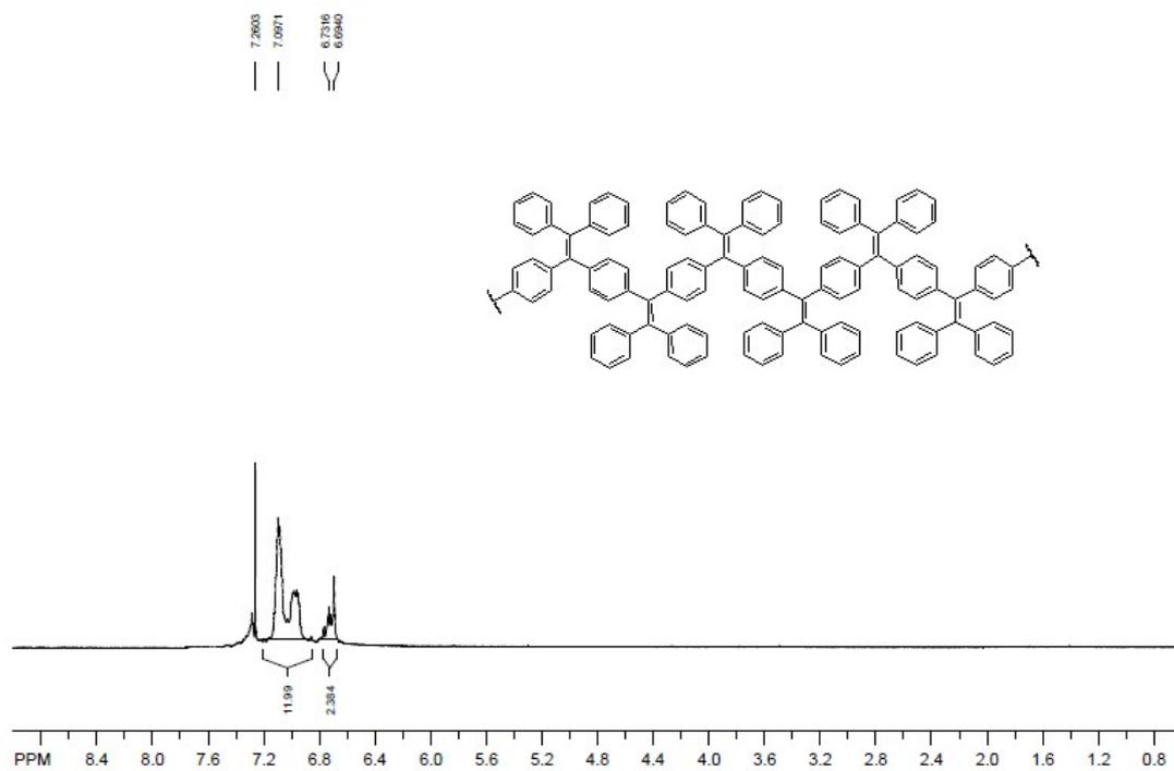
Fig. S16 <sup>1</sup>H NMR spectrum of PTriPE in CDCl<sub>3</sub>.
