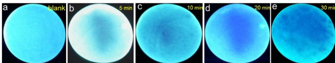
**Fig. S9** The fluorescence quenching of substrate on exposure to DNT saturated vapor for different time: (a) 0 min, (b) 5 min, (c) 10 min, (d) 20 min, (e) 30 min. The images of substrate are under UV light illumination (365 nm).
