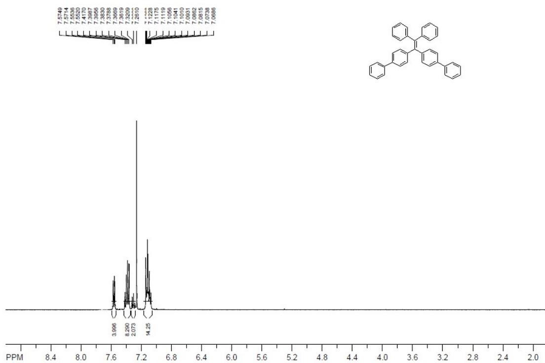
**Fig. S12** <sup>1</sup>H NMR spectrum of **DPDB** in CDCl<sub>3</sub>.
