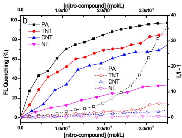
**Fig. S4** Concentration-dependent fluorescence quenching of **PTPE** by nitro compounds.  $[\text{PTPE}] = 100.0 \mu\text{g}\cdot\text{mL}^{-1}$  in THF/ $\text{H}_2\text{O}$  (1:9 v/v) mixture.
