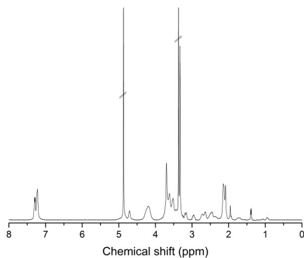
**Fig. S20** <sup>1</sup>H NMR (400 MHz, MeOD) of **P2c**: **P2** (poly(oligo(MeOx-*alt*-AA)<sub>2.5</sub>A)<sub>10</sub>) functionalised with phenylalanine methyl ester.
