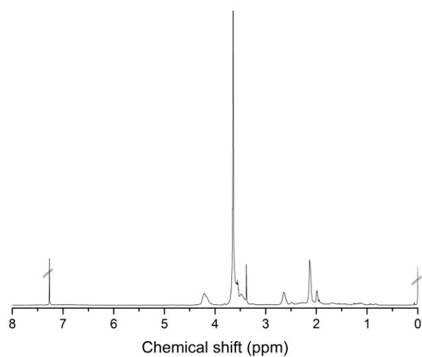
**Fig. S17** <sup>1</sup>H NMR (400 MHz, CDCl<sub>3</sub>) of **P1b: P1** (poly(oligo(MeOx-*alt*-AA)<sub>3</sub>A)<sub>10</sub>) functionalised with PEG-amine.
