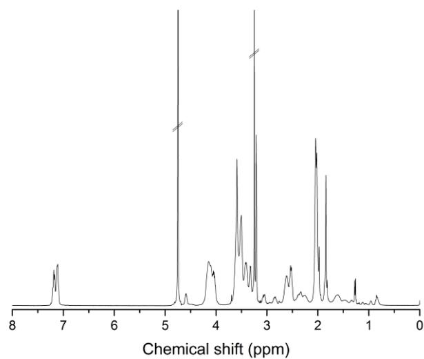
**Fig. S18** <sup>1</sup>H NMR (400 MHz, MeOD) of **P1c: P1** (poly(oligo(MeOx-*alt*-AA)<sub>3</sub>A)<sub>10</sub>) functionalised with phenylalanine methyl ester.
