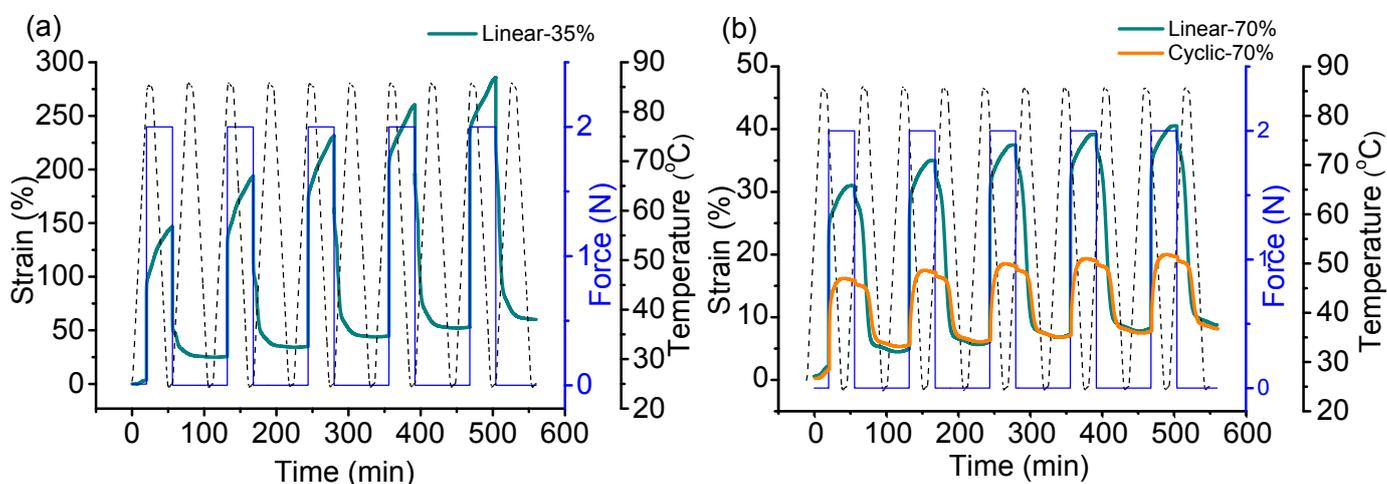
**Figure S12.** (a) Shape memory experiment for **Linear-35%** and (b) **Cyclic-70%** and **Linear-70%** showing five cycles. The material was heated to 85 °C, and a force of 2 N was applied to stretch the sample. The sample was then cooled to 25 °C. The force was removed, and the degree of fixing was measured. The
