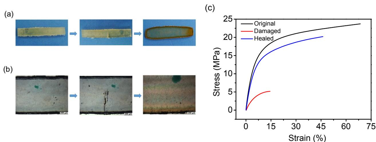
**Figure S17.** The thermally active self-healing process of a crack in **Cyclic-70%** and mechanical properties. (a) Digital photos of **Cyclic-70%**. (b) Optical micrographs of **Cyclic-70%**. (c) Stress-strain curve for representative original (black curve), damaged (red curve), and healed (blue curve) samples of **Cyclic-70%**. Tensile tests were executed by DMA in the Controlled Force Stress-Strain mode and conducted at a rate of 1 N/min to 18 N.
