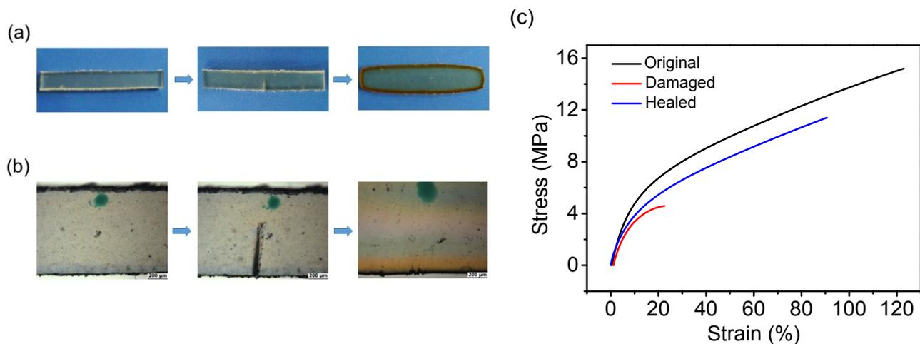
**Figure S16.** The thermally active self-healing process of a crack in **Linear-70%** and mechanical properties. (a) Digital photos of **Linear-70%**. (b) Optical micrographs of **Linear-70%**. (c) Stress-strain curve for representative original (black curve), damaged (red curve), and healed (blue curve) samples of **Linear-70%**. Tensile tests were executed by DMA in the Controlled Force Stress-Strain mode and conducted at a rate of 1 N/min to 18 N.
