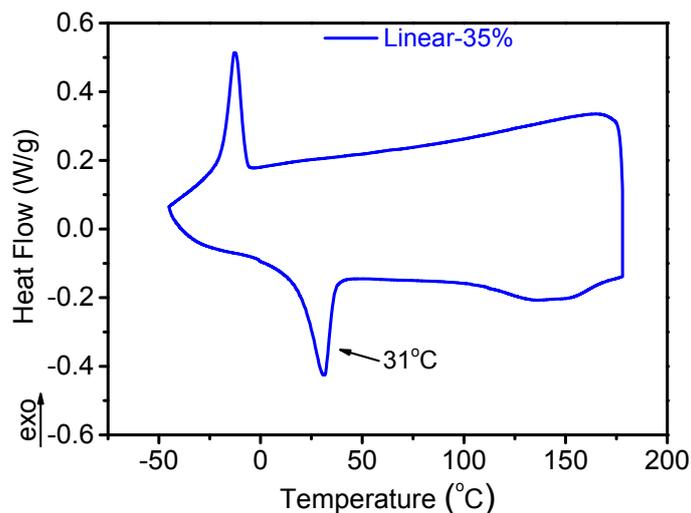
**Figure S8.** DSC thermograms of **Linear-35%**. The heating rate was 10 °C /min from -50 °C to 180 °C under a N<sub>2</sub> atmosphere.
