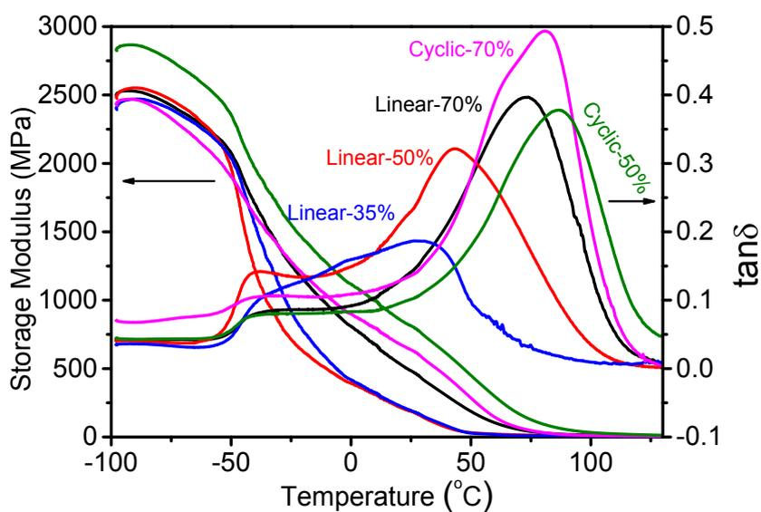
**Figure S10.** DMA curves of PUs. The heating rate was 3 °C/min from -100 °C to 130 °C.
