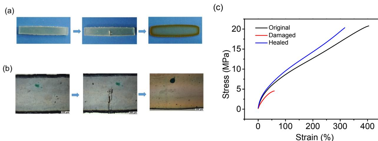
**Figure S15.** The thermally active self-healing process of a crack in **Linear-50%** and mechanical properties. (a) Digital photos of **Linear-50%**. (b) Optical micrographs of **Linear-50%**. (c) Stress-strain curve for representative original (black curve), damaged (red curve), and healed (blue curve) samples of **Linear-50%**. Tensile tests were executed by DMA in the Controlled Force Stress-Strain mode and conducted at a rate of 1 N/min to 18 N.
