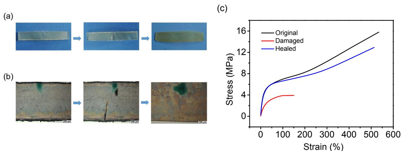
**Figure S14.** The thermally active self-healing process of a crack in **Linear-35%** and mechanical properties. (a) Digital photos of **Linear-35%**. (b) Optical micrographs of **Linear-35%**. (c) Stress-strain curve for representative original (black curve), damaged (red curve), and healed (blue curve) samples of **Linear-35%**. Tensile tests were executed by DMA in the Controlled Force Stress-Strain mode and conducted at a rate of 1 N/min to 18 N.
