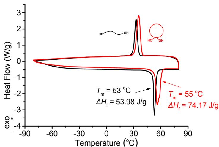
**Figure S7.** DSC thermograms of *l*-PCL-2OH and *c*-PCL-2OH. The heating rate was 10 °C /min from -80 °C to 80 °C under a nitrogen flow.
