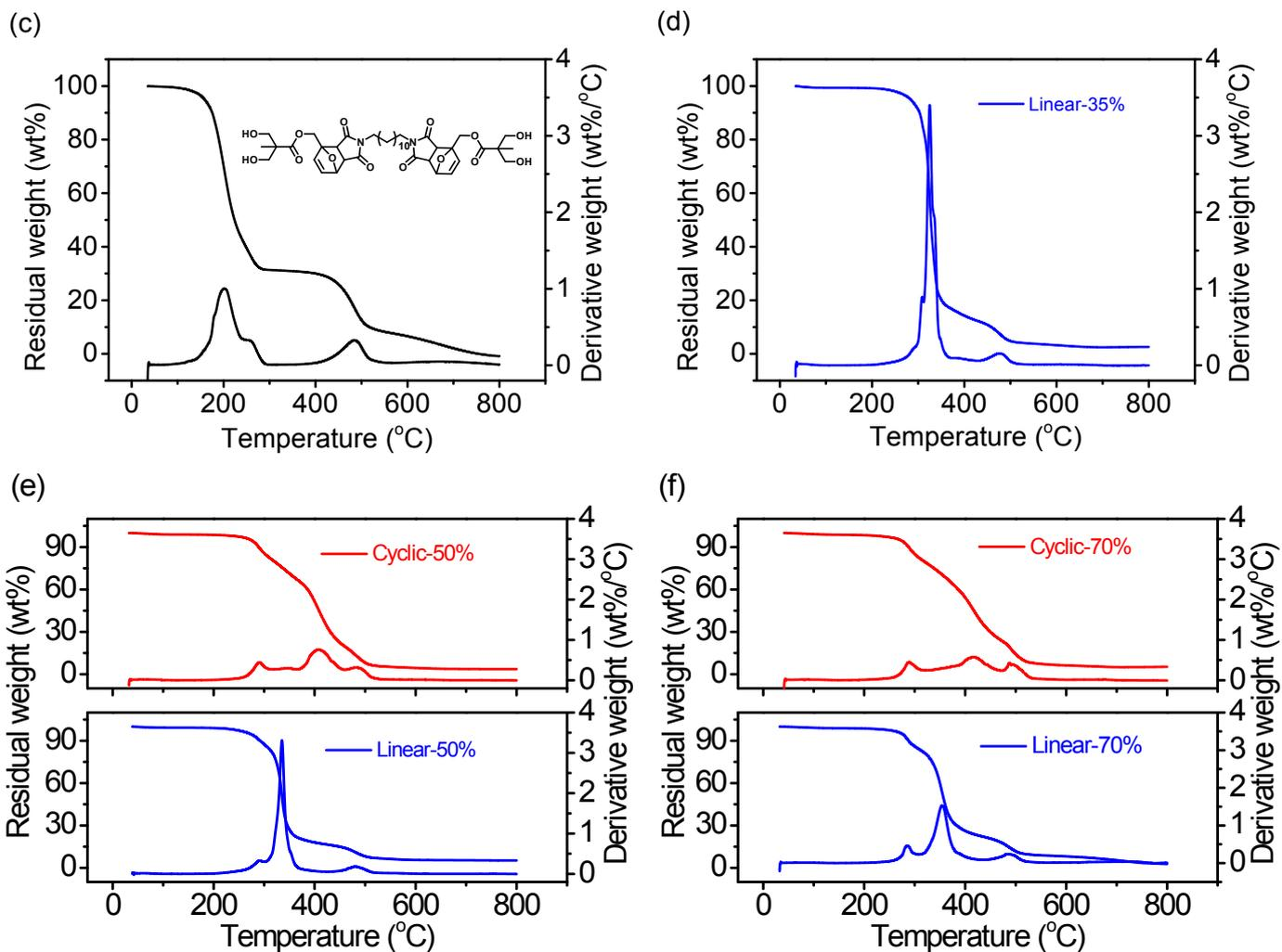
**Figure S9.** (a) TGA curves of *l*-PCL-2OH, (b) *c*-PCL-2OH, (c) FM and (d,e,f) PUs. The heating rate was 10 °C /min from room temperature to 800 °C under a N<sub>2</sub> atmosphere.
