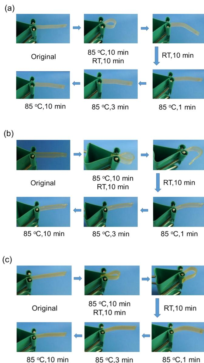
**Figure S11.** Pictures showing the shape memory properties of (a) **Linear-35%**, (b) **Linear-70%** and (c) **Cyclic-70%**.
