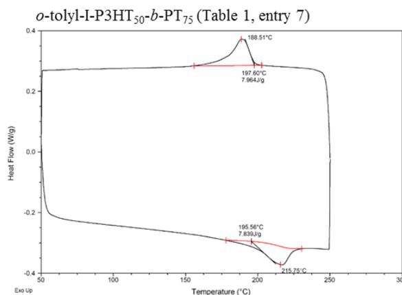
1<sup>st</sup> cycle for crystallization and 2<sup>nd</sup> cycle for melting
