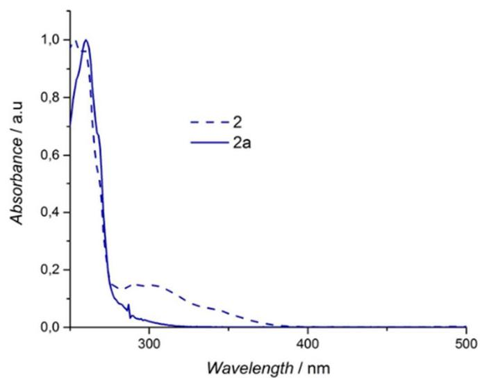
**Figure S4.** UV-Vis spectra of **2** before (dashed line) and after (dashed line, **2a**) end group capping with 2-methoxy-6-methylbenzaldehyde.
