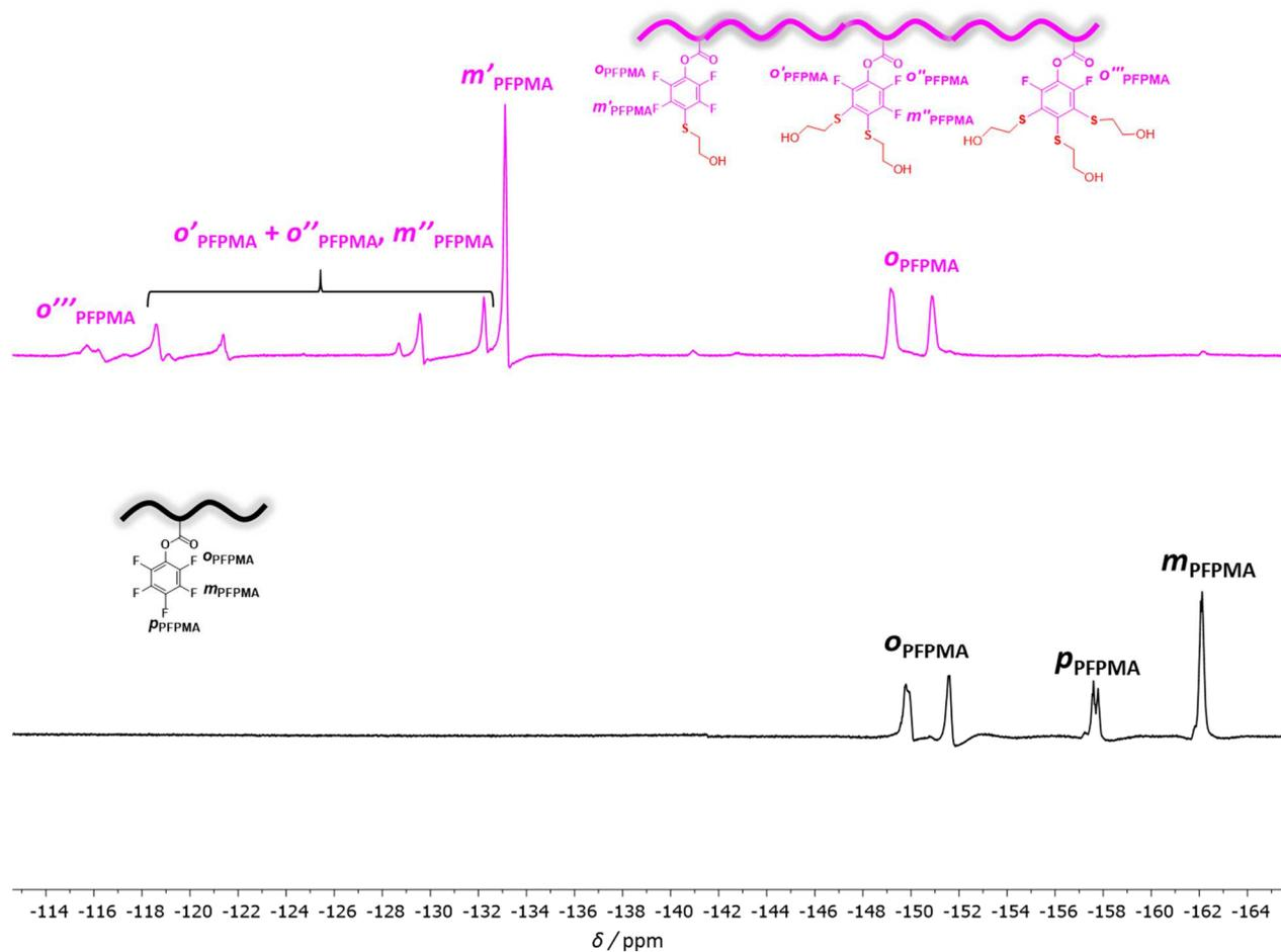
**Figure 13.**  $^{19}\text{F}$  NMR of **1a** before (bottom) and after (top) reaction with 5 eq. mercaptoethanol under PFTR standard conditions.
