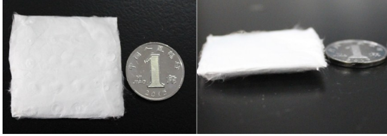
Figure S3 Images of polystyrene electrospun mat collected on our cooled collector with array of icy balls. The diameter of the coin (ten cent CNY) is 19.5 mm and the thickness is 16.7 mm.
