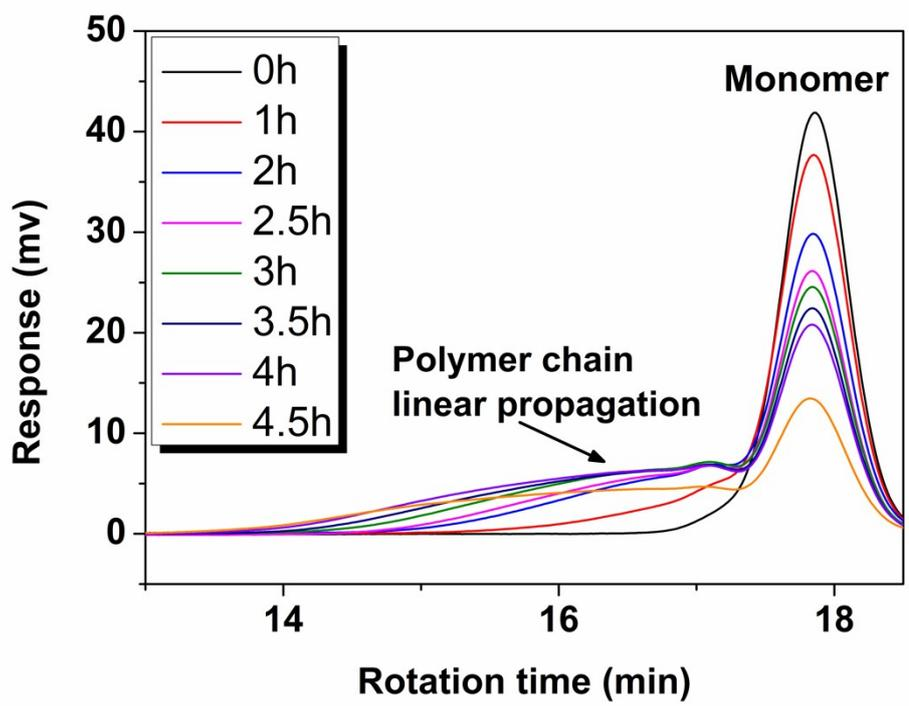
Figure S1 GPC traces of *in situ* DE-ATRP of PEGDA<sub>700</sub>.
