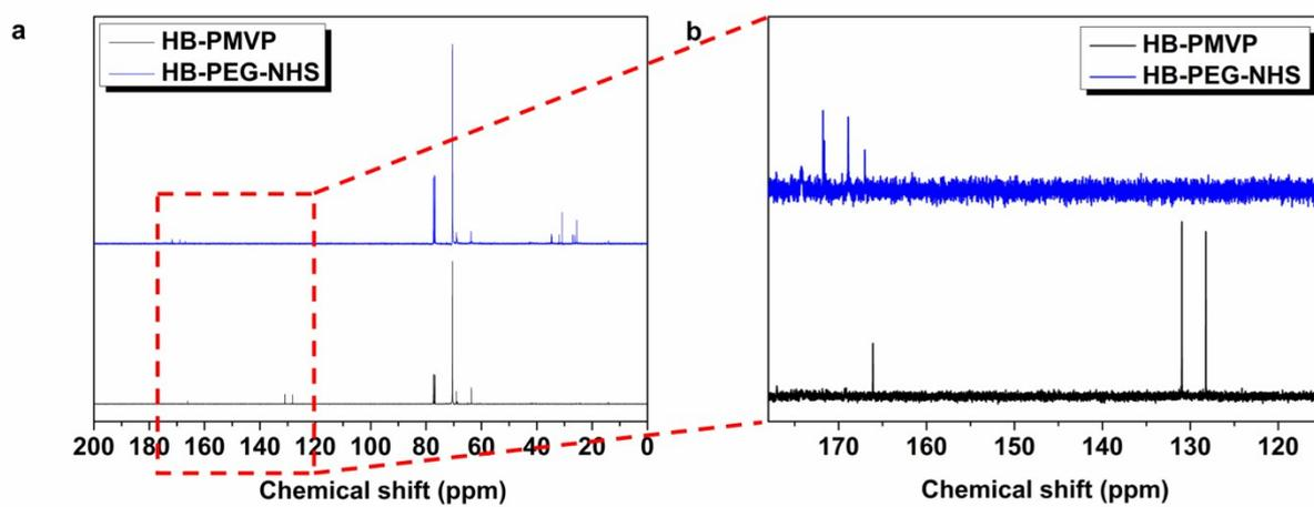
**Figure S6**  $^{13}\text{C}$ -NMR results of HB-PMVP (black) and HB-PEG-NHS (blue). (a) Full spectrum of  $^{13}\text{C}$ -NMR results. (b) Zoom in area of (a) from 115 ppm to 178 ppm.
