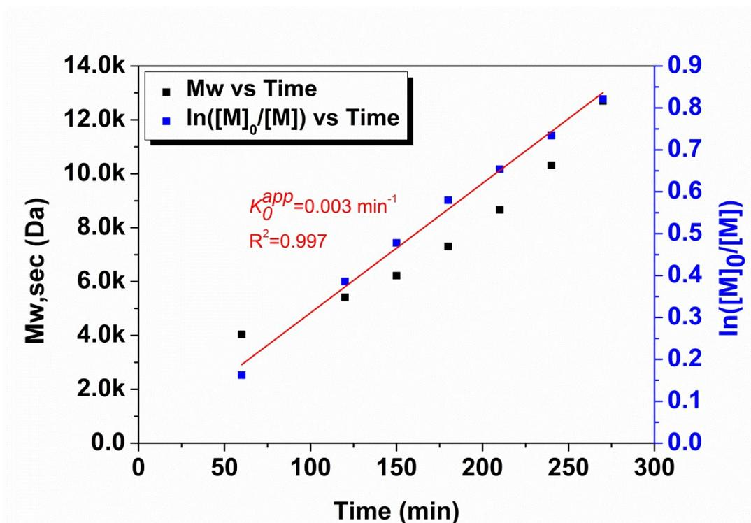
**Figure S3** Kinetic plot of *in situ* DE-ATRP PEGDA<sub>700</sub> (Mw versus time and ln([M]<sub>0</sub>/[M]) versus time).
