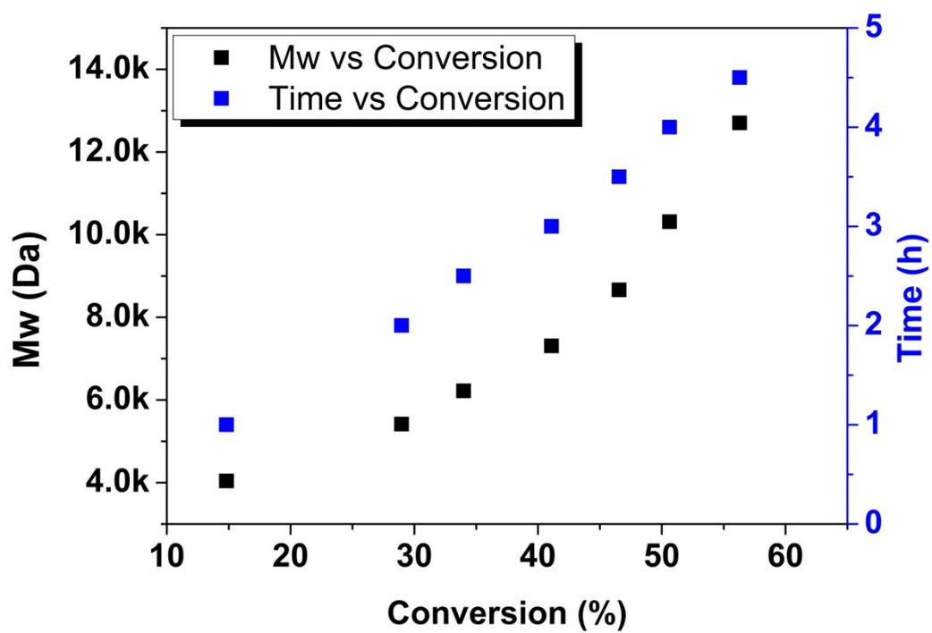
Figure S2 Kinetic plot of *in situ* DE-ATRP PEGDA<sub>700</sub> (Mw versus conversion and time versus conversion).
