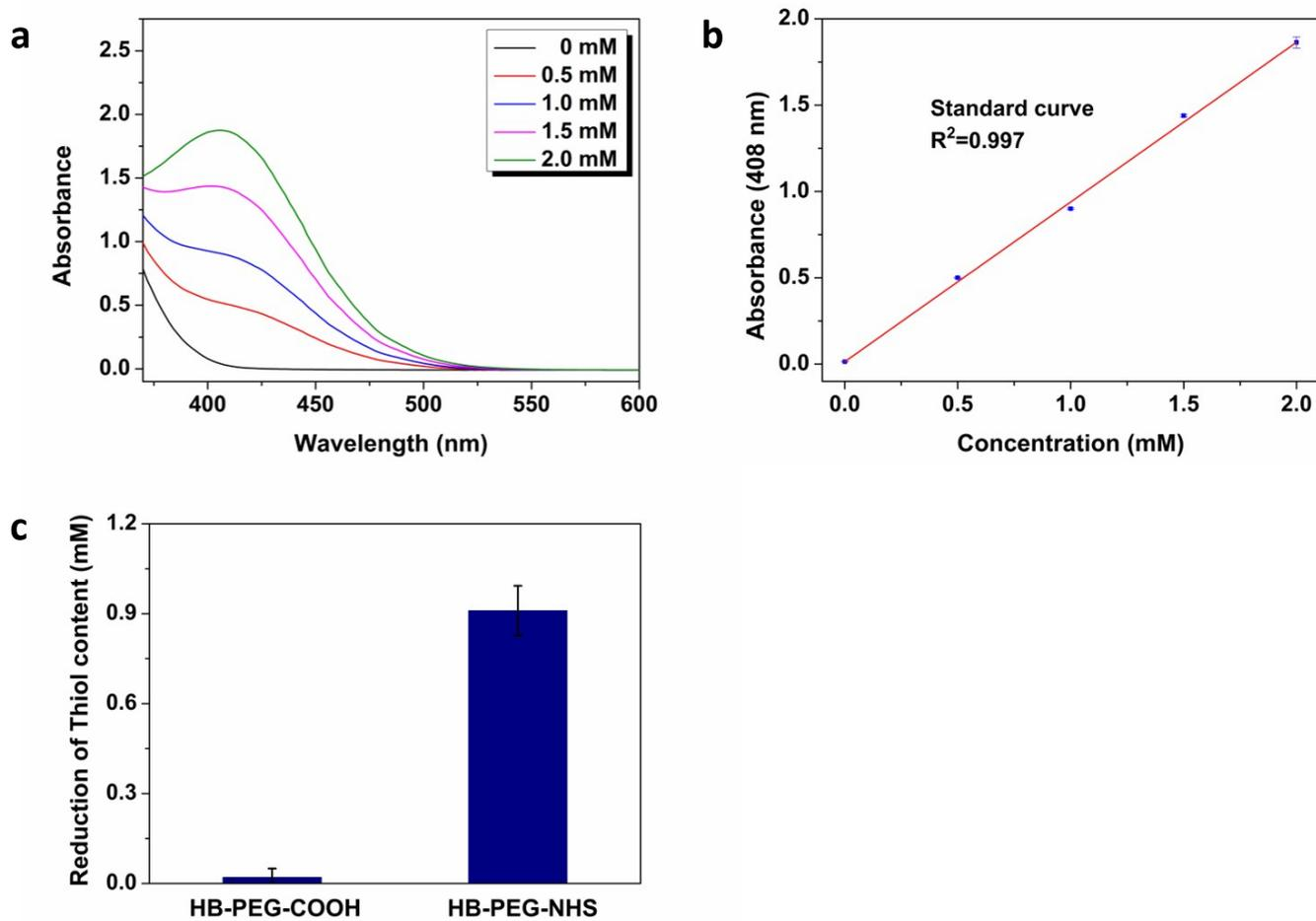
**Figure S7** (a) Absorbance of the standard samples. (b) Fitted standard curve of absorbance at 408 nm. (c) NHS content determination by Ellman method.
