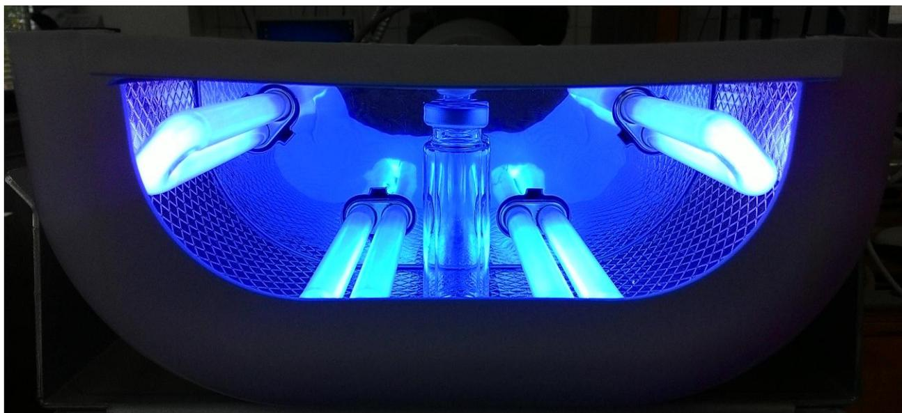
Figure SF3. Setup for surface-initiated photoinduced SET-LRP.
