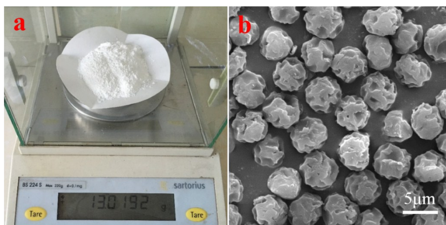
Fig. S2 Large-scale preparation of irregular microparticles by ultrasound swelling for 10 min with the ratio of DBP/S was 1.5/1.5.
