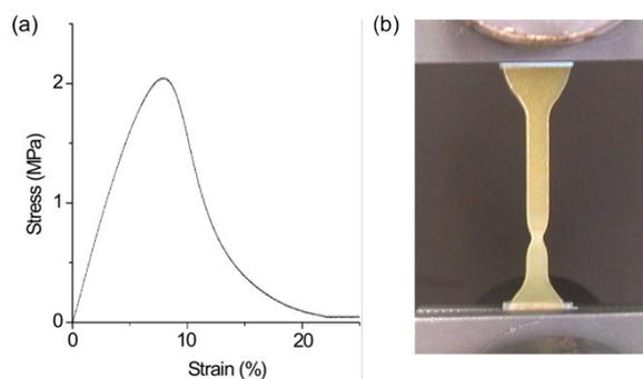
Figure S12. (a) Stress-strain curve obtained for compound **6** and (b) macroscopic image of the sample during the measurement.
