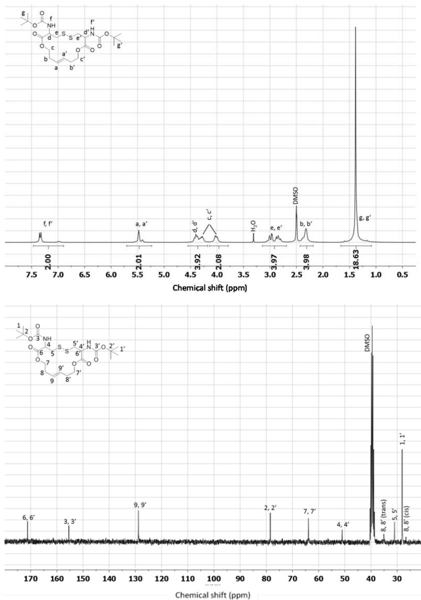
**Figure S3.**  $^1\text{H}$  NMR spectrum (300 MHz, DMSO- $d_6$ ) (top) and  $^{13}\text{C}$  NMR spectrum (75 MHz, DMSO- $d_6$ ) (bottom) of **3a**.
