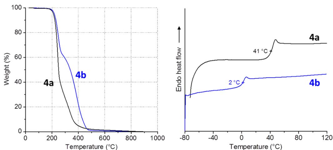
**Figure S13.** TGA (left) and DSC (right) curves of polymers **4a** and **4b**. Thermal decomposition proceeds in two steps at 160-170 °C (decomposition of Boc protecting group) and >260 °C (decomposition of polymer backbone). Glass transitions occurred at 41 °C (**4a**) and 2 °C (**4b**).
