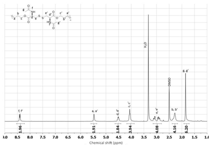
**Figure S19.**  $^1\text{H}$  NMR spectrum (300 MHz, DMSO- $d_6$ ) of functionalized polymer **6a**.
