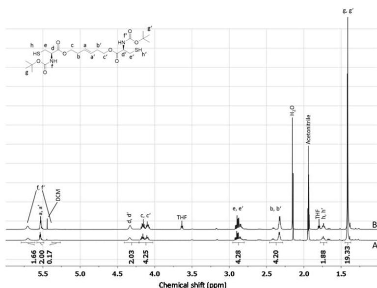
**Figure S21.** <sup>1</sup>H NMR spectra (600 MHz, CD<sub>3</sub>CN) of the products obtained by disulfide reduction of polymer **4a** (A) and macrocycle **3a** (B).
