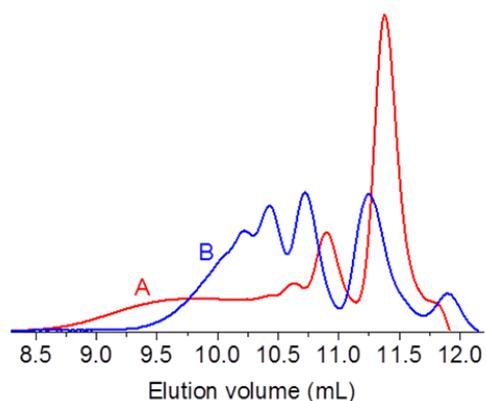
**Figure S8.** SEC-RI traces (eluent: THF) of the crude products obtained by ADMET polymerizations **A** and **B**, revealing the presence of just low molar mass and cyclic products.
