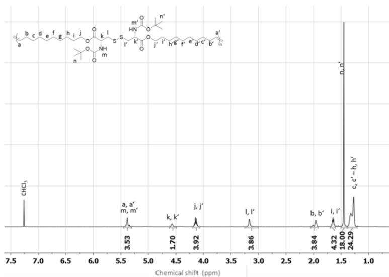
**Figure S10.**  $^1\text{H}$  NMR spectrum (600 MHz,  $\text{CDCl}_3$ ) of polymer **4b**.
