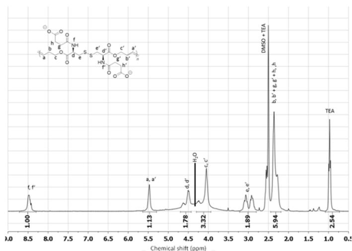
**Figure S20.**  $^1\text{H}$  NMR spectrum (300 MHz, DMSO- $d_6$ ) of functionalized polymer **7a**.
