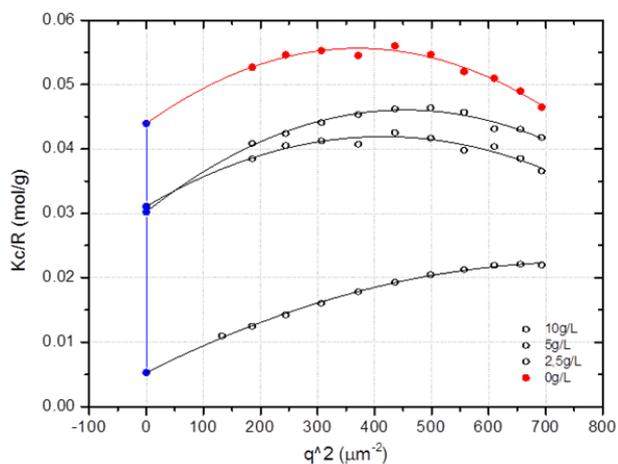
**Figure S12.** Concentration- and angle-dependent SLS data for polymer **4a** in ethyl acetate at room temperature ( $dn/dc = 0.128 \text{ mL/g}$ ).
