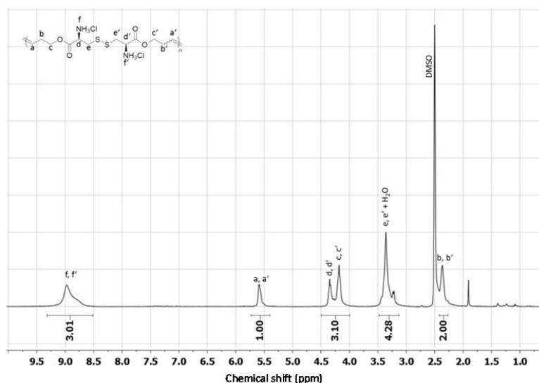
**Figure S14.**  $^1\text{H}$  NMR spectrum (300 MHz,  $\text{DMSO-d}_6$ ) of deprotected polymer **5a**.
