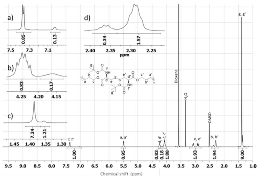
**Figure S9.** <sup>1</sup>H NMR (600 MHz, DMSO-d<sub>6</sub>) of polymer **4a**. Expanded regions show two signals for the a) NH urethane (*f*, *f'*) b) α-CH (*d*, *d'*) and c) *tert*-butyl group (*g*, *g'*) due to the hindered rotation of the Boc group; d) two signals of -CH<sub>2</sub>-C= (*b*, *b'*) arise from the *cis* and *trans* isomers of the double bond.
