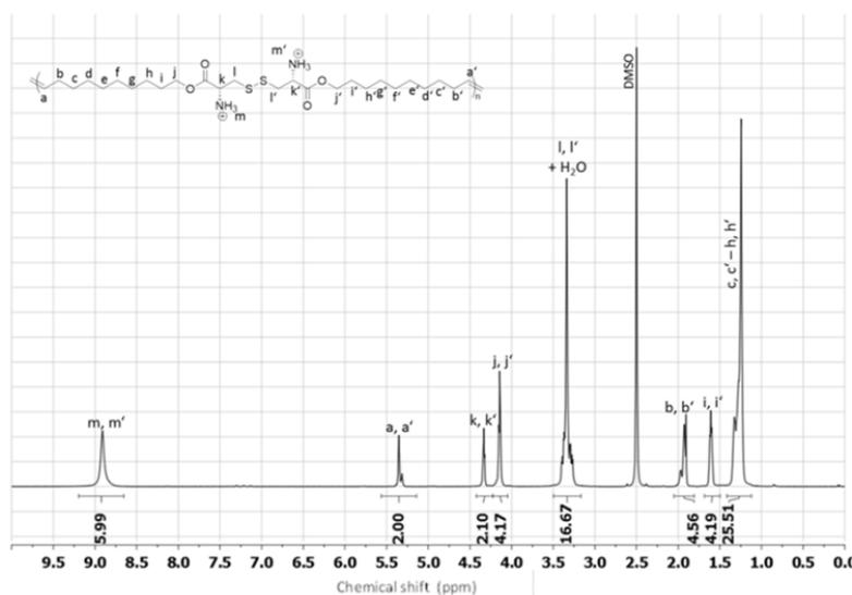
**Figure S16.**  $^1\text{H}$  NMR spectrum (600 MHz,  $\text{DMSO-d}_6$ ) of deprotected polymer **5b**.
