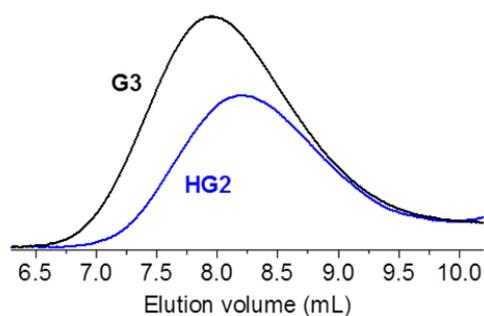
**Figure S11.** SEC-RI traces (eluent: THF) of the polymer products obtained by polymerization of **3a** with catalysts G3 ( $\rightarrow$  **4a**, monomer conversion: 80%) and HG2 (70%). Polymerizations were performed applying the same reaction conditions (see above).
