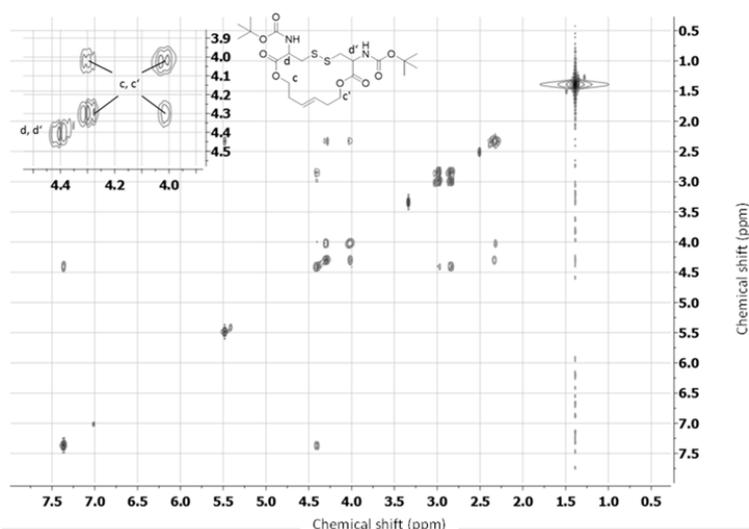
**Figure S4.** 2D [ $^1\text{H}$ ,  $^1\text{H}$ ] COSY NMR spectrum (300 MHz,  $\text{DMSO-d}_6$ ) of **3a**. Inset shows the expanded region between 3.8 and 4.6 ppm revealing the geminal coupling of  $-\text{OCH}_2-$  groups.
