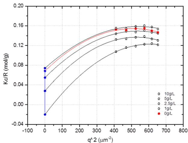
**Figure S15.** Concentration- and angle-dependent SLS data for polymer **5a** in water at room temperature ( $dn/dc = 0.184 \text{ mL/g}$ ).
