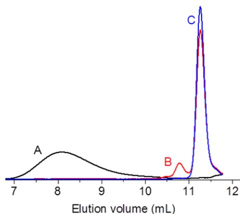
**Figure S22.** SEC-RI traces (eluent: THF) of the polymer **4a** (A) and the degradation products obtained by reduction of main-chain disulfide after reaction time of 10 minutes (B) and 30 minutes (C).
