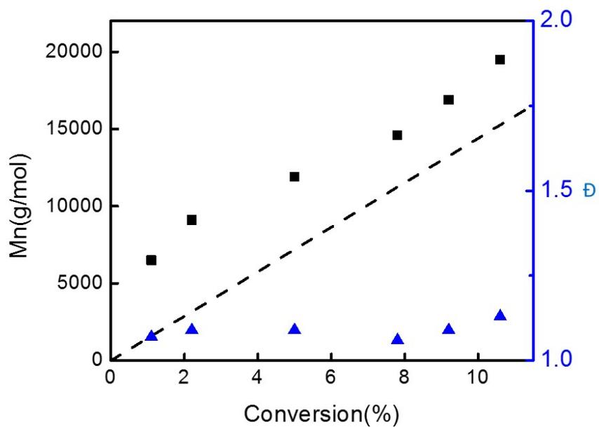
Figure S3. Molecular weight versus conversion and polydispersity for surface-initiated polymerization of BzMA from SiO<sub>2</sub>-g-(PHPMA, CPDB) NPs at 70°C in ethanol.
