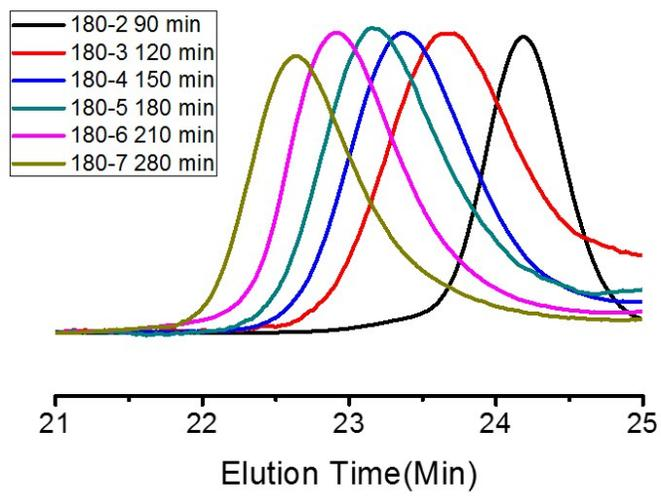
Figure S4. THF gel permeation chromatograms (vs poly (methyl methacrylate) standards) obtained from PBzMA chains cleaved-off from  $\text{SiO}_2$ -g-(PHPMA, PBzMA) NPs.
