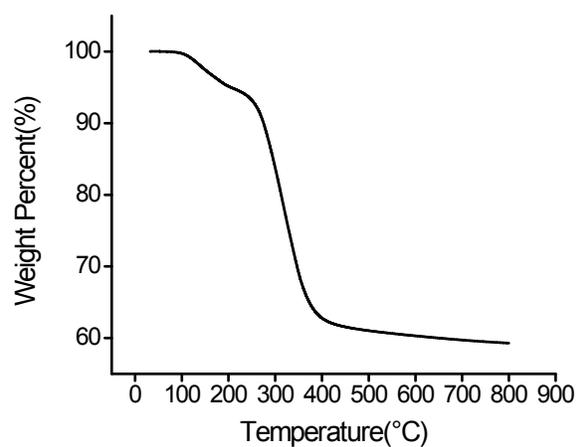
Figure S1. Thermal gravimetric analysis of SiO<sub>2</sub>-g-(PHPMA, CPDB) NPs.
