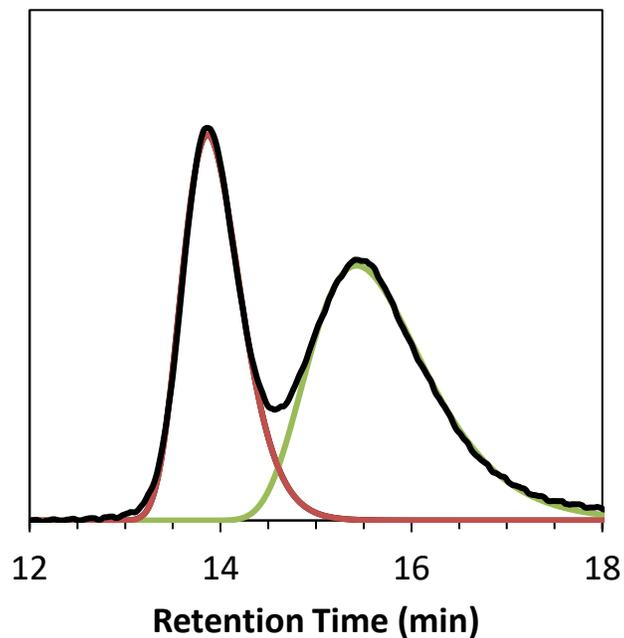
**Figure S4:** SEC trace and peak fit of bottlebrush polymer from Table 1, entry 2. The black trace is the raw RI signal obtained via SEC. Red and green traces represent fits of bottlebrush and linear polymer populations, respectively.
