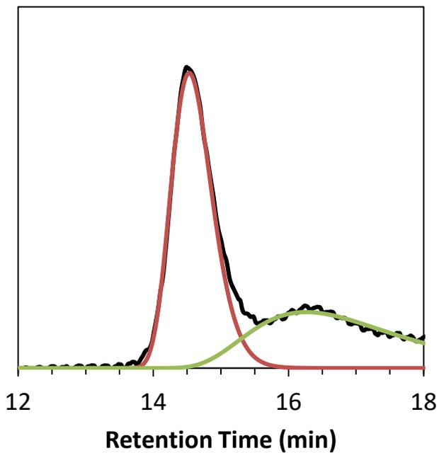
**Figure S3:** SEC trace and peak fit of bottlebrush polymer from Table 1, entry 1. The black trace is the raw RI signal obtained via SEC. Red and green traces represent fits of bottlebrush and linear polymer populations, respectively.
