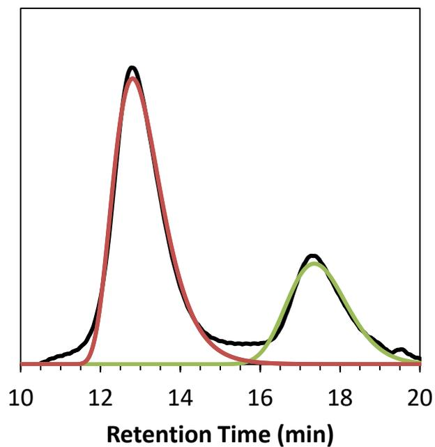
**Figure S11:** SEC trace and peak fit of bottlebrush polymer from Table 1, entry 9. The black trace is the raw RI signal obtained via SEC. Red and green traces represent fits of bottlebrush and linear polymer populations, respectively.
