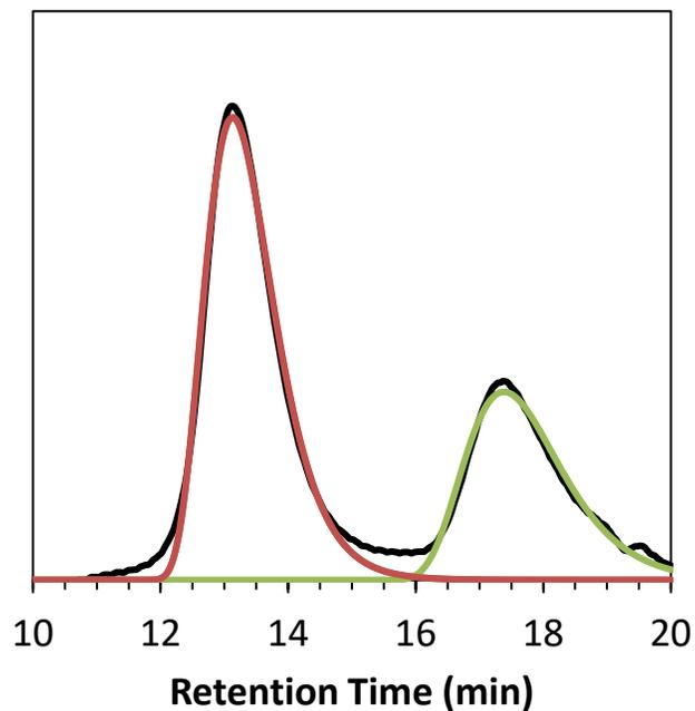
**Figure S10:** SEC trace and peak fit of bottlebrush polymer from Table 1, entry 8. The black trace is the raw RI signal obtained via SEC. Red and green traces represent fits of bottlebrush and linear polymer populations, respectively.
