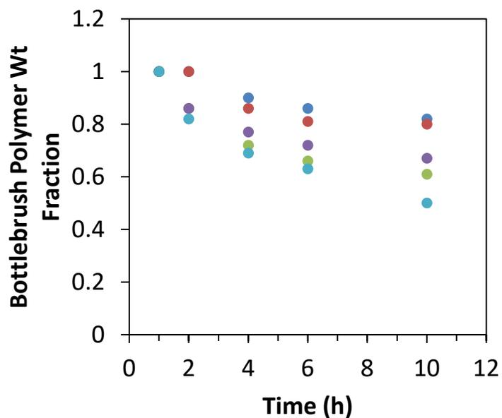
**Figure S19.** Change in bottlebrush polymer weight fraction over time for polymerizations conducted with PCTA DP = 50 (dark blue circles), 100 (purple circles), 500 (green circles), 750 (red circles), and 1000 (light blue circles).
