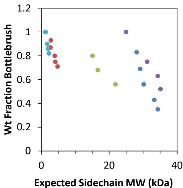
**Figure S17.** Relationship between expected sidechain molecular weight, calculated using the equation  $MW_{sidechains} = conv * \frac{[M]}{[CTA]} * MW_{styrene}$ , and the bottlebrush polymer sample composition based on area under the curves of the SEC traces at each time point for polymerizations conducted with  $[M]/[CTA] = 1000$  (dark blue circles), 750 (purple circles), 500 (green circles), 100 (red circles), and 50 (light blue circles).
