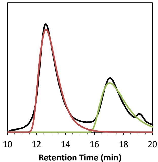
**Figure S12:** SEC trace and peak fit of bottlebrush polymer from Table 1, entry 10. The black trace is the raw RI signal obtained via SEC. Red and green traces represent fits of bottlebrush and linear polymer populations, respectively.
