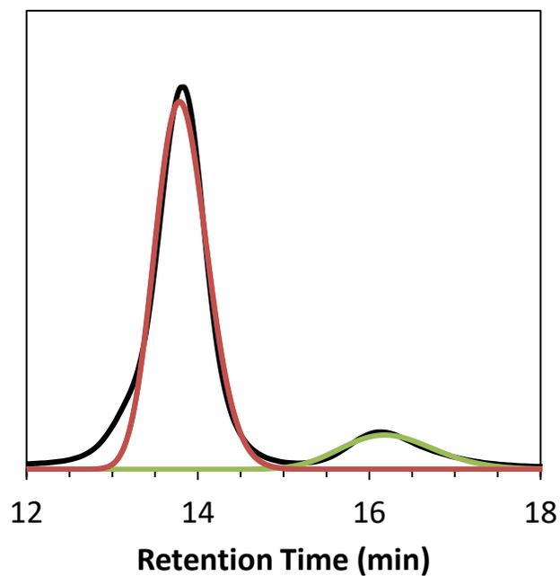
**Figure S13:** SEC trace and peak fit of bottlebrush polymer from Table 1, entry 11. The black trace is the raw RI signal obtained via SEC. Red and green traces represent fits of bottlebrush and linear polymer populations, respectively.
