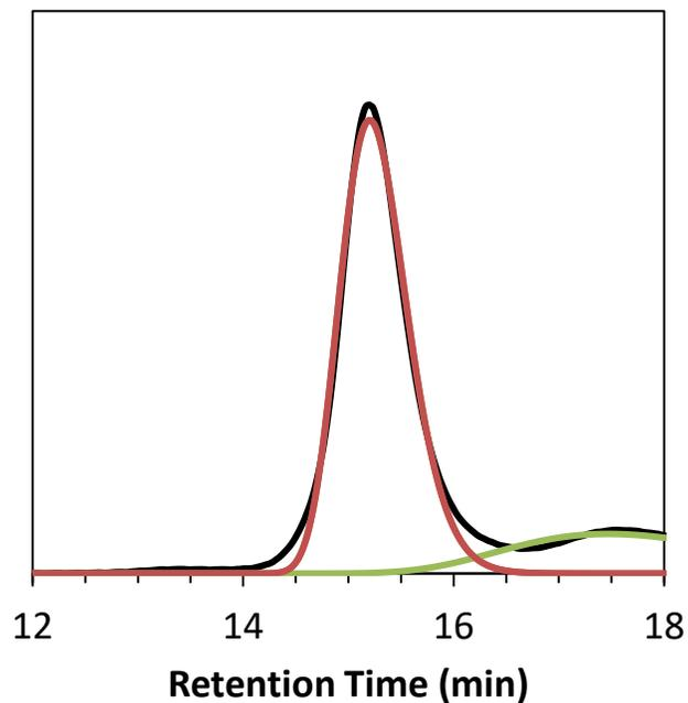
**Figure S8:** SEC trace and peak fit of bottlebrush polymer from Table 1, entry 6. The black trace is the raw RI signal obtained via SEC. Red and green traces represent fits of bottlebrush and linear polymer populations, respectively.
