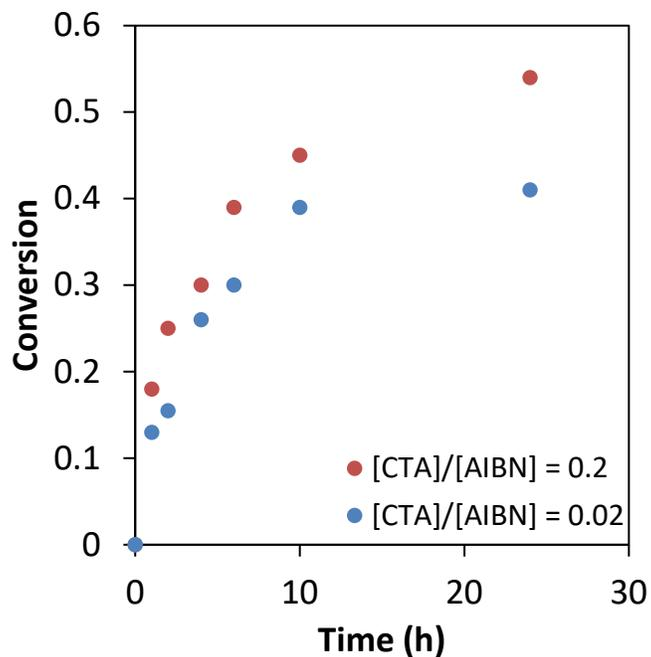
**Figure S15.** Kinetics of RAFT transfer-to polymerization of styrene with different amounts of radical initiator. Polymerizations were conducted at  $[M]/[CTA] = 1000$  with different equivalents of AIBN relative to CTA.
