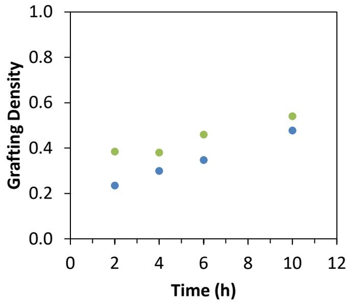
**Figure S22.** Comparison of bottlebrush polymer grafting density calculated by dividing the observed MW of the bottlebrush polymer by sidechain MWs calculated from monomer conversions obtained via  $^1\text{H}$  NMR spectroscopy (green circles) and measured for cleaved sidechains (blue circles) for the polymerization with  $[\text{M}]/[\text{CTA}] = 50$  and a backbone DP of 50.
