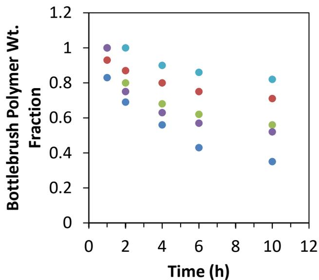
**Figure S16.** Change in bottlebrush weight fraction over time for polymerizations conducted with  $[M]/[CTA] = 1000$  (dark blue circles), 750 (purple circles), 500 (green circles), 100 (red circles), and 50 (light blue circles).
