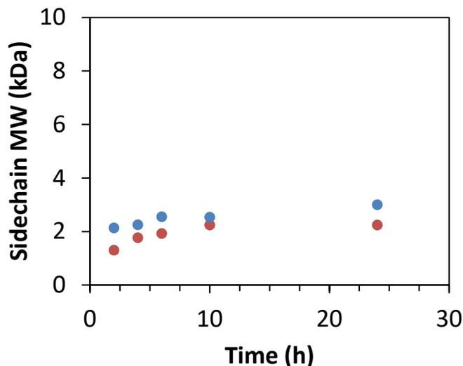
**Figure S21.** Comparison of bottlebrush polymer sidechain MWs calculated from monomer conversions obtained via <sup>1</sup>H NMR spectroscopy (red circles) and measured for cleaved sidechains (blue circles) for the polymerization with [M]/[CTA] = 50 and a backbone DP of 50. Sidechains MWs were calculated using the equation  $MW_{sidechains} = conv * \frac{[M]}{[CTA]} * MW_{styrene}$ .
