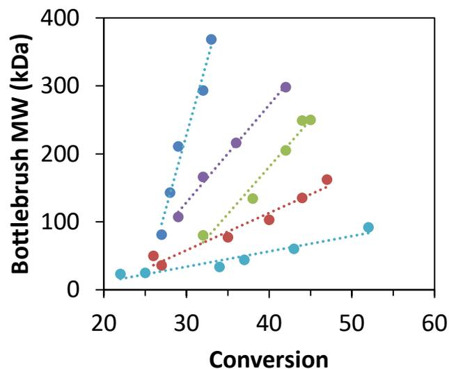
**Figure S18.** MW vs conversion for polymerizations conducted with conducted with  $[M]/[CTA] = 1000$  (dark blue circles), 750 (purple circles), 500 (green circles), 100 (red circles), and 50 (light blue circles). Linear fit lines have been provided as a visual aid.
