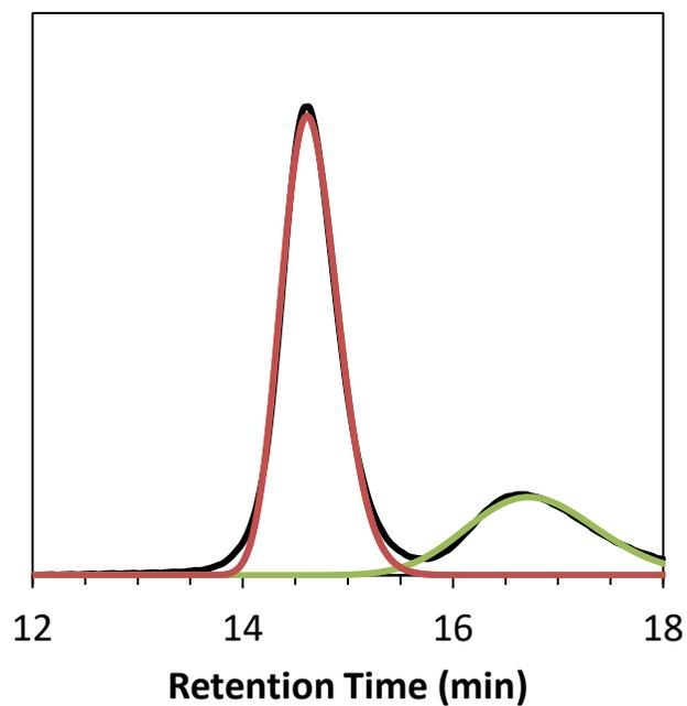
**Figure S7:** SEC trace and peak fit of bottlebrush polymer from Table 1, entry 5. The black trace is the raw RI signal obtained via SEC. Red and green traces represent fits of bottlebrush and linear polymer populations, respectively.
