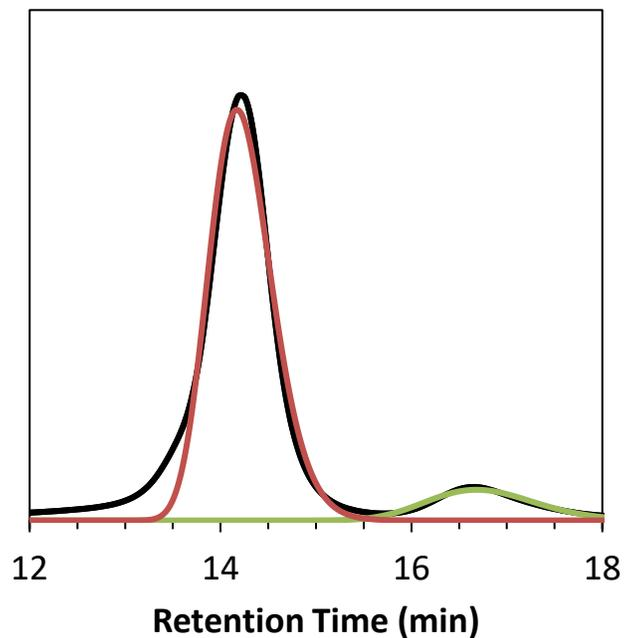
**Figure S14:** SEC trace and peak fit of bottlebrush polymer from Table 1, entry 12. The black trace is the raw RI signal obtained via SEC. Red and green traces represent fits of bottlebrush and linear polymer populations, respectively.
