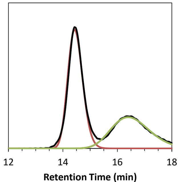
**Figure S6:** SEC trace and peak fit of bottlebrush polymer from Table 1, entry 4. The black trace is the raw RI signal obtained via SEC. Red and green traces represent fits of bottlebrush and linear polymer populations, respectively.
