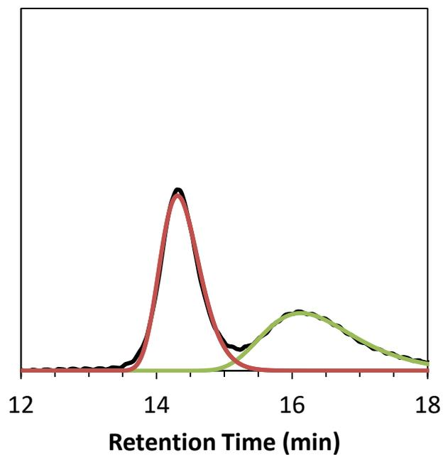
**Figure S5:** SEC trace and peak fit of bottlebrush polymer from Table 1, entry 3. The black trace is the raw RI signal obtained via SEC. Red and green traces represent fits of bottlebrush and linear polymer populations, respectively.
