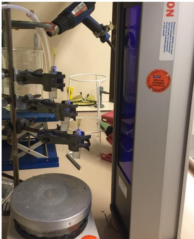
*Figure S21: Set-up photo-initiation for both, distance and time-dependent reactions. Samples were exposed vertically to the blacklight Vilber Lourmat VL-215.L.*
