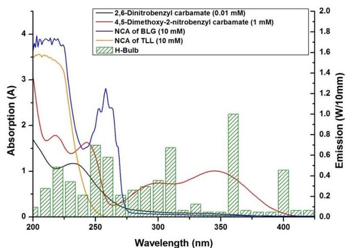
Figure S2: Absorption spectra of photoamine generators and NCA monomers in comparison with emission spectrum of the light source. All compounds were dissolved in acetonitrile.
