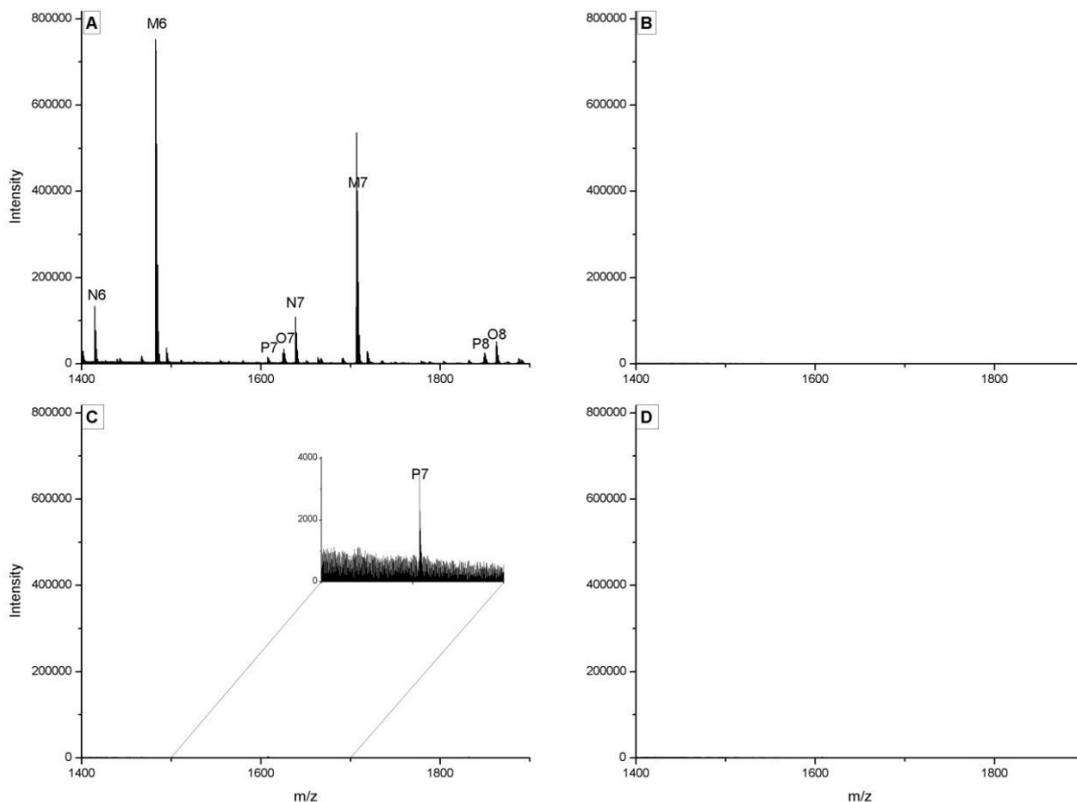
Figure S5: MALDI-ToF-MS spectra of photo-induced polymerization of TLL-NCA by 2,6-Dinitrobenzyl cyclohexylcarbamate **1**. A: +UV+1; B: -UV+1; C: +UV-1; D: -UV-1.
