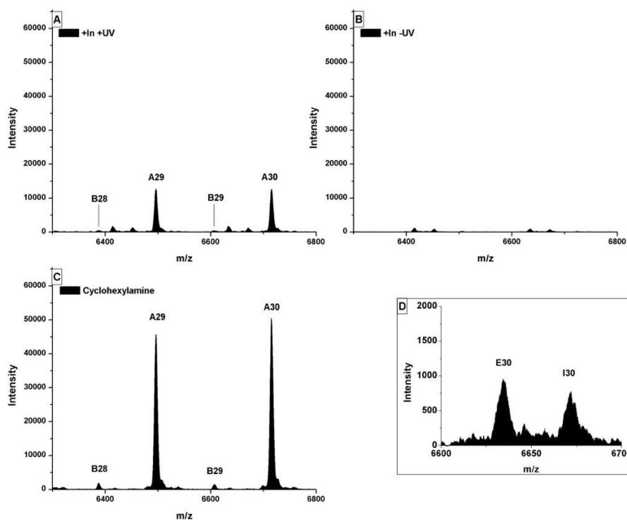
Figure S6: MALDI-ToF-MS spectra of photo-initiated polymerization of BLG-NCA by 4,5-dimethoxy-2-nitrobenzylcyclohexylcarbamate **2**. A: +UV+1; B: -UV+1; C: conventional cyclohexylamine initiated ROP; D: Zoom in of B.
