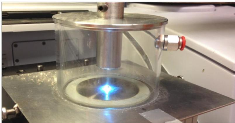
Figure S20: Set up of the Real-time infrared spectrometer. In 1 cm distance above the ATR-crystal the lamp was positioned.
