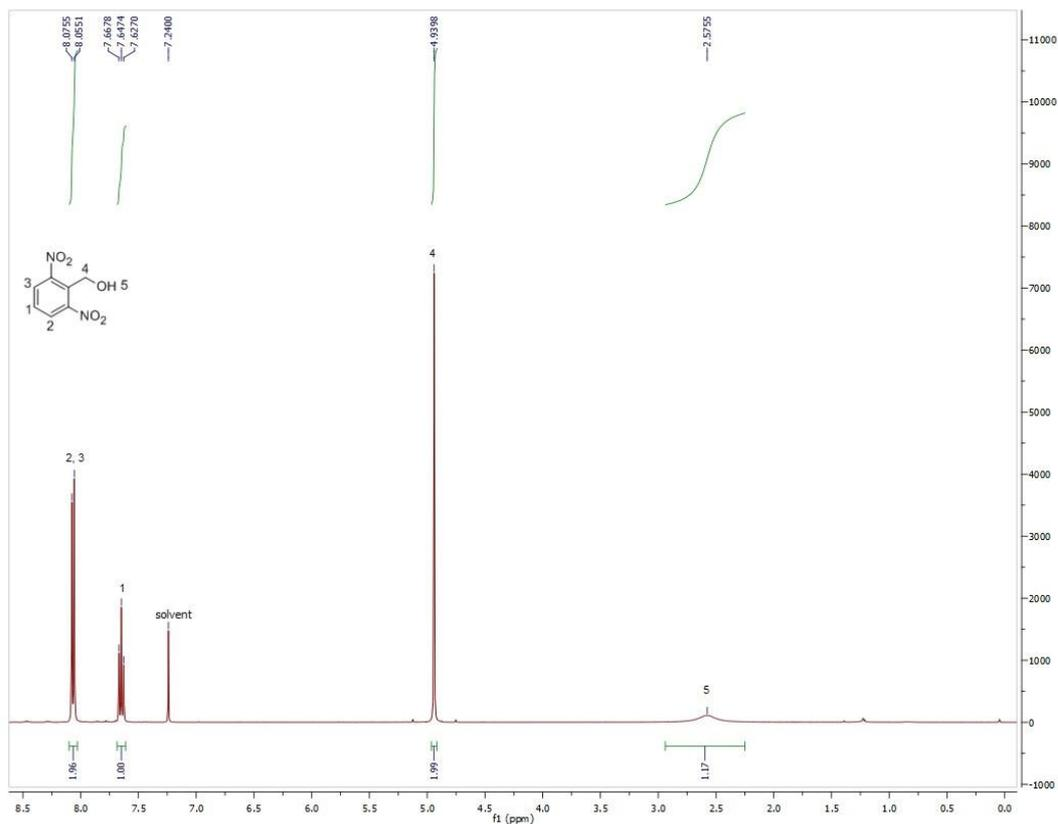
Figure S14: <sup>1</sup>H-NMR spectrum of 2,6-dinitrobenzenemethanol in CDCl<sub>3</sub>.
