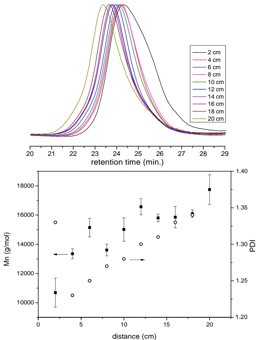
Figure S9: GPC traces of samples obtained at constant irradiation time and different light source to reactor distance using photoinitiator 2 and plot of average  $M_n$  and PDI of triplicate samples. Error bars represent standard deviation.
