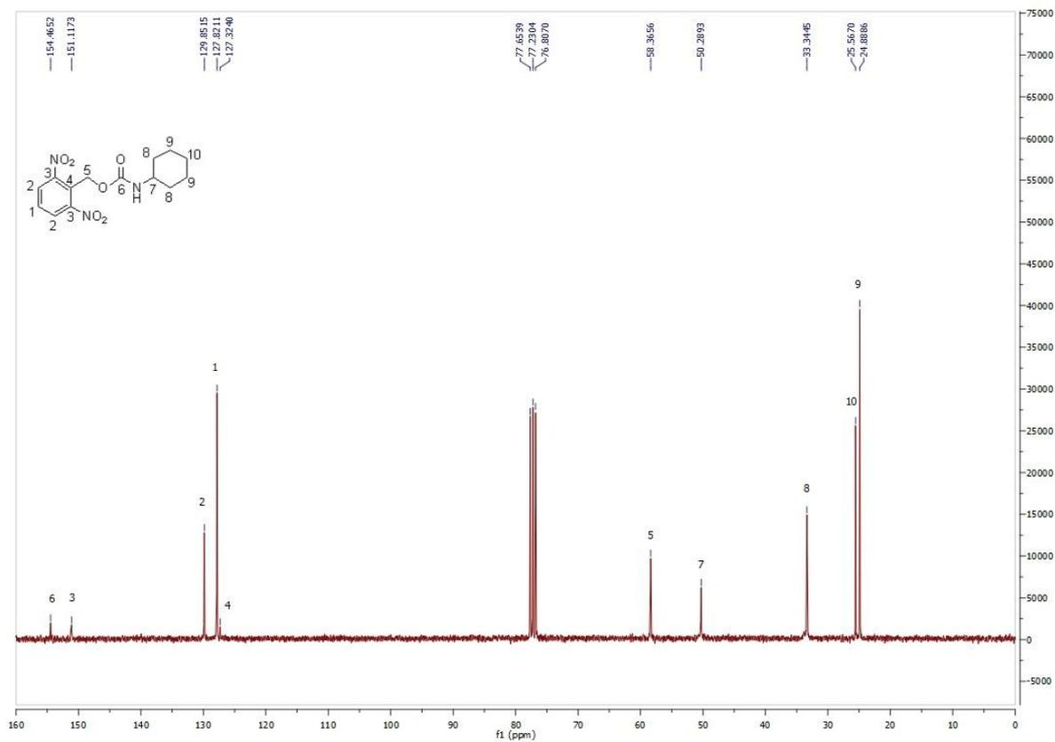
Figure 17: <sup>13</sup>C-NMR spectrum of 2,6-dinitrobenzylcyclohexylcarbamate in CDCl<sub>3</sub>.
