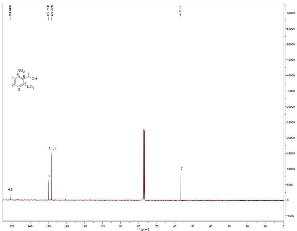
Figure S15: <sup>13</sup>C-NMR spectrum of 2,6-dinitrobenzenemethanol in CDCl<sub>3</sub>.
