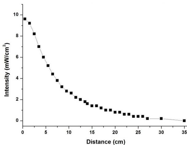
Figure S8: Dependence of light intensity of the Vilber-Lourmat L215-L UV lamp. The intensity was measured with Silverline Intensometer (real-time DMA setup)
