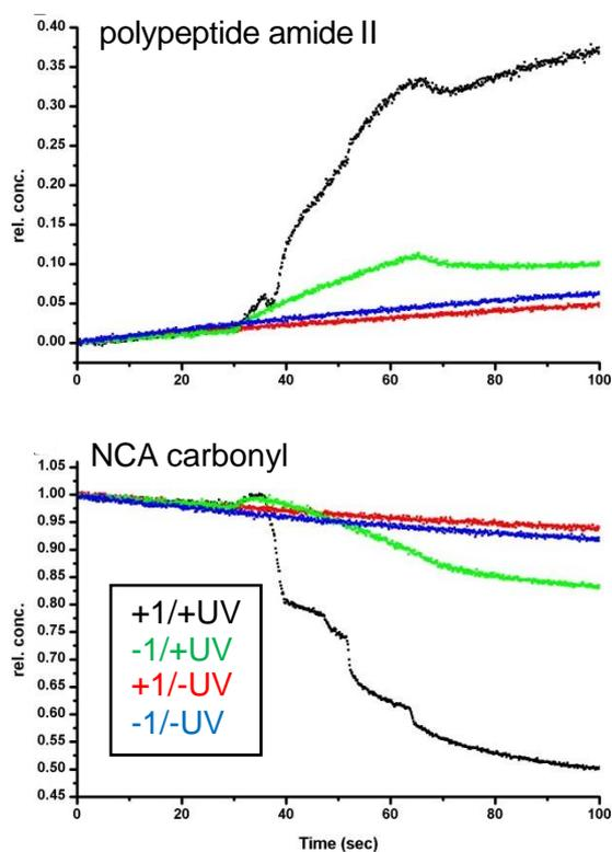
Figure S3: Real-time FTIR results of TFL NCA polymerization with and without **1** and UV light following the NCA carbonyl band at 1782  $\text{cm}^{-1}$  and the polypeptide amide II band at 1548  $\text{cm}^{-1}$ .
