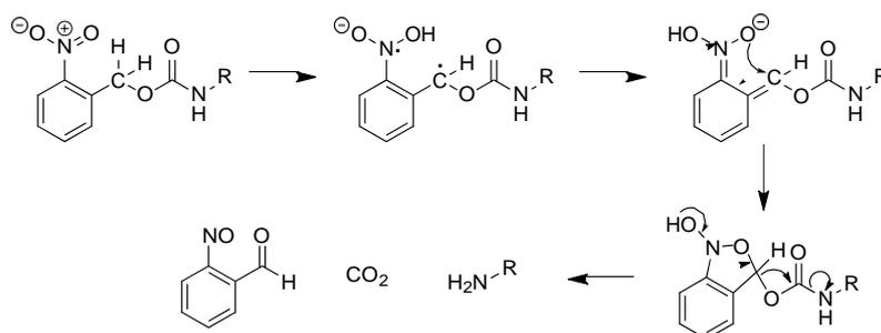
Figure S1: Photo-cleavage mechanism of the benzylcarbamate-based photoamine generators.
