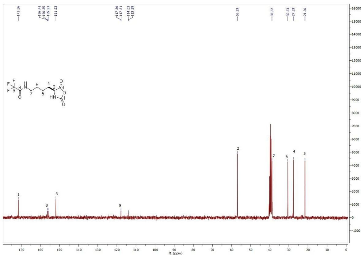
Figure S13:  $^{13}\text{C}$ -NMR spectrum of TLL-NCA in Dimethyl Sulfoxide- $d_6$
