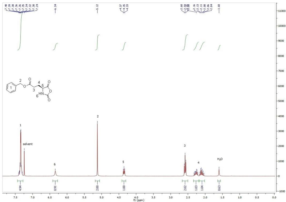
Figure S10:  $^1\text{H-NMR}$  spectrum of BLG-NCA in  $\text{CDCl}_3$
