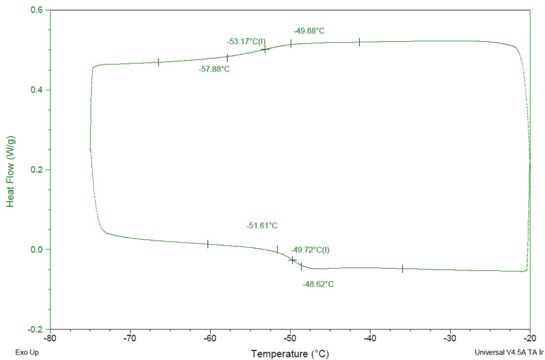
Figure S18. DSC trace for homopolymer showing glass transition at -49.72 °C (table 1, entry 6).
