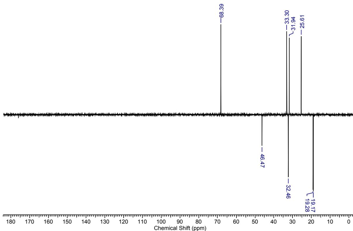
Figure S10. DEPT-135  $^{13}\text{C}\{^1\text{H}\}$  NMR spectrum for **4**.
