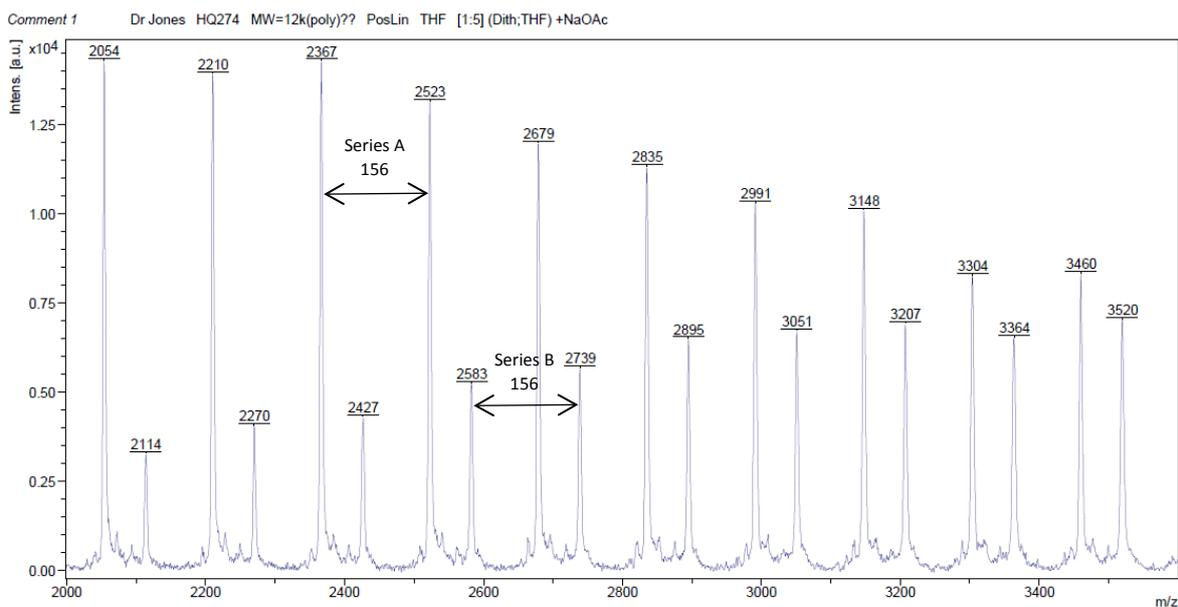
Figure S22. MALDI-TOF spectrum for Table 1, entry 6 showing polymer repeat units of  $156 \text{ g mol}^{-1}$ . Series A is cyclic polymer; series B is linear.
