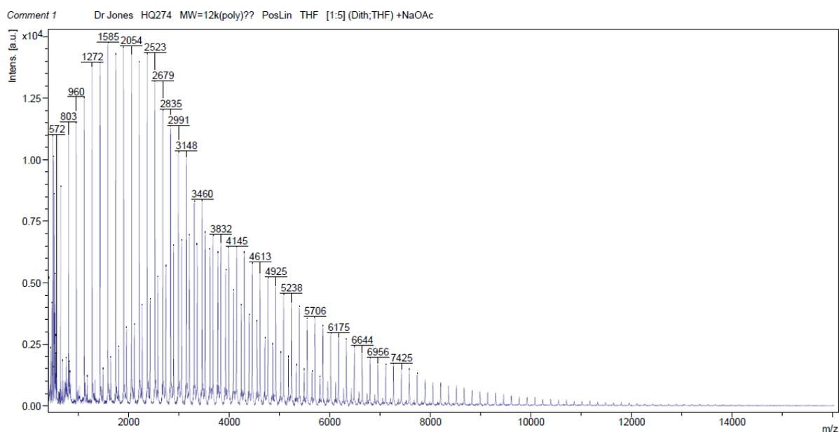
Figure S21. MALDI-TOF spectrum for Table 1, entry 6. Series A is cyclic polymer; series B is linear (HO<sup>i</sup>Pr capped).
