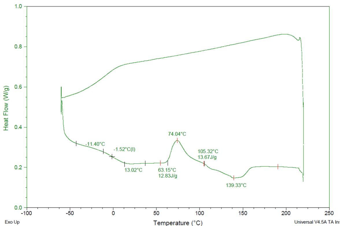
Figure S29. DSC trace for polymer sample (table 2, entry 13) showing  $T_g$ ,  $T_c$  and  $T_m$  thermal events.
