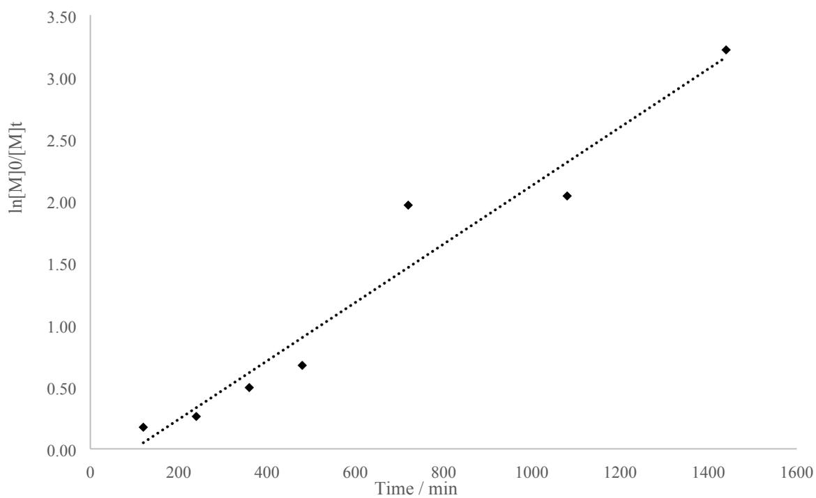
Figure S14. Kinetic plot for homopolymerisation of **4** with  $\text{Zr}(\text{tris})(\text{O}^i\text{Pr})$ ,  $[M]:[\text{Zr}] = 100:1$ , 100 °C, solvent free.
