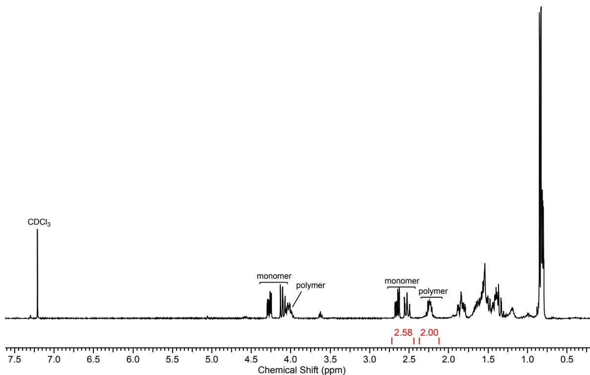
Figure S17. Example crude NMR spectrum showing conversion (table 1, entry 2).
