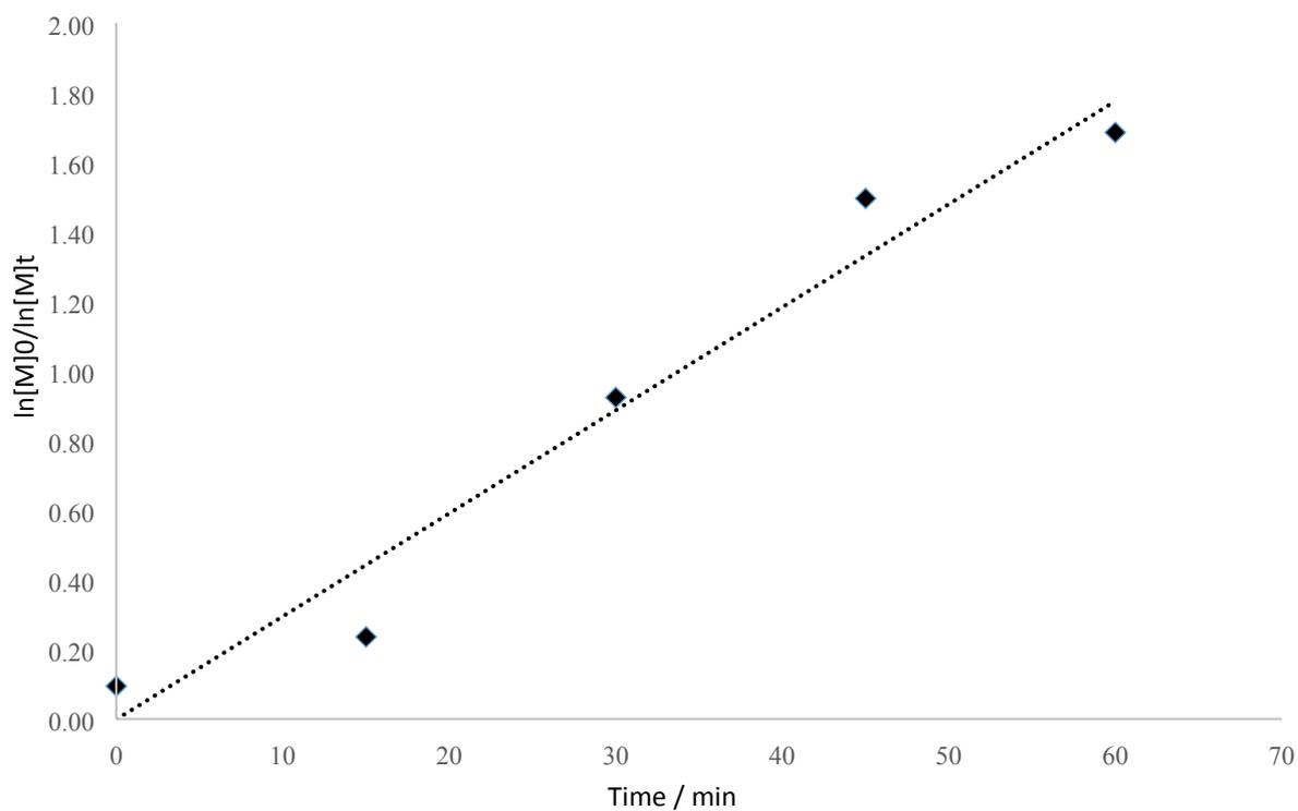
Figure S16. Kinetic plot for solution kinetics of homopolymerisation of **4** with  $Zr(bis)(O^iPr)_2$ ,  $[M]:[Zr] = 100$ ,  $d^8$  toluene,  $60\text{ }^\circ\text{C}$ .
