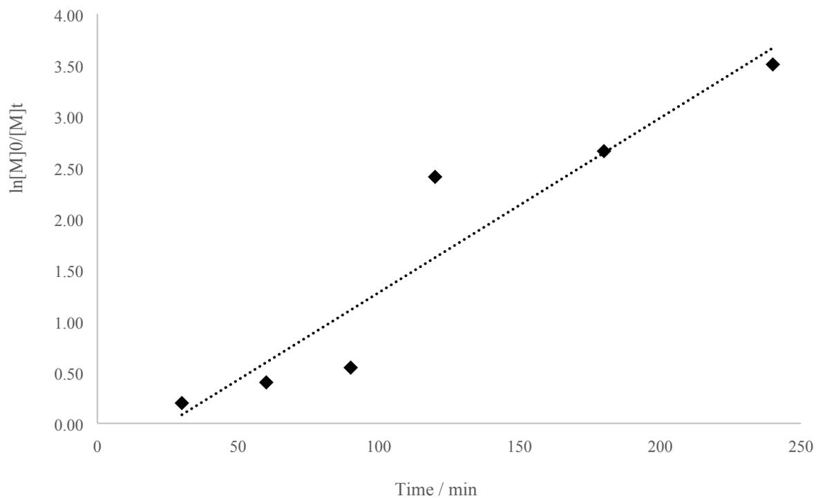
Figure S13. Kinetic plot for homopolymerisation with  $\text{ZnEt}_2/\text{BnOH}$ .  $[M]:[\text{Zn}]:[\text{BnOH}] = 100:1:1$ , 100 °C, solvent free.
