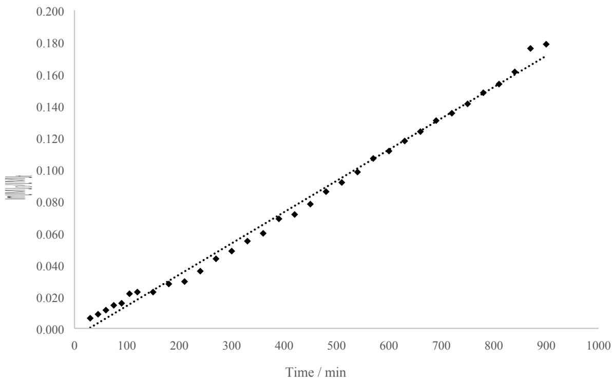
Figure S15. Kinetic plot for solution kinetics for homopolymerisation of **4** with  $Zr(tris)(O^iPr)$ ,  $[M]:[Zr] = 100:1$ ,  $d^8$  toluene,  $80\text{ }^\circ\text{C}$ .
