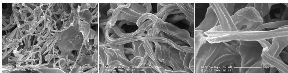
Figure S4. Scanning electron microscopy of the PSMA-hex-NH 2 fibers obtained from wet electrospinning.
