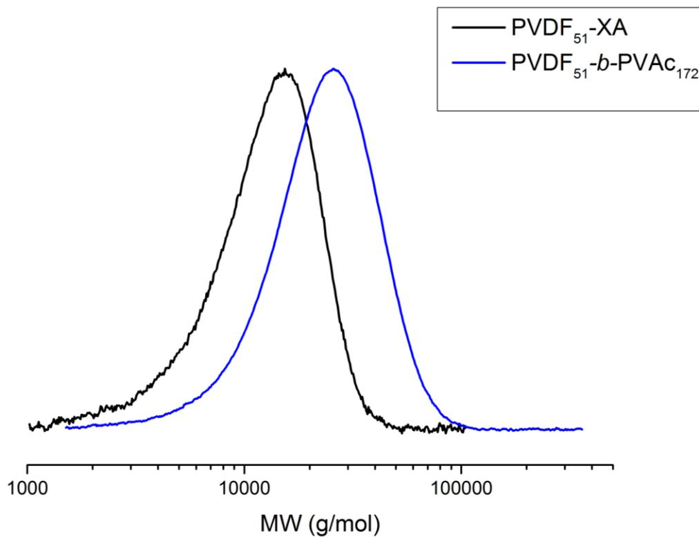
**Figure S6.** SEC chromatogram of PVDF<sub>51</sub> and PVDF<sub>51</sub>-*b*-PVAc<sub>172</sub> block copolymer before hydrolysis.
