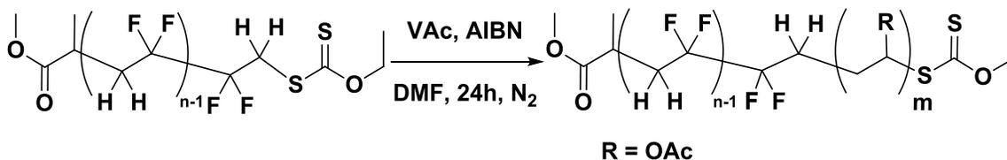
**Scheme 1.** Schematic synthetic procedure for the PVDF-*b*-PVAc block copolymer.
