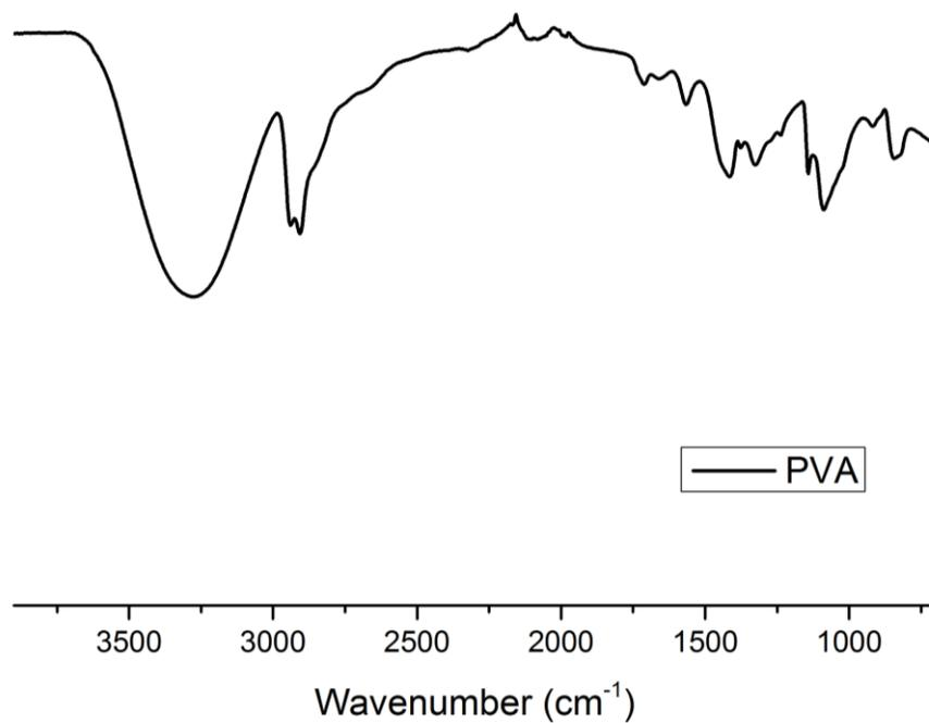
**Figure S7.** FTIR spectrum of commercial poly(vinyl alcohol) (>99 % of acetate hydrolysis).
