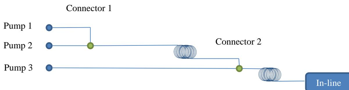
**Scheme S1.** Scheme of flow set-up
