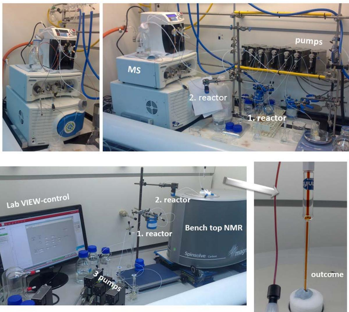
**Figure S1:** Top: flow set-up for the experiments in flow with the ESI-MS. Bottom: flow set-up for the flow NMR
