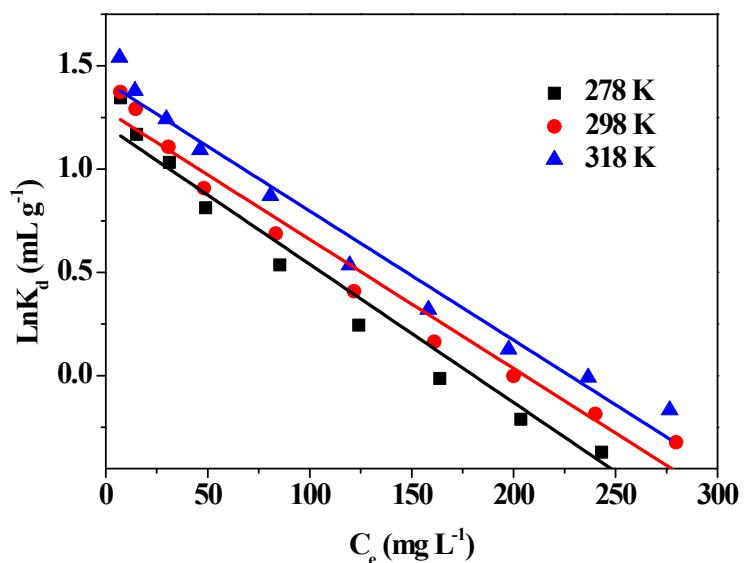
**Fig. S5** The linear plots of  $\ln K_d$  vs.  $C_e$  for U(VI) removal on N-doped Fe/Fe<sub>3</sub>C@C-800 at three different temperatures, m/V = 0.1 g L<sup>-1</sup>, pH = 6.0, and I = 0.1 mM Na<sub>2</sub>CO<sub>3</sub>.
