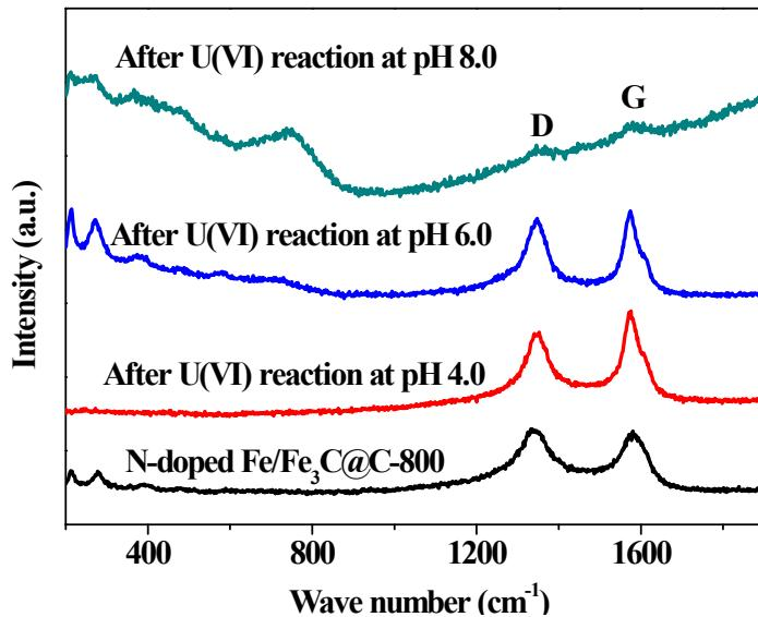
**Fig. S6** Raman spectra of N-doped Fe/Fe<sub>3</sub>C@C-800 before and after U(VI) reaction at pH = 4.0, 6.0, and 8.0.
