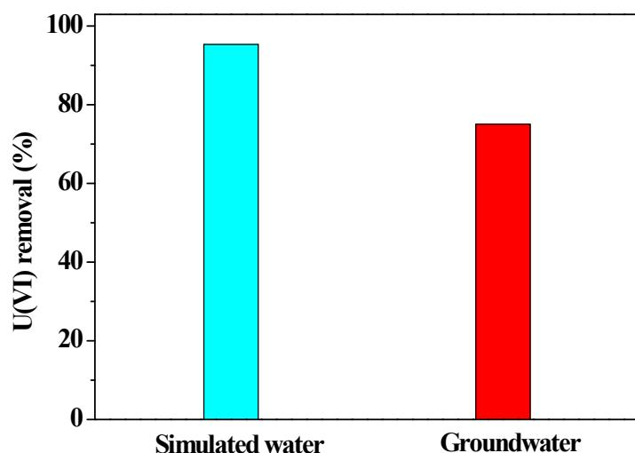
**Fig. S4** The removal efficiency of U(VI) by N-doped Fe/Fe<sub>3</sub>C@C-800 in simulated water (m/V = 0.1 g L<sup>-1</sup>, pH = 6.0, I = 0.1 mM Na<sub>2</sub>CO<sub>3</sub>, T = 25 °C) and contaminated groundwater (m/V = 0.1 g L<sup>-1</sup>, pH = 6.8, T = 25 °C).
