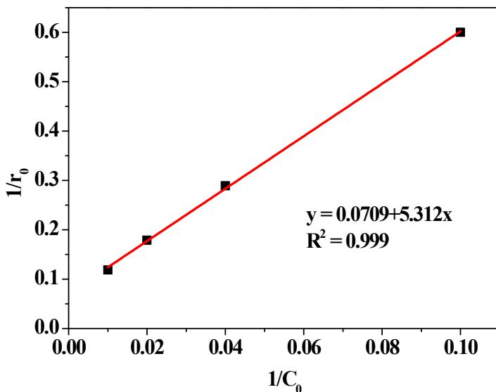
**Fig. S3** Linear fit of using a Langmuir-Hinshelwood kinetic model at different initial U(VI) concentrations. All batch experiments were conducted in  $m/V = 0.1 \text{ g L}^{-1}$ , pH = 6.0, 0.1 mM  $\text{Na}_2\text{CO}_3$ , and  $T = 298 \text{ K}$ .
