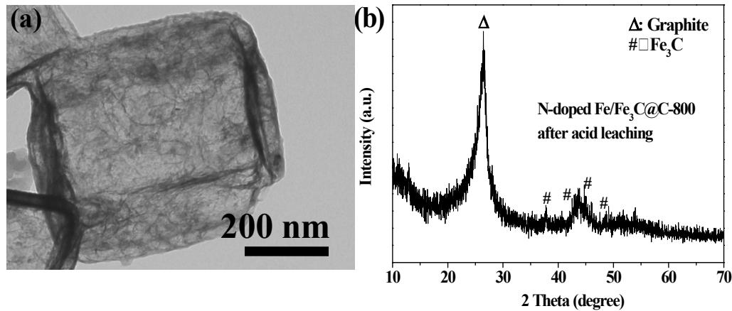
**Fig. S1** TEM image and XRD pattern of N-doped Fe/Fe<sub>3</sub>C@C sample after acid leaching.
