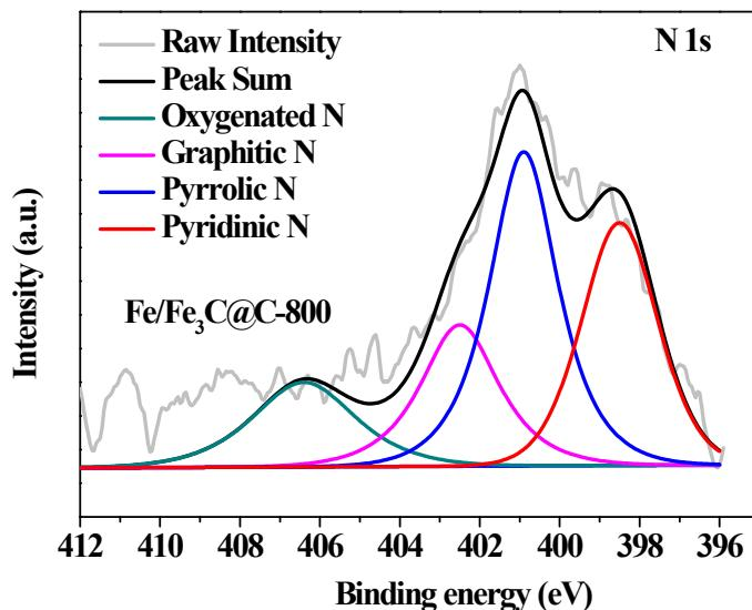
**Fig. S8** High resolution N 1s XPS spectrum of N-doped Fe/Fe<sub>3</sub>C@C-800.
