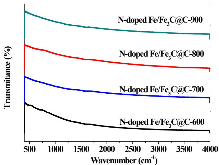
**Fig. S2** FTIR spectra of N-doped Fe/Fe<sub>3</sub>C@C products at different temperatures.
