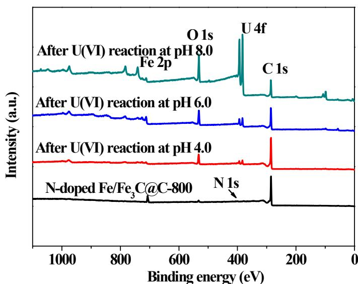
**Fig. S7** XPS survey of N-doped Fe/Fe<sub>3</sub>C@C-800 before and after U(VI) reaction at pH = 4.0, 6.0, and 8.0.
