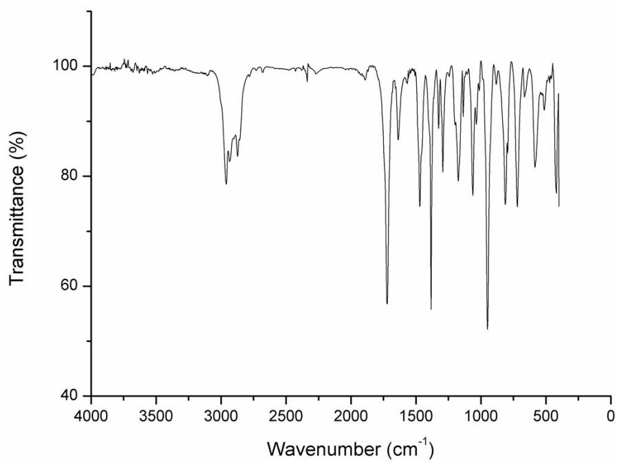
**Figure S1.** FT-IR spectroscopy studies of compound **2**.
