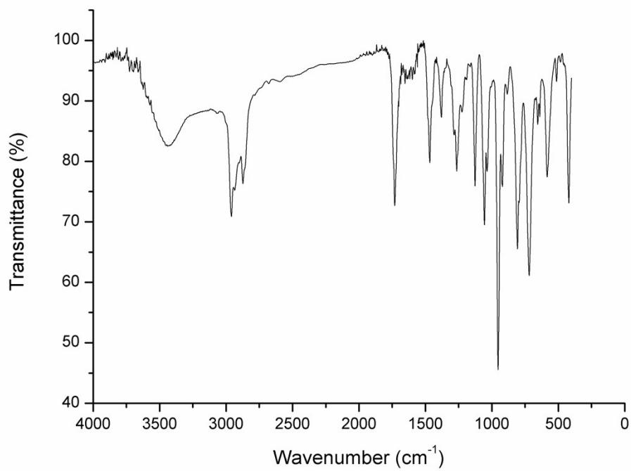
**Figure S2 .**FT-IR spectroscopy studies of compound **3**.
