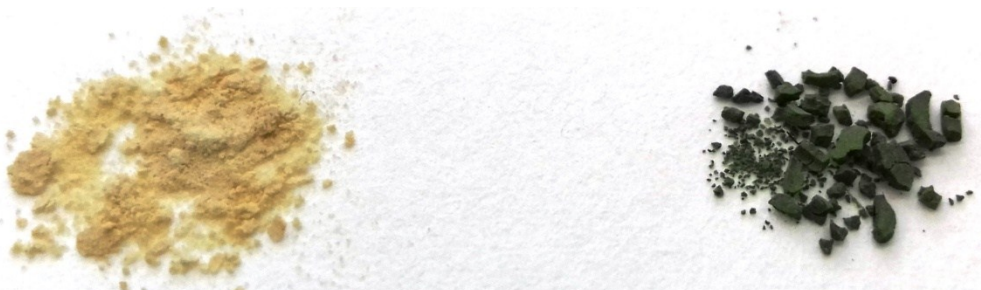
Fig. S6. Photos of polycrystalline powder samples of AEMOF-7 (left) and AEMOF-7-Cu (right).
