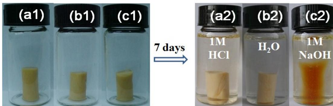
**Figure S7.** Stability of the hydrogel-5. Digital photographs of hydrogel-5 before and after swelling in acidic and alkaline conditions.
