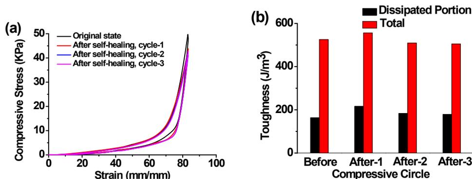
**Figure S5.** Self-healing property. (a) Cycle compression tests of hydrogel-5 of compression to 80 % strain before self-healing and undergoing 3 cycles after healed for 24 h. (b) the calculated total toughness and the dissipated toughness of hydrogel-5 before self-healing and after self-healing based on (a).
