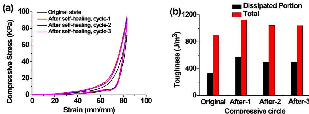
**Figure S6.** Self-healing property. (a) Cycle compression tests of hydrogel-4 of compression to 80%
