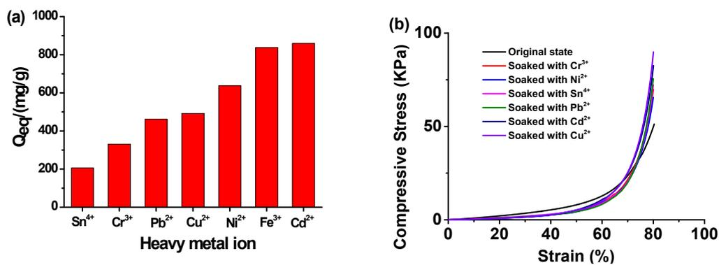
**Figure S8.** (a) Saturated adsorption capacities of hydrogel-5 for seven metal ions, (b) the compression tests of hydrogel-5 soaked in different metal ions' solution (c=0.001 mol/L).
