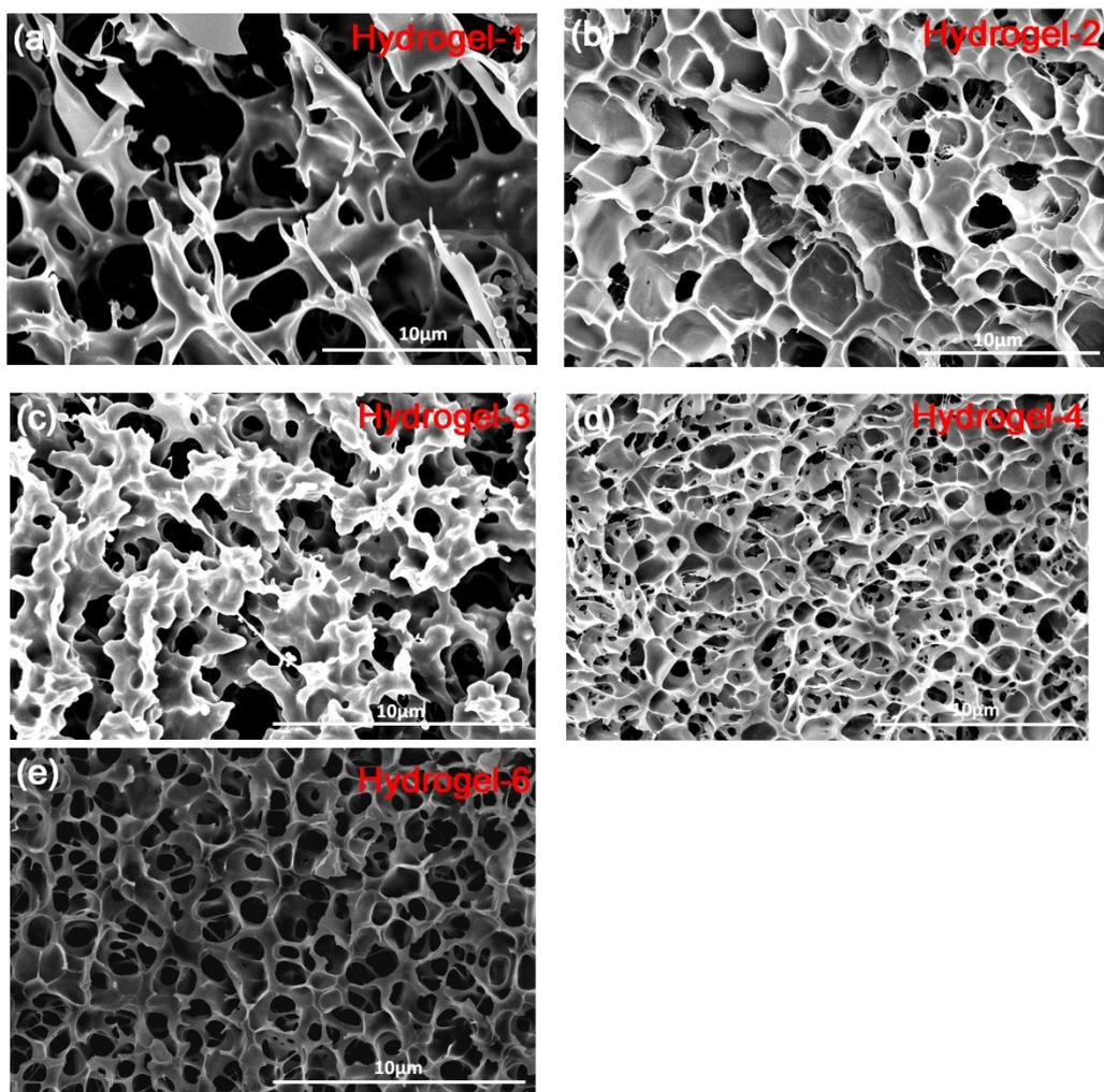
**Figure S1.** The cross-section surface morphology of the obtained hydrogels. Representative SEM images of cross-section surface morphology of (a) hydrogel-1, (b) hydrogel-2, (c) hydrogel-3, (d) hydrogel-4, (e) hydrogel-6.
