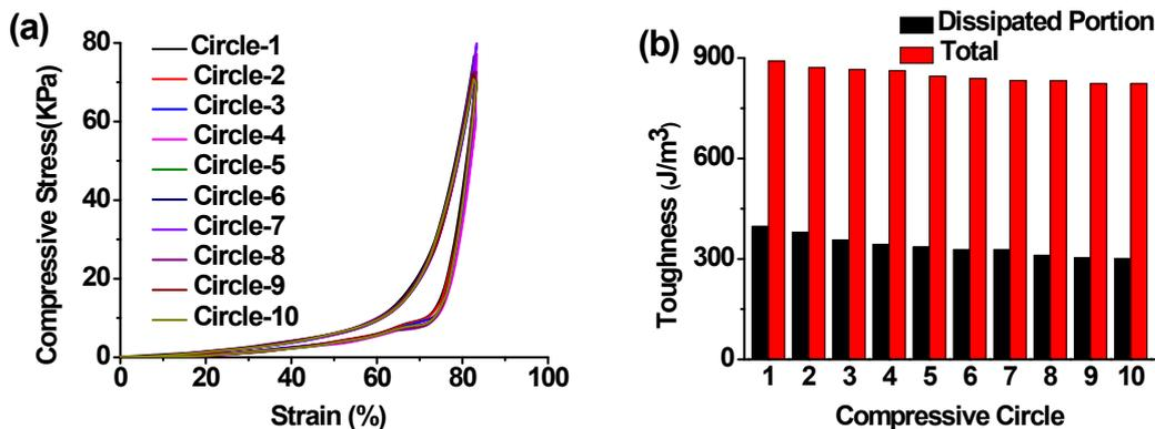
**Figure S4.** Fatigue resistance of hydrogel-4. Cycle compression test of hydrogel-4 undergoing 10 cycles of compression to 80% strain (a); (b) the calculated total toughness and the dissipated toughness of hydrogel-4 during loading-unloading tests based on (a).
