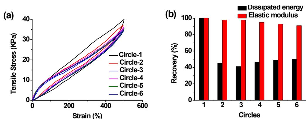
**Figure S3.** Loading-unloading cycling tests of hydrogel-4. (a) Six successive loading-unloading cycles of the hydrogel-4; (b) the recovery of elastic modulus and hysteresis loop area calculated from (a).
